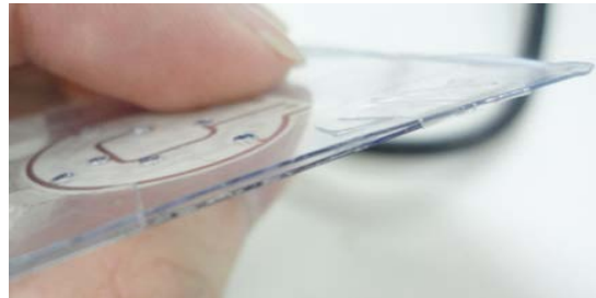
Figure 16. Flexible opto-electronic patch sensor (OEPS).
