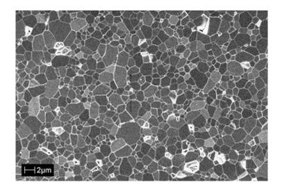
Fig. 1. SEM micrograph of the alumina microstructure after 1  $\mu$ m polishing and thermal
