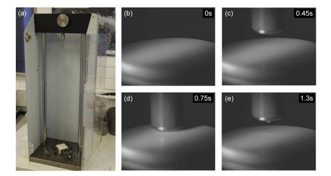
Fig. 2. The DW test apparatus; (a) a photograph of the DW test rig, (b-e) frames taken from high-speed camera footage of the DW impact process; (b) shows the sample prior to damage;
