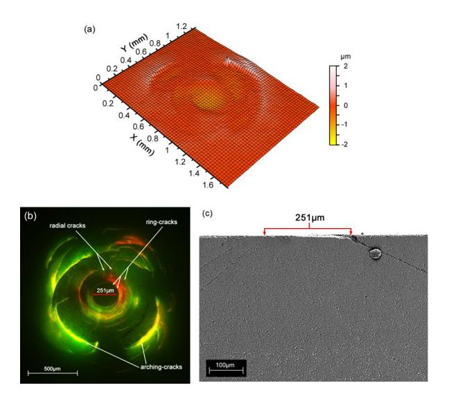
Fig. 3. Optical and SEM imaging of the deformation and damage produced during a 0.6kg DW impact test on alumina: (a) 3D optical microscopy map of the residual impression, (b) UV optical microscopy of the resultant fracture patterns, (c) SEM image of the crosssectioned DW impression.
