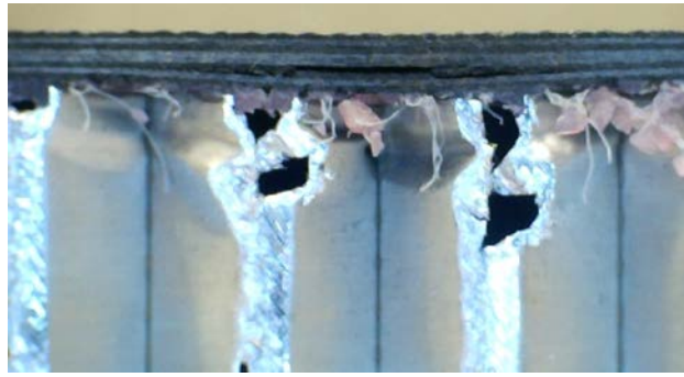
Fig. 9. A thin sandwich panel with cross ply skins under rigid support with 20 mm diameter indenter
