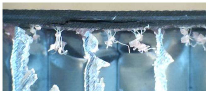
Fig. 11. A thin sandwich panel with quasi-isotropic skins under rigid support with 20 mm diameter indenter
