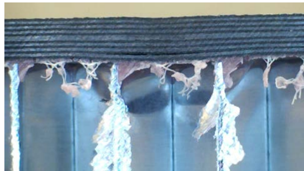
Fig. 10. A thick sandwich panel with cross ply skins under rigid support with 8 mm diameter indenter
