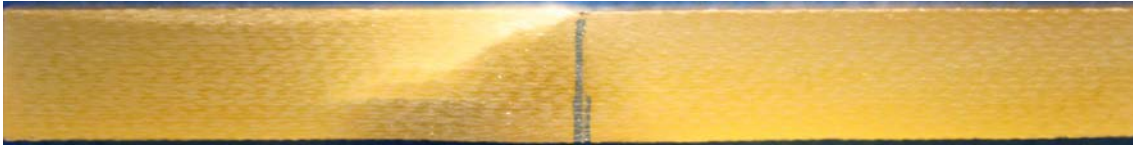
Figure 5: A failed SBS quasi-isotropic E-glass/epoxy specimen
