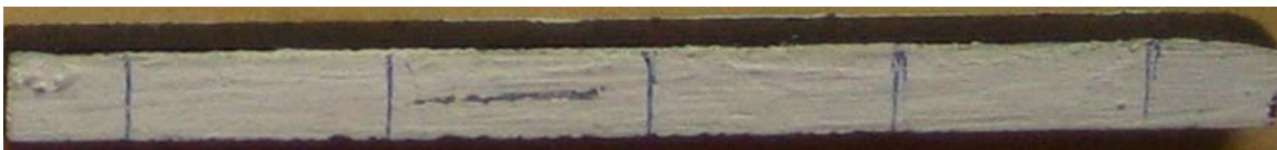
Figure 4: A failed DBS quasi-isotropic carbon/epoxy specimen
