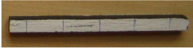
Figure 4. Failed DBS carbon/epoxy specimen
