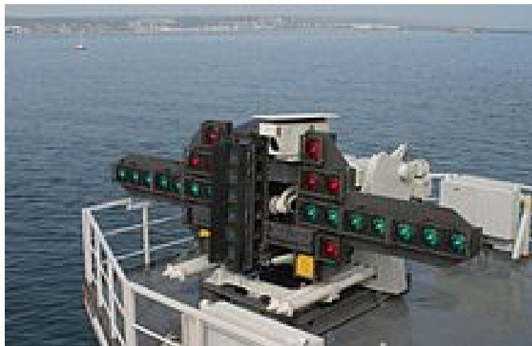
Figure 6. A Deck Approach Light Projector mounted on a naval vessel.
