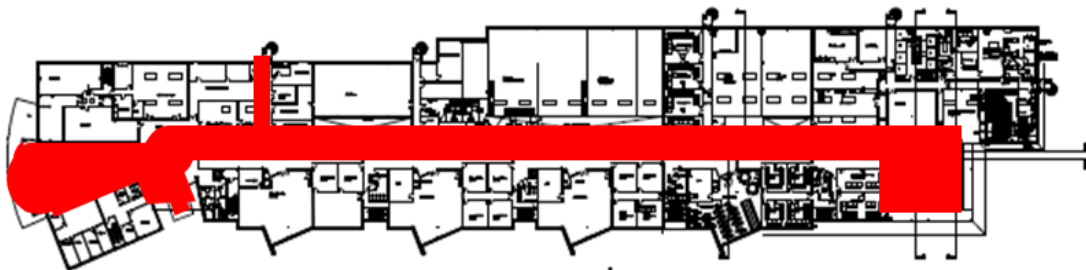
Figure 4. Plan View Schematic of the College Building; Red Areas Denoting Locations Simulated within IES
