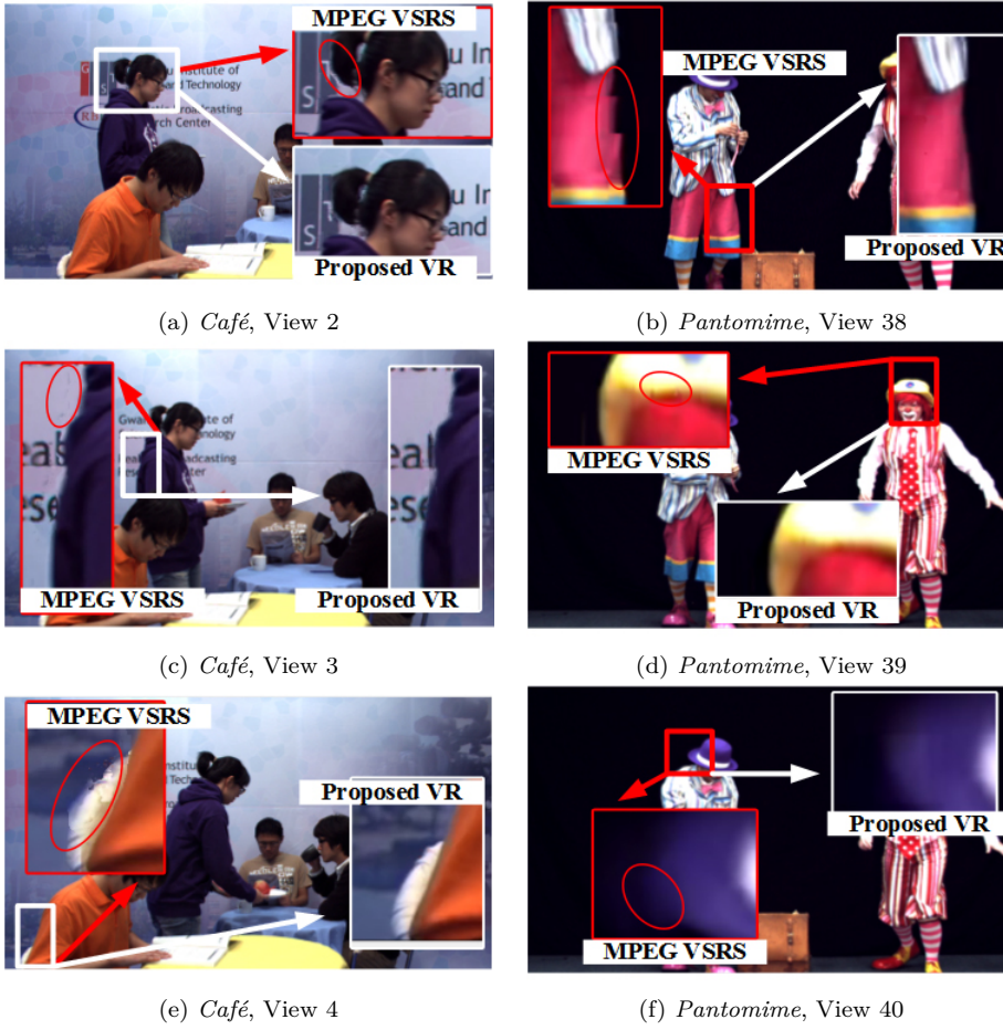
Fig. 13: Visual view reconstruction performance comparison between the MPEG-VSRS and the proposed view reconstruction ( proposed VR ) method. The resulting reconstruction views are shown for two different MVV contents: Café (left) and Pantomime (right). Three successive views for each content are shown and the most representative distortion areas are marked with red.
