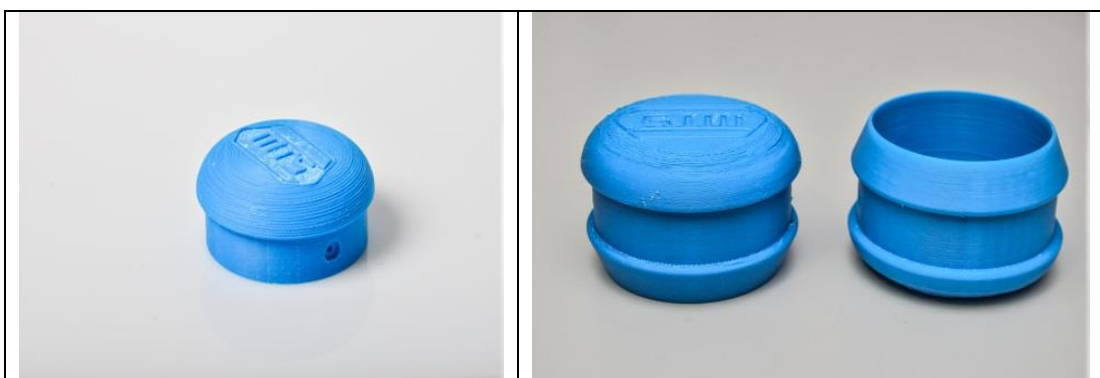
Fig 3: Partially printed bottom part
