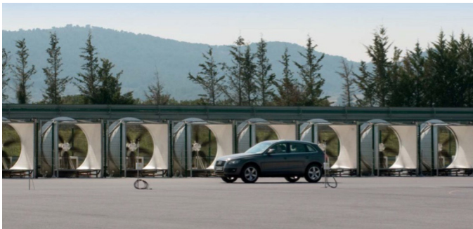
Figure 1. Crosswind Generator Facility at Applus+ IDIADA Proving Ground, Spain [12].
