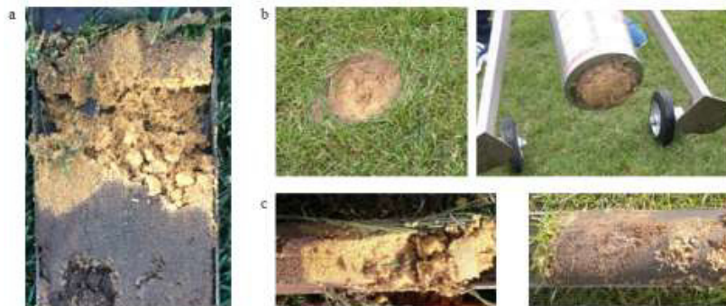
Figure 1. (a) Soil Profile with Distinct Soil Variation (b) Rotational Traction device (RTD) irregular catastrophic failure of sand top-dressed natural pitch (c) Soil profiles: (left) Desso Grassmaster system with synthetic fibres through structure; (right) Sand top dressed natural soil pitch with agglomerated sand in its structure
