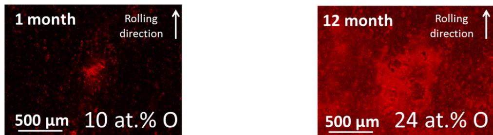
Figure 4-5: EDS maps showing the increase in O concentration with increasing atmospheric exposure time on Cu1.
