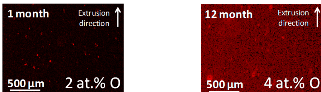
Figure 4-41: EDS maps showing the increase in O concentration with increasing atmospheric exposure time on SF2.
