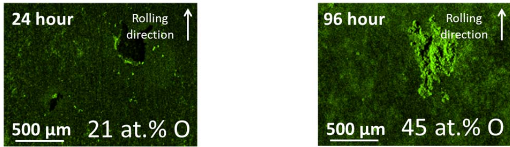
Figure 5-19: EDS maps showing the increase in O concentration with increasing immersion time on Cu3.
