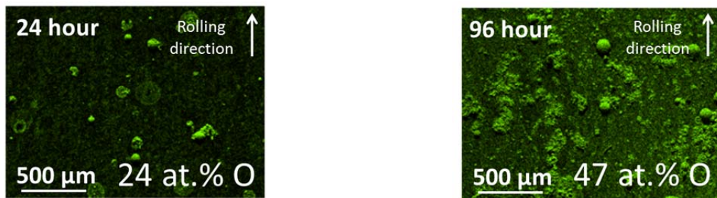
Figure 5-4: EDS maps showing the increase in O concentration with increasing immersion time on Cu1.
