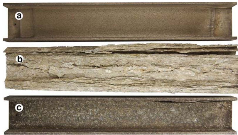
Figure 1-31: Different types of atmospheric corrosion on AA2024 which are dependant on location a) urban, b) coastal c) industrial [126].
