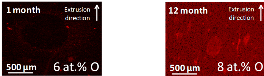
Figure 4-27: EDS maps showing the increase in O concentration with increasing atmospheric exposure time on Mg1.
