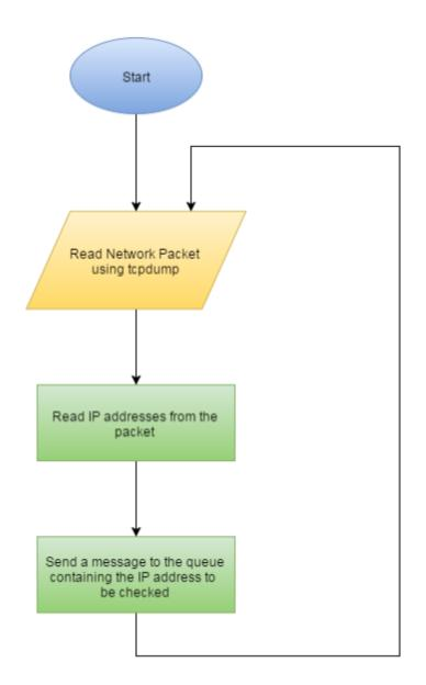
Figure 5.12: Network sniffing module when using message broker
