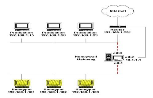
Figure 2.5: Honeywall architecture (Source: (Project, 2012))
