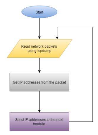
Figure 5.3: The flow chart of the network sniffing module
