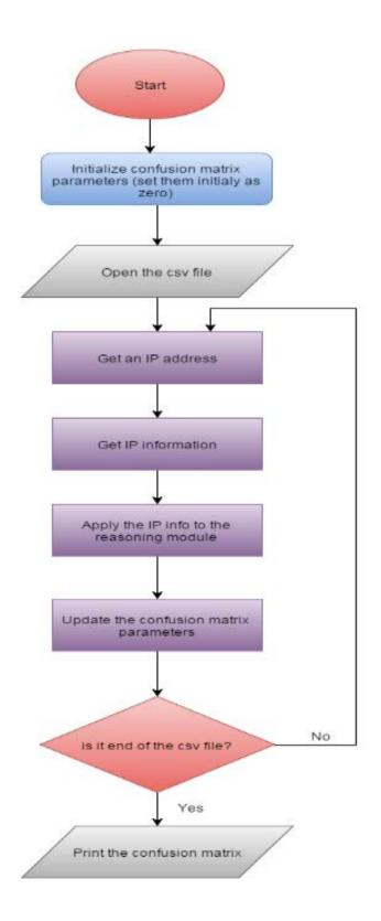
Figure 6.2: The flow chart of the testing proces
