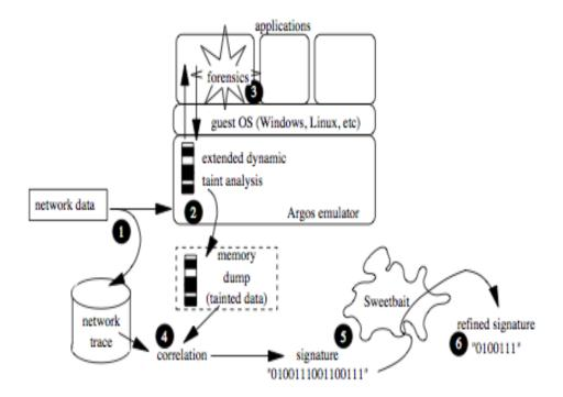
Figure 2.6: High-Level overview of Argos (Source: (Portokalidis et al., 2006))
