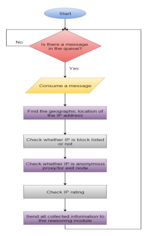
Figure 5.13: The flow chart of the IP information module when using
