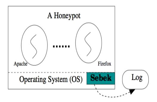
Figure 2.4: Sebek based approach in honeypot monitoring in context of HTTP (Source: (Jiang and Wang, 2007))
