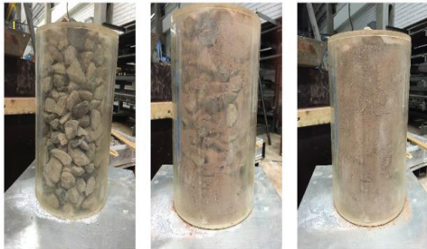
Figure 3 Representation of 3 fouling states using R_{FV} = 100\% , R_{FV} = 50\% and R_{FV} = 0\% :
