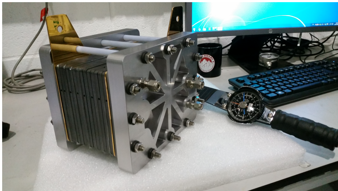
Figure 6.2: Pragma 7 cell, 470W research development stack
