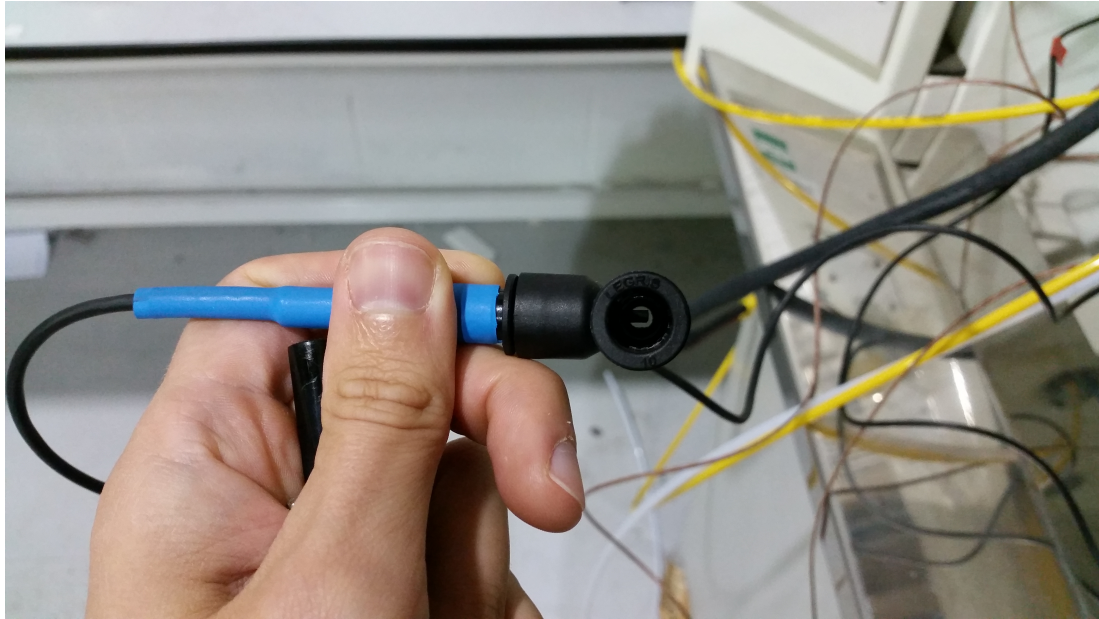
Figure 6.7: Humidity sensor T-piece detail
