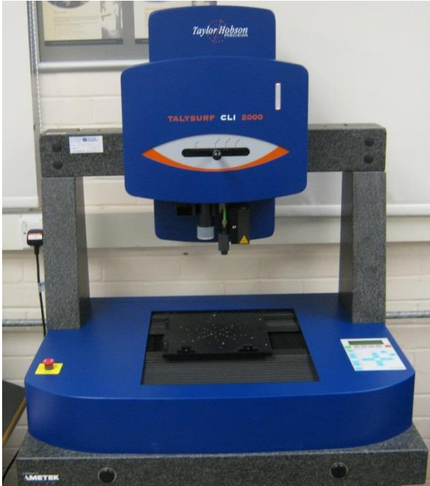
Figure 65 – The Talysurf™ CLI 2000 scanning topography measurement system at the Metrology Unit within the School of Mechanical and Manufacturing Engineering at Loughborough University. The particle coated slides were placed on the mobile stage under the gauge.
