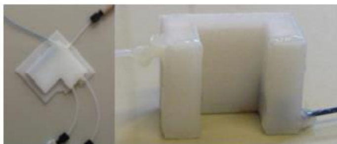
Figure 28: Examples of acetoxysilicone polymer microfluidic devices manufactured via FDM. 119
