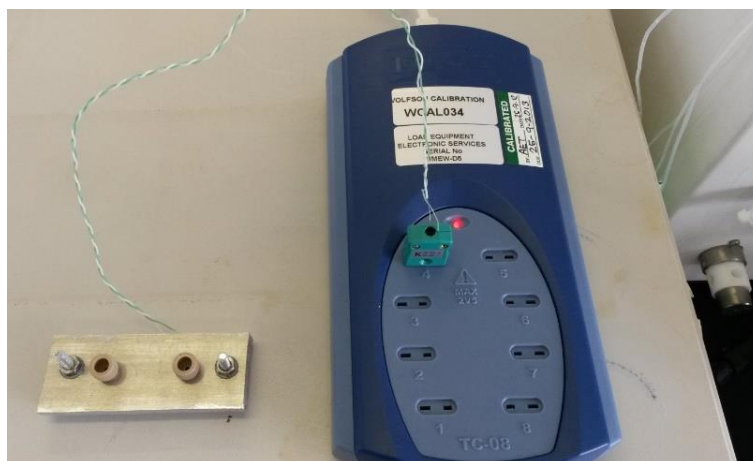
Figure 119: UAM Part 3 attached to a data logger.
