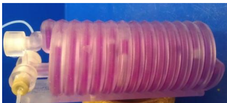
Figure 57: SL part 4 with a coloured solution being pumped through, confirming the sealing of the part.
