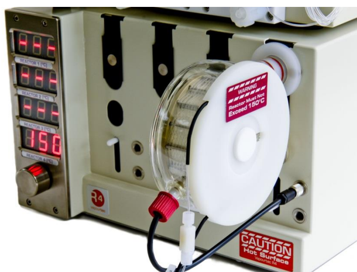
Figure 24: Example of a PFA mesofluidic reactor coil. 112
