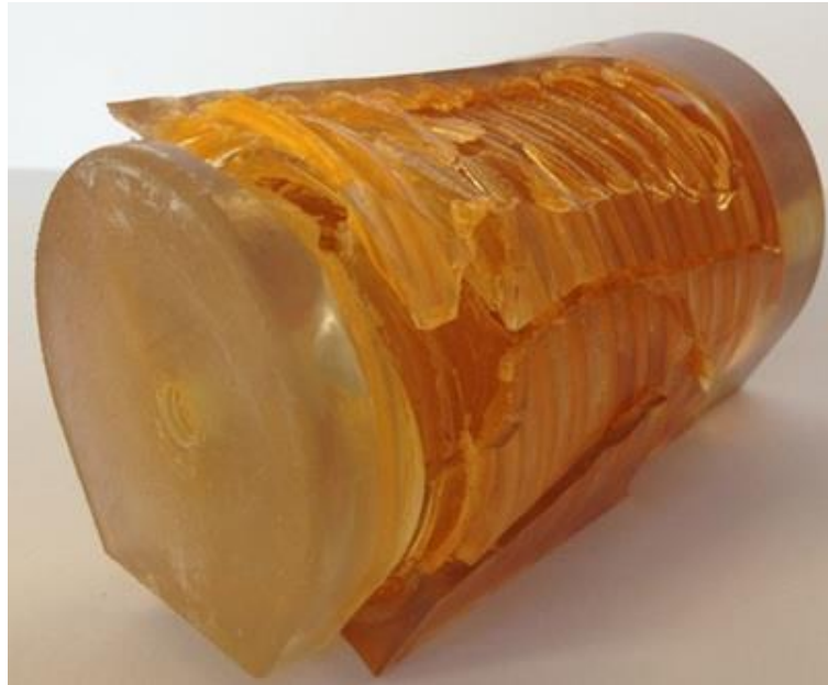
Figure 54: Destructive swelling of SL part 3
