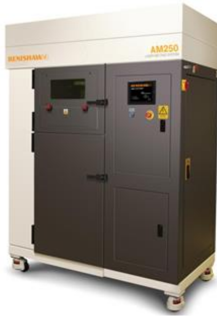
Figure 69: The Renishaw AM250 used during this research. 158
