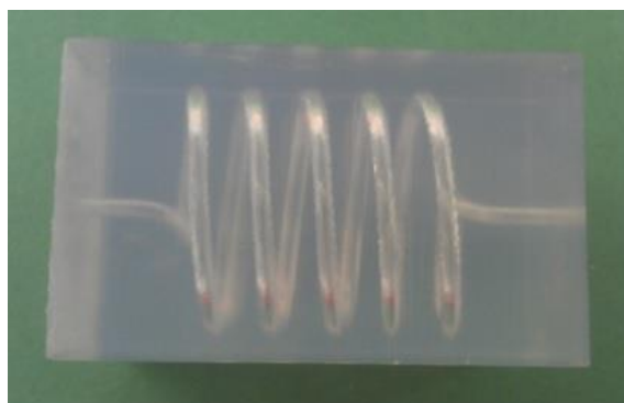
Figure 50: Photograph of SL Part 1 after cleaning.
