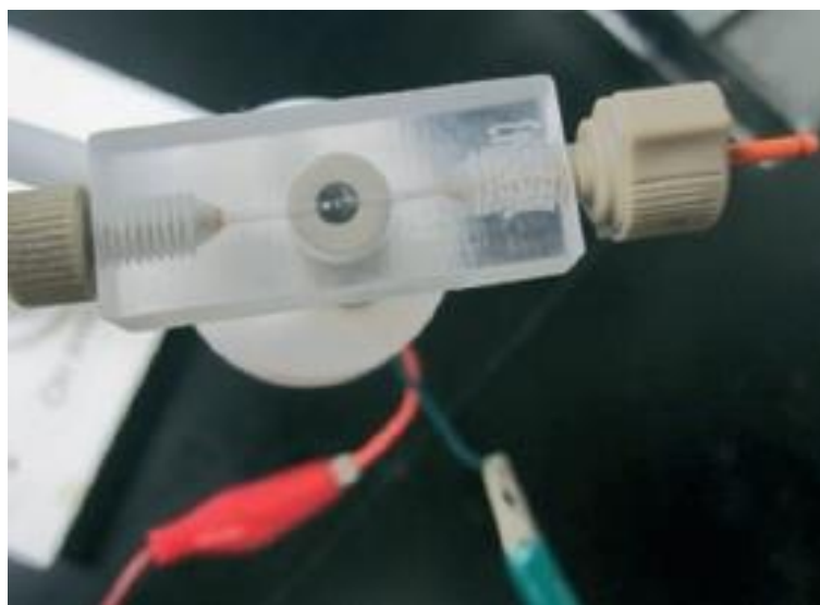
Figure 32: Electrochemical flow cell manufactured using an Objet Connex. 127
