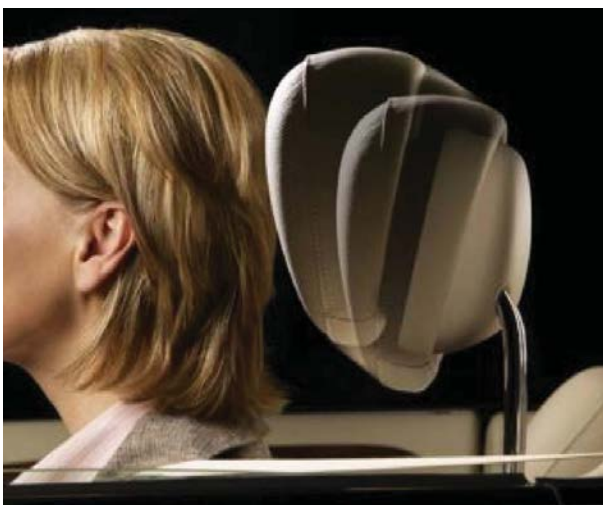
Figure 5. The movement of the NECK-PRO relative to the occupant's head [3].
