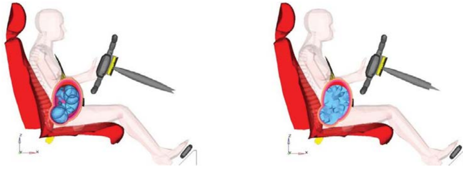
Figure 4. Computational pregnant occupant model ‘Expecting’ (with fetus) and modified ‘Expecting’ without a fetus.
