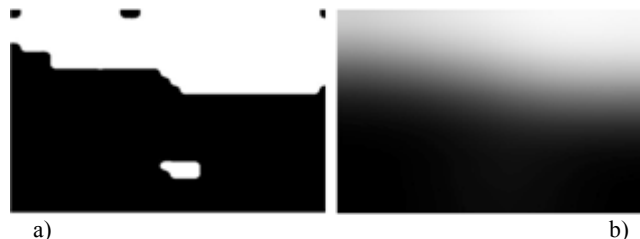
Figure 7: a) Fusion mask obtained from section 2.2.2. b) Fusion mask with blurred with a Gaussian kernel
