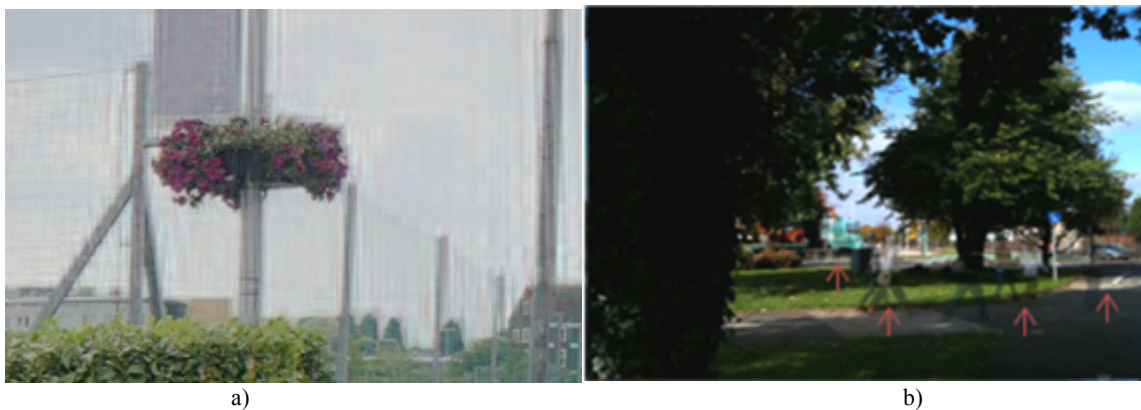
Figure 3: a) Fusion artefacts appeared in a fused image (150 % zoom) when using a WCBT fusion as in [16]. Visible artefacts: blockiness, lost of resolution, chromatic aberrations effect, and hazy appearance. b) Image with a ghosting effect (indicated by the arrows).
