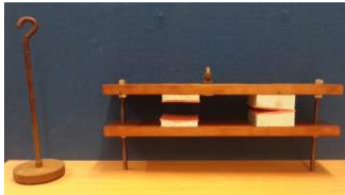
Figure 6.1 (a) An annotated diagram illustrating the frame design used to suspend varying weights from the Carter wind turbine blade. (b) Photograph of frame as-built and the hook.
