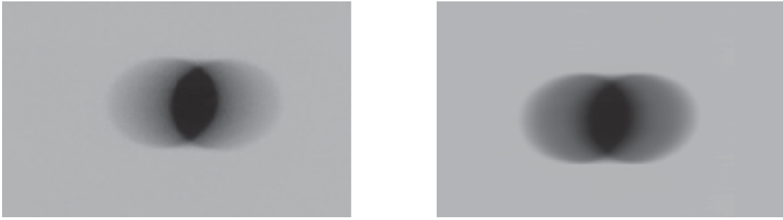
Figure 3.17: (a) As-taken and (b) simulated image of a motion blurred circular target
