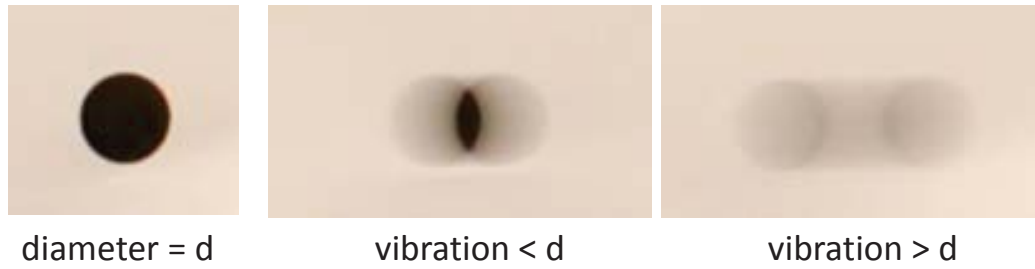
Figure 3.16: Motion blurred circular targets where motion is smaller and larger than target diameter. The motion-blurred images correspond with figure 2.11(b) and (d) by Kraus (1993).
