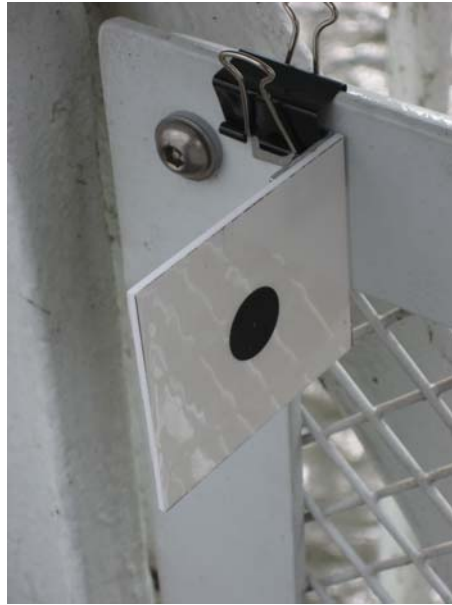
Figure 4.10: Targets used on the Wilford Bridge case study
