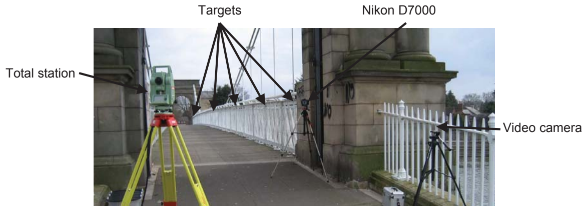
Figure 4.9: Arrangement of of sensors and target for Wilford Suspension Bridge case study
