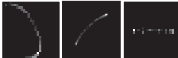
Figure 2.15: Samples of generated point spread functions describing linear and other non-linear motion. These figures were created using the procedure described by Fergus et al. (2006) from motion blurred images taken in the lab.
