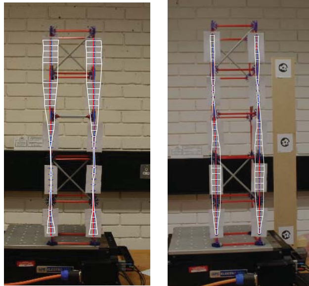
Figure 4.4: Test model with measured second (3.0 Hz) and third (8.1 Hz) vibration envelopes overlain
