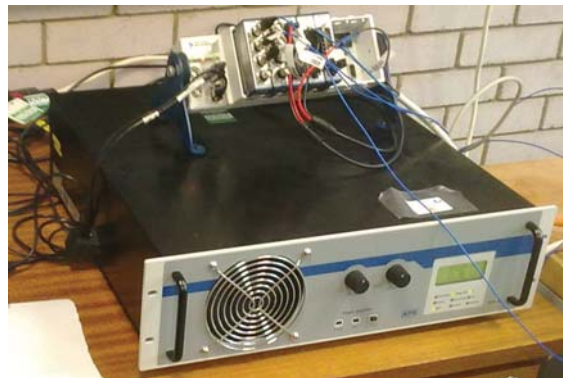
Figure 3.6: Shake table control system (NI CompactDAQ and APS 125 signal amplifier)
