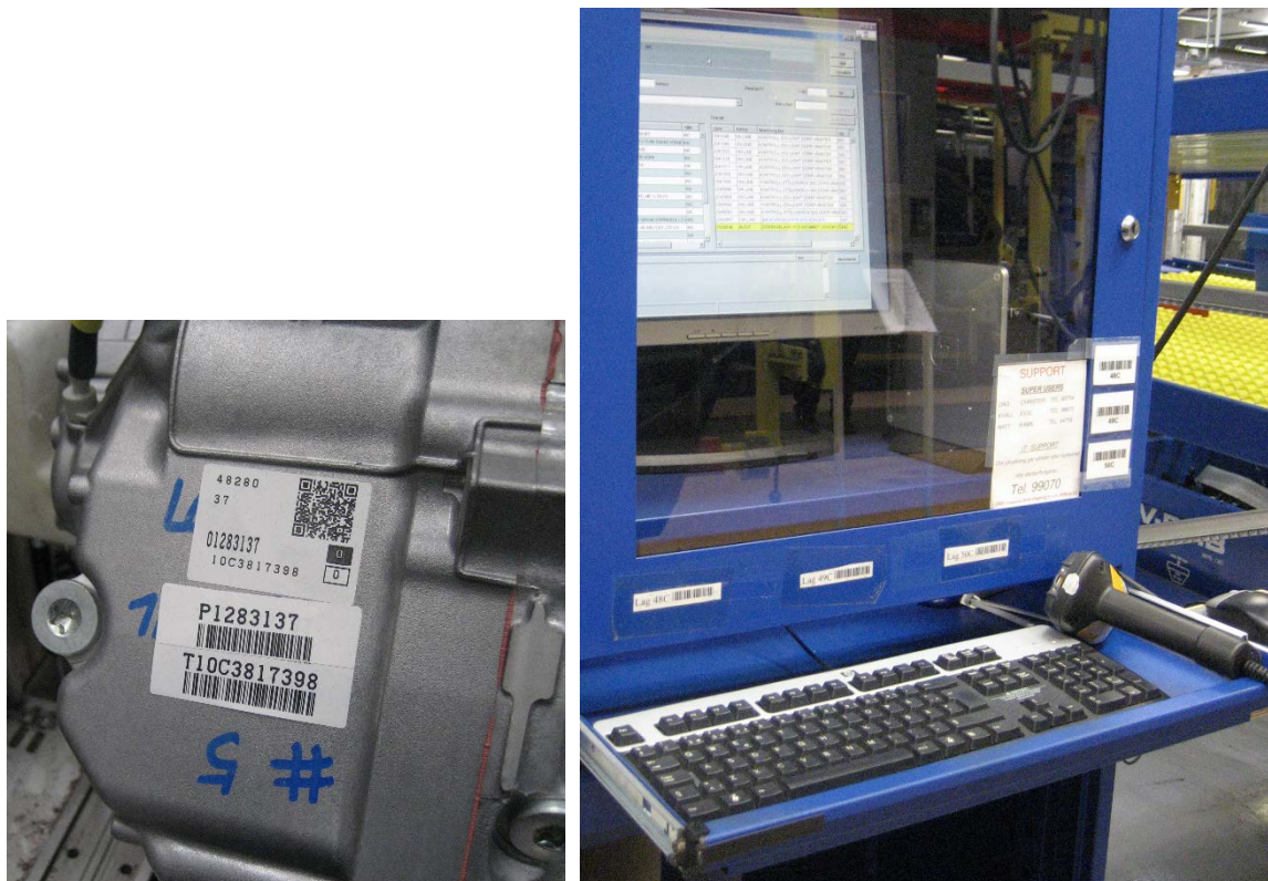
Figure 3.10. A component with attached scancode and an example of a scanning device connected to the workstation
