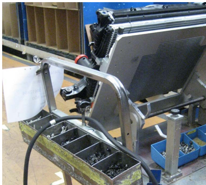
Figure 3.13. An example of fasteners provided by the assembly workstation
