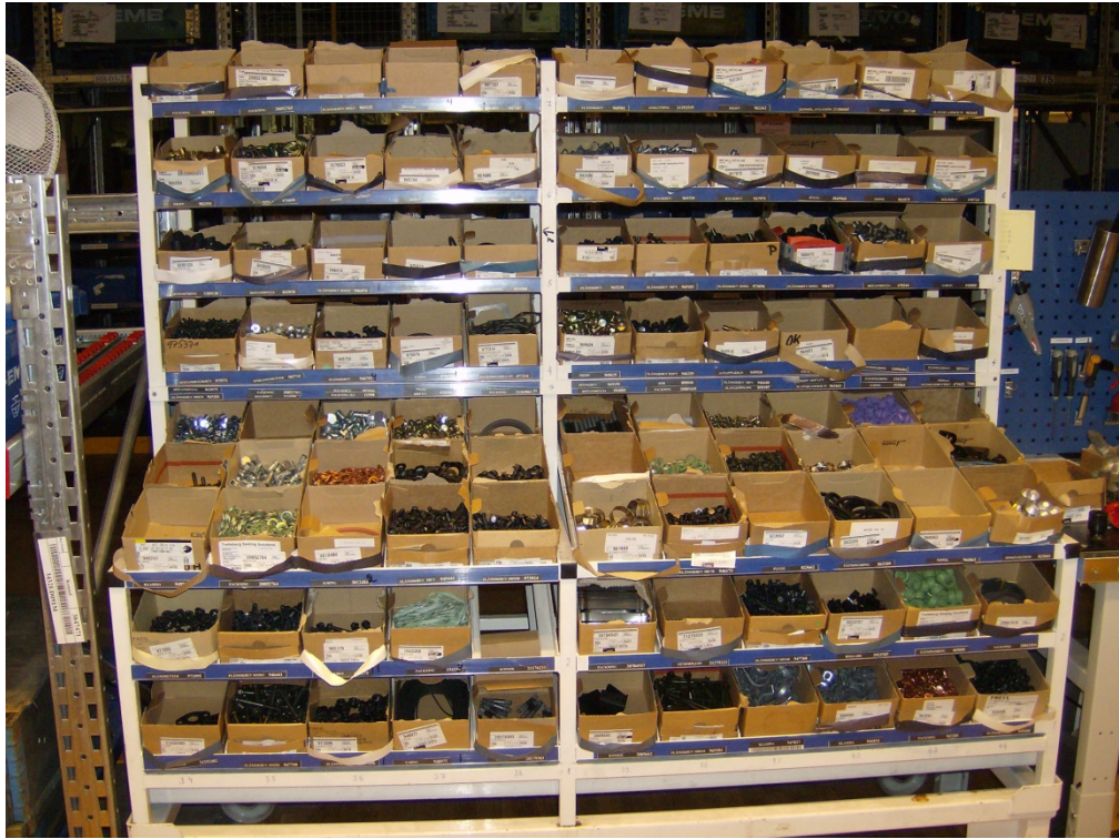
Figure 3.4. An example of a material rack that provides too much information
