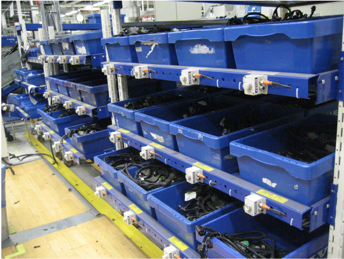
Figure 3.8. An example of a pick-by-light system
