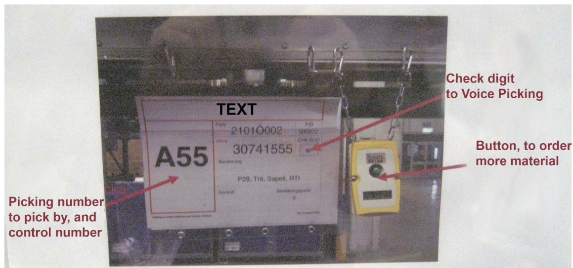
Figure 3.11. An instruction of how to use the pick-by-voice system, located in a storage area
