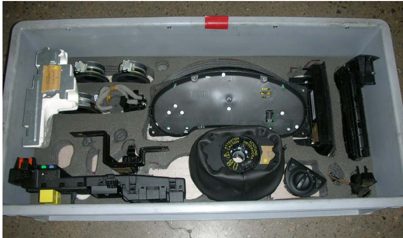
Figure 3.12. An example of a kitting box with cut-outs for the components
