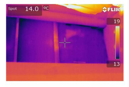
Figure 6 IR image of air leakage paths via the attic stairs
