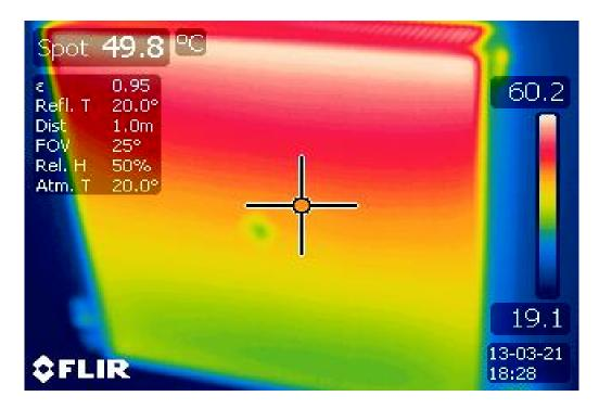
Figure 63 IR image of the radiator near the entrance in the corridor
