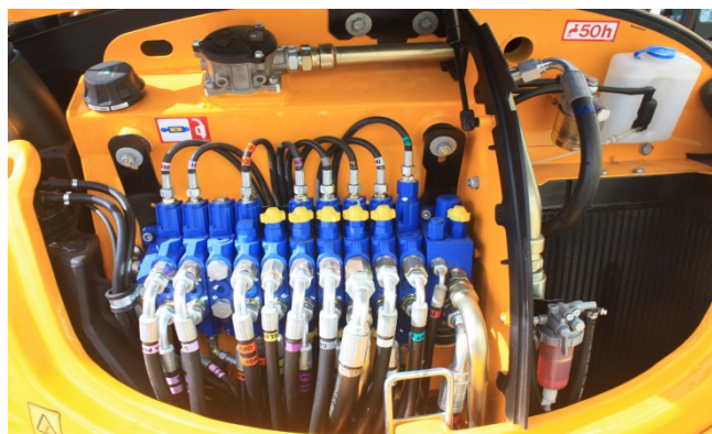
Figure 4-3: Typical Hydraulic Valve Block Installation on off-highway machines
