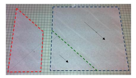
Figure 2.2.4. Picture showing completed 45° ply
