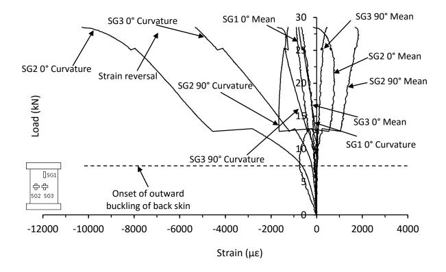
Figure 7.2.28. Mean and curvature strain responses from thin unsymmetrical CP carbon/epoxy panel with 20mm of core removed after a 20J impact (HD-8-6-CP-ICR-20J)
