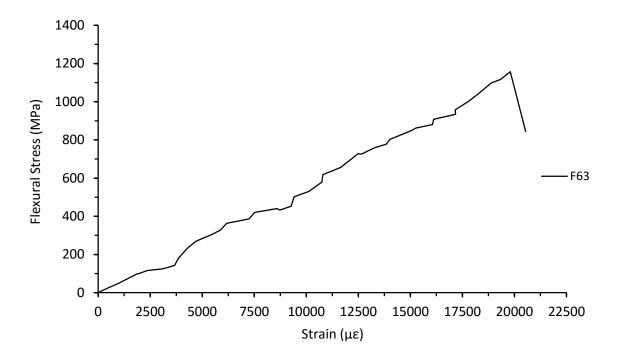
Figure 2.1.5. Flexural strength/strain response from 6 ply multi-directional laminate
