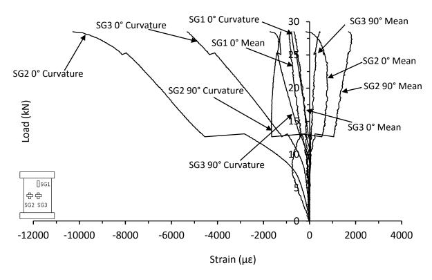
Figure D.18. Mean and curvature strain responses from thin unsymmetrical CP carbon/epoxy panel with 70kg/m<sup>3</sup> core density with 20mm of core removed impacted at 20J (HD-8-6-CP-ICR-20J)
