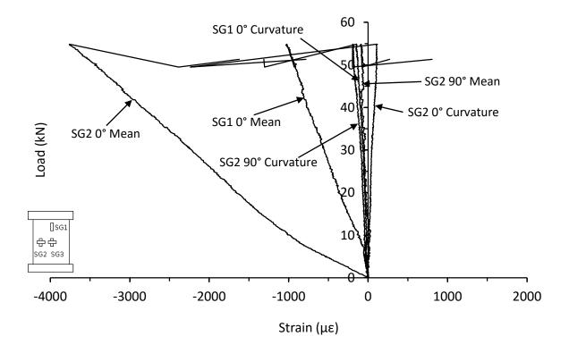
Figure D.26. Mean and curvature strain responses from thin unsymmetrical CP carbon/epoxy panel with 70kg/m<sup>3</sup> core density with 40mm hole drilled in both skins (HD-8-6-CP-2H-B)P
