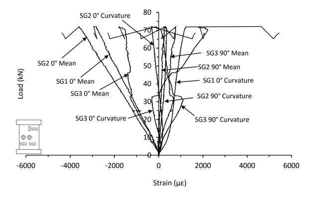
Figure C.62. Mean and curvature strain responses from thin symmetrical CP carbon/epoxy panel with 135kg/m<sup>3</sup> core density impacted at 15J (RM-8-8-CP-15J-A)
