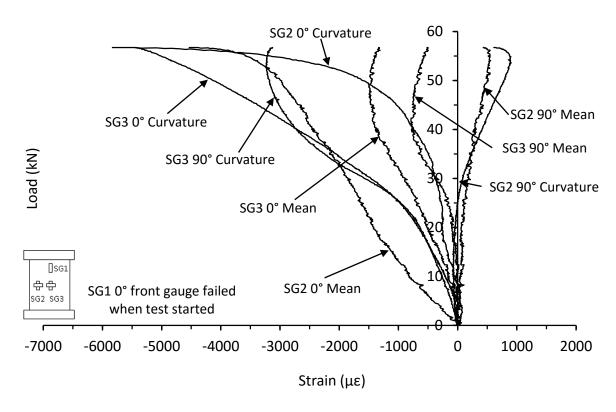
Figure 7.2.26. Mean and curvature strain responses from thin symmetrical CP carbon/epoxy panel with 20mm of core removed after a 10J impact (HD-8-8-CP-ICR-10J)
