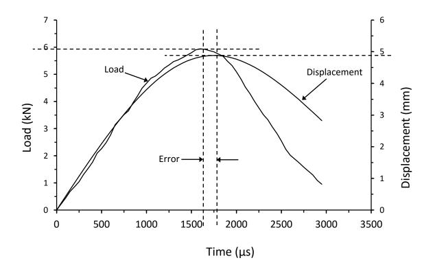
Figure 4.2.4. Load and displacement vs time response for thin symmetrical CP carbon/epoxy panels with 70kg/m<sup>3</sup> core density impacted at 16J (CI-8-8-CP-16J)
