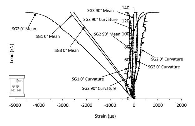
Figure D.8. Mean and curvature strain responses from thick symmetrical CP carbon/epoxy panel with 70kg/m<sup>3</sup> core density with 40mm of core removed (CI-16-16-CP-CR-2)
