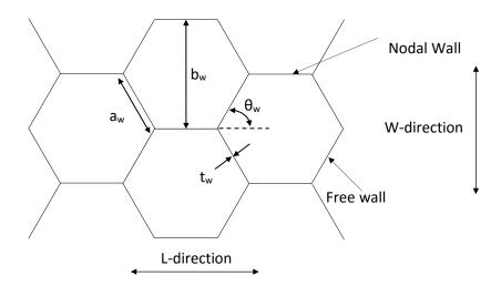
Figure 2.3.1. Diagrammatic representation of honeycomb elements and key geometric definitions
