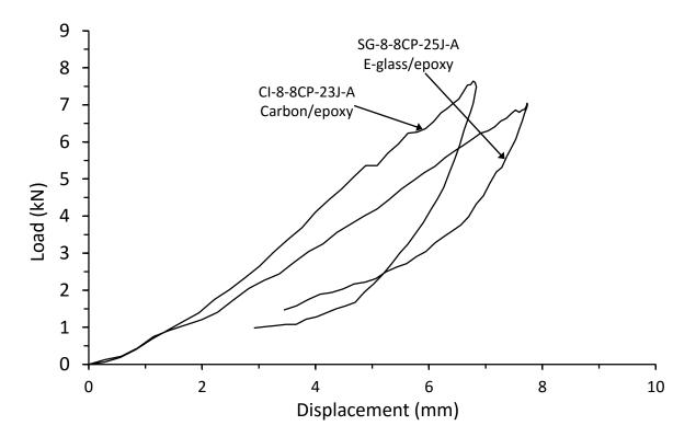
Figure 4.2.25. Load vs displacement response comparison for thin symmetrical CP carbon and E-glass/epoxy panels with 70kg/m<sup>3</sup> core density impacted at 23J and 25J respectively
