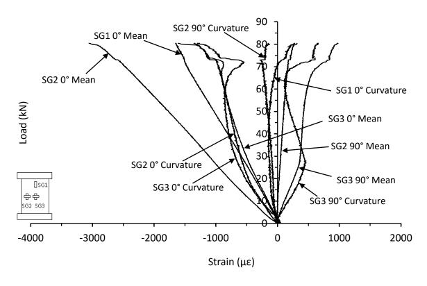
Figure C.42. Mean and curvature strain responses from thick unsymmetrical CP carbon/epoxy panel with 70kg/m<sup>3</sup> core density impacted at 35J (NC-16-12-CP-35J)
