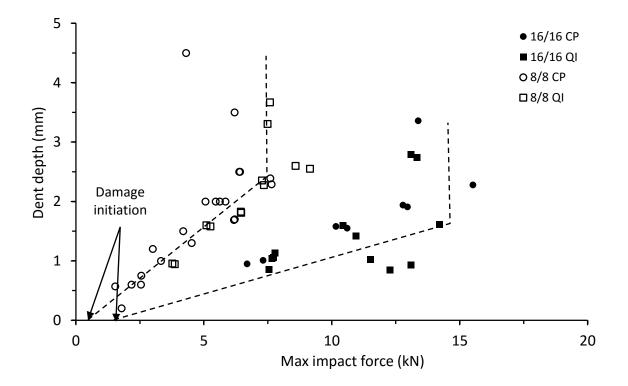
Figure 4.3.9. Dent depth vs maximum impact force for thin and thick symmetrical CP and QI carbon/epoxy panels with 70 kg/m<sup>3</sup> core density
