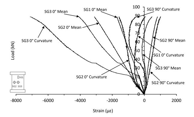
Figure C.45. Mean and curvature strain responses from thick unsymmetrical CP carbon/epoxy panel with 70kg/m<sup>3</sup> core density impacted at 60J (NC-16-12-CP-60J)
