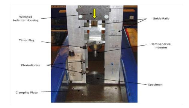
Figure 3.1.1. Drop test rig for low velocity impact testing
