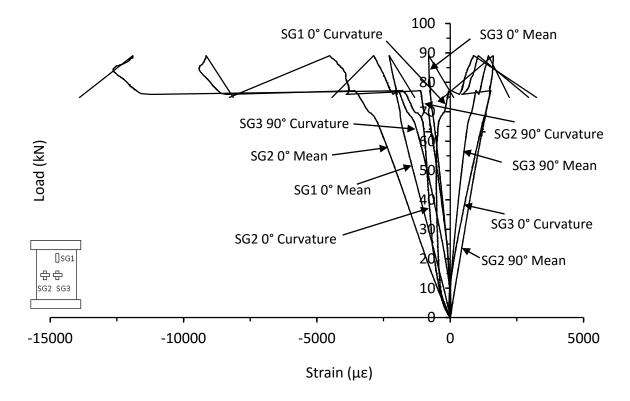
Figure C.50. Mean and curvature strain responses from thick unsymmetrical QI carbon/epoxy panel with 70kg/m<sup>3</sup> core density impacted at 45J (LB-16-12-QI-45J-A)
