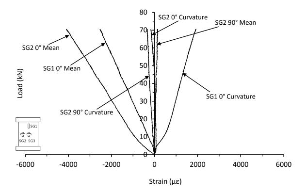
Figure D.19. Mean and curvature strain responses from thin symmetrical CP carbon/epoxy panel with 70kg/m<sup>3</sup> core density with 40mm hole drilled in the top skin (HD-8-8-CP-1H-A)
