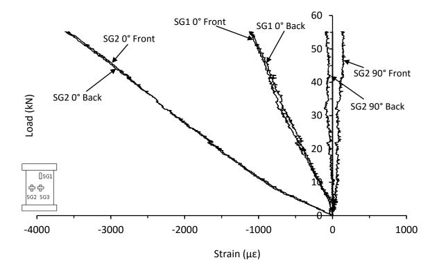
Figure 7.2.32. Strain responses from thin symmetrical CP carbon/epoxy panel with 40mm holes drilled in both skins (HD-8-8-CP-2H-A)
