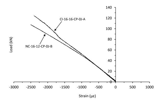
Figure 6.3.6. Mean strain response from the far-field region for thick symmetrical and unsymmetrical CP carbon/epoxy control panels with 70kg/m<sup>3</sup> core density
