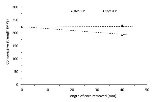
Figure 7.8.2. Compressive strengths of core removed of thick symmetrical and unsymmetrical CP carbon/epoxy panels with 70kg/m<sup>3</sup> core density
