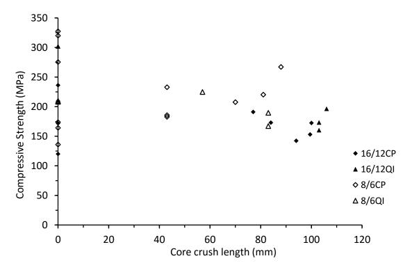
Figure 7.4.8. Compressive strength vs core crush length for thick and thin unsymmetrical CP and QI carbon/epoxy panels 70kg/m<sup>3</sup> core density
