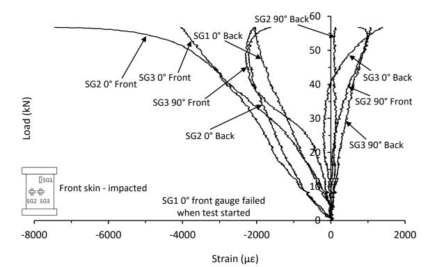
Figure 7.2.25. Strain responses from thin symmetrical CP carbon/epoxy panel with 20mm of core removed after a 10J impact (HD-8-8-CP-ICR-10J)
