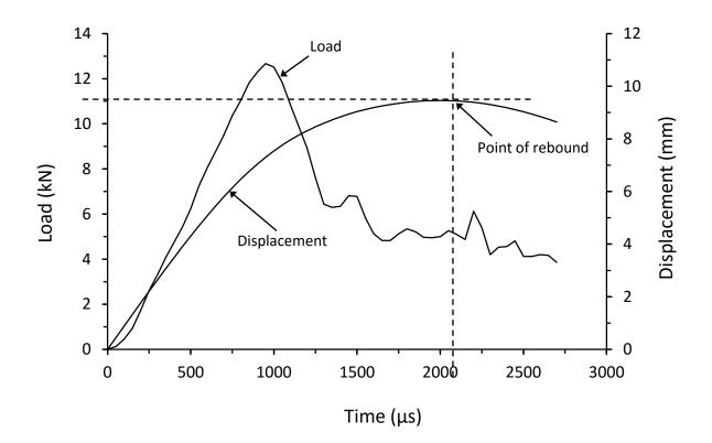
Figure 4.2.8. Load and displacement vs time response for thick symmetrical CP carbon/epoxy panel with 70kg/m<sup>3</sup> core impacted at 60J (CI-16-16-CP-60J-B)
