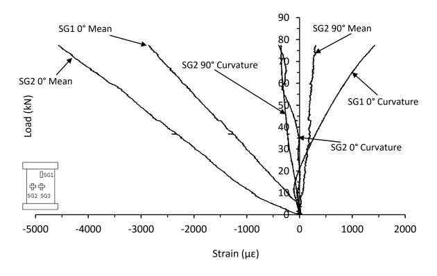
Figure D.24. Mean and curvature strain responses from thin unsymmetrical CP carbon/epoxy panel with 70kg/m<sup>3</sup> core density with 40mm hole drilled in the top skin (HD-8-6-CP-1H-B)
