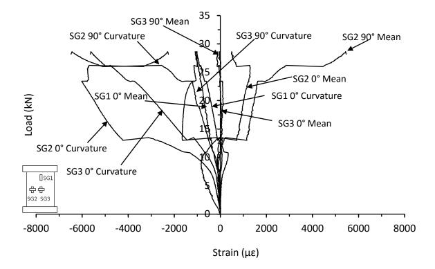
Figure D.17. Mean and curvature strain responses from thin unsymmetrical CP carbon/epoxy panel with 70kg/m<sup>3</sup> core density with 20mm of core removed impacted at 10J (HD-8-6-CP-ICR-10J)
