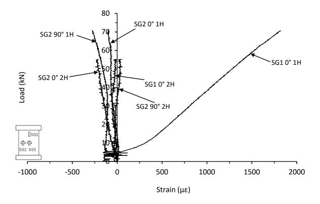
Figure 7.2.34. Comparison of curvature strain responses from thin symmetrical CP carbon/epoxy panels with two 40mm holes (HD-8-8-CP-2H-A) and one 40mm hole drilled (HD-8-8-CP-1H-A)
