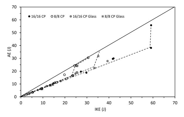
Figure 4.5.12. Absorbed energy vs incident kinetic energy for thin and thick symmetrical CP carbon and Eglass/epoxy panels with 70 kg/m<sup>3</sup> core density
