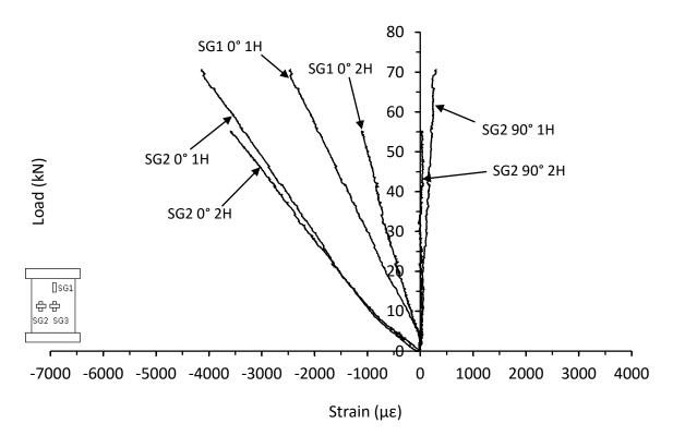
Figure 7.2.33. Comparison of mean strain responses from thin symmetrical CP carbon/epoxy panels with two 40mm holes (HD-8-8-CP-2H-A) and one 40mm hole drilled (HD-8-8-CP-1H-A)
