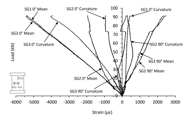
Figure C.21. Mean and curvature strain responses from thin symmetrical QI carbon/epoxy panel with 70kg/m<sup>3</sup> core density impacted at 20J (JL-8-8-QI-20J-B)
