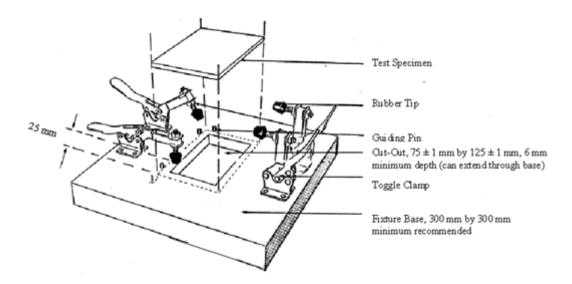
Figure 1.2.2. Clamping arrangement recommended by ASTM D7766/D7766M-11, image from ASTM D7136/D7316M-07
