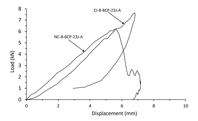
Figure 4.2.19. Load vs displacement response comparison for thin symmetrical and unsymmetrical CP carbon/epoxy panels with 70kg/m<sup>3</sup> core density impacted at 23J
