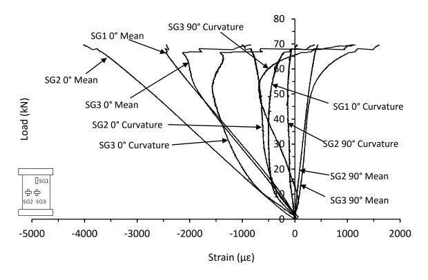
Figure C.14. Mean and curvature strain responses from thin unsymmetrical CP carbon/epoxy panel with 70kg/m<sup>3</sup> core density impacted at 23J (NC-8-6-CP-23J-2)
