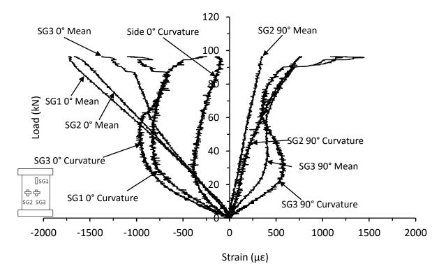
Figure C.30. Mean and curvature strain responses from thick symmetrical CP carbon/epoxy panel with 70kg/m<sup>3</sup> core density impacted at 45J (CI-16-16-CP-45J)
