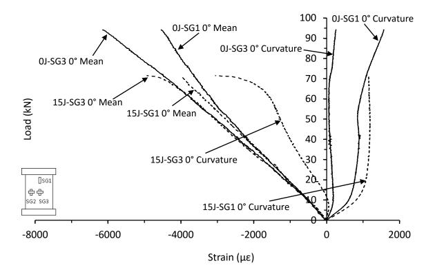
Figure 7.2.9. Mean and curvature strain responses from thin symmetrical QI carbon/epoxy control and 15J impacted panel (JL-8-8-QI-0J-A and JL-8-8-QI-15J-B)
