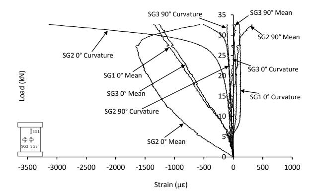
Figure D.13. Mean and curvature strain responses from thin unsymmetrical CP carbon/epoxy panel with 70kg/m<sup>3</sup> core density with 20mm of core removed (HD-8-6-CP-CR-A)
