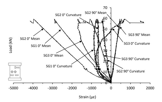
Figure C.7. Mean and curvature strain responses from thin unsymmetrical CP carbon/epoxy panel with 70kg/m<sup>3</sup> core density impacted at 8J (NC-8-6-CP-8J)
