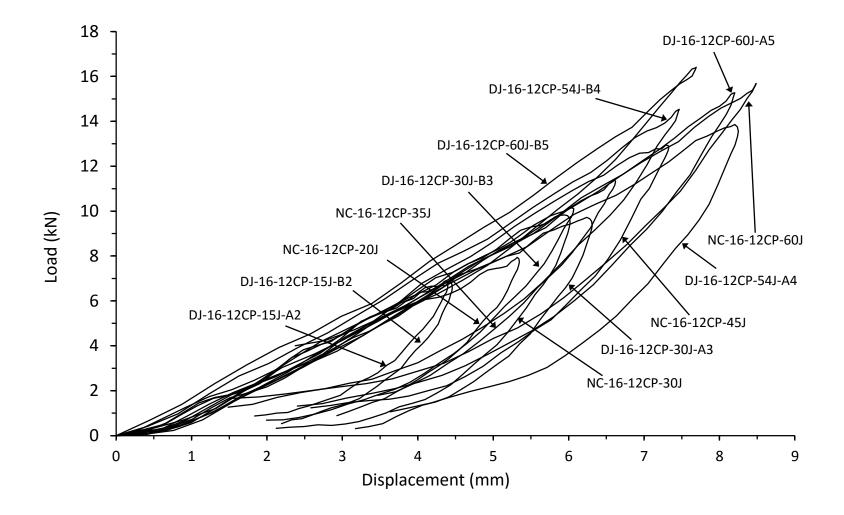
Figure B4. All impact testing load displacement responses from thick unsymmetrical CP carbon/epoxy panels with 70kg/m<sup>3</sup> core density
