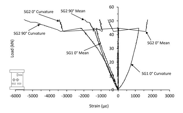
Figure C.69. Mean and curvature strain responses from thin symmetrical CP carbon/epoxy panel with 135kg/m<sup>3</sup> core density impacted at 45J (MB-8-8-CP-45J)
