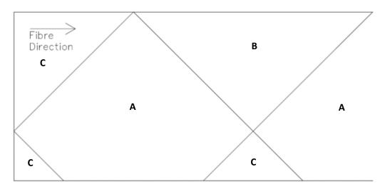
Figure 2.2.2. Cutting plan for 45° plies (A: primary, B: secondary, C: waste)
