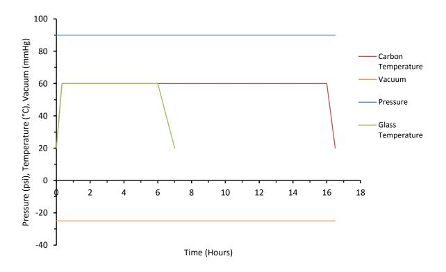
Figure 2.2.6. Autoclave cure cycle for PP1062/LTM26 and 34-700/LTM45-EL
