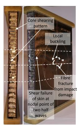
Figure 7.3.4. Photograph of thick unsymmetrical QI carbon/epoxy panel impacted at 60J after in-plane compression showing left external edge and impacted skin front (LB-16-12-QI-60J-A)
