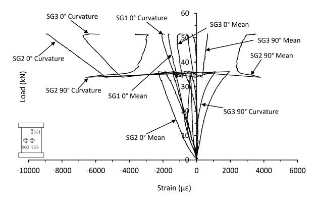
Figure C.54. Mean and curvature strain responses from thin symmetrical CP carbon/epoxy panel with 110kg/m<sup>3</sup> core density impacted at 20J (AR-8-8-CP-20J-A)
