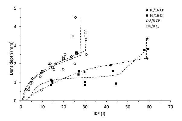
Figure 4.3.5. Dent depth vs incident kinetic energy for thin and thick symmetrical CP and QI carbon/epoxy panels with 70 kg/m<sup>3</sup> core density
