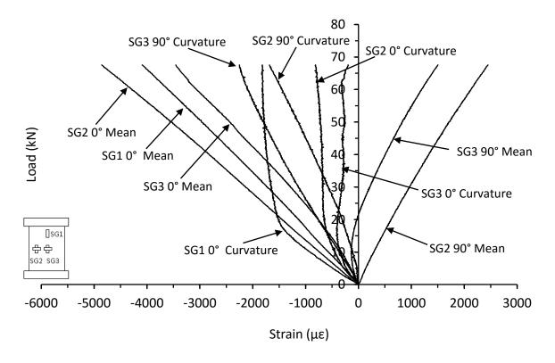
Figure C.26. Mean and curvature strain responses from thin unsymmetrical QI carbon/epoxy panel with 70kg/m<sup>3</sup> core density impacted at 15J (LB-8-6-QI-15J-B)
