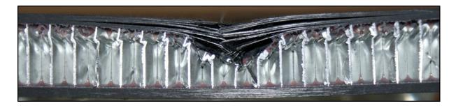
Figure 4.1.3. Cross section of thick symmetrical CP carbon/epoxy panel with 70kg/m<sup>3</sup> core density impacted at 60J (CI-16-16-CP-60J-B)
