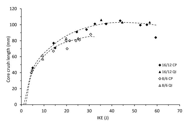
Figure 4.3.4. Core crush length vs incident kinetic energy for thin and thick unsymmetrical CP and QI carbon/epoxy panels with 70 kg/m<sup>3</sup> core density
