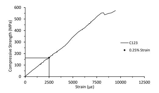
Figure 2.1.4. Compressive stress/strain response from 12 ply multi-directional laminate showing chord point used in modulus calculation, specimen C123
