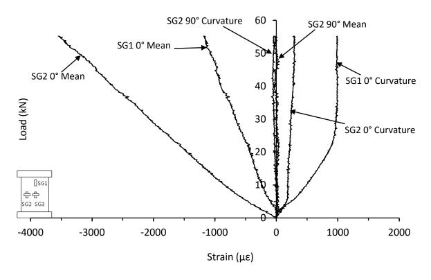
Figure D.22. Mean and curvature strain responses from thin symmetrical CP carbon/epoxy panel with 70kg/m<sup>3</sup> core density with 40mm hole drilled in both skins (HD-8-8-CP-2H-B)
