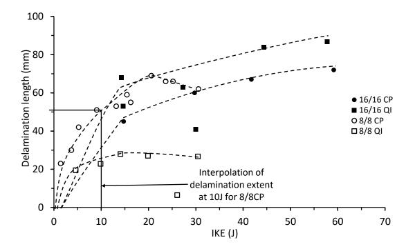
Figure 4.3.1. Delamination length vs incident kinetic energy for thin and thick symmetrical CP carbon/epoxy and QI panels with 70 kg/m<sup>3</sup> core density
