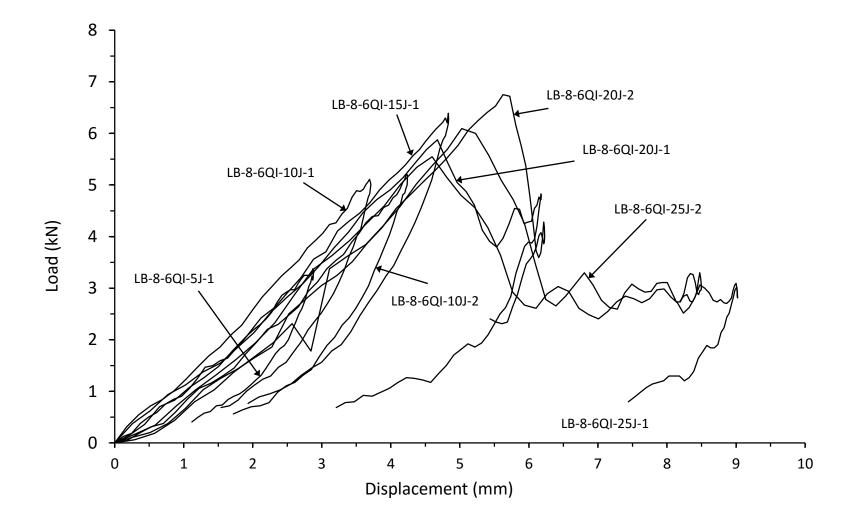
Figure B5. All impact testing load displacement responses from thin symmetrical QI carbon/epoxy panels with 70kg/m<sup>3</sup> core density
