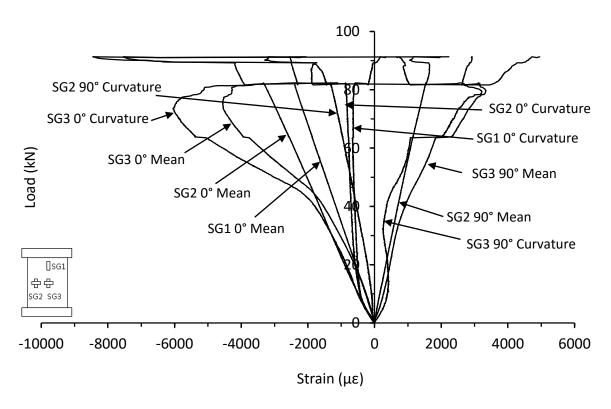
Figure C.48. Mean and curvature strain responses from thick unsymmetrical QI carbon/epoxy panel with 70kg/m<sup>3</sup> core density impacted at 20J (LB-16-12-QI-20J-B)
