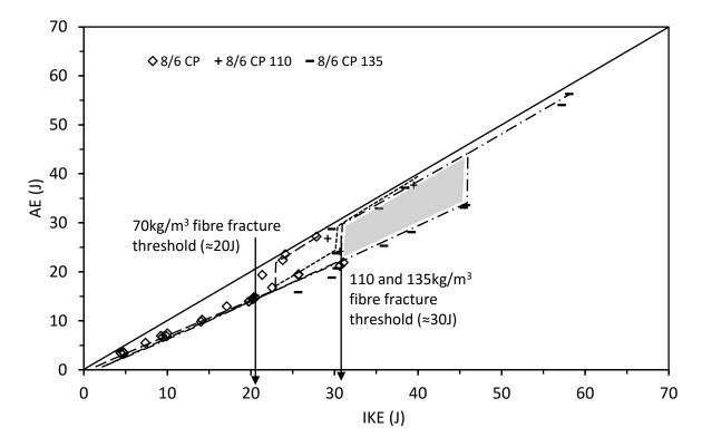
Figure 4.5.6. Absorbed energy vs incident kinetic energy for thin unsymmetrical CP carbon/epoxy panels with 70, 110 and 135 kg/m<sup>3</sup> core densities
