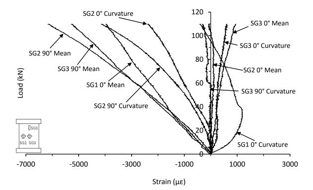
Figure C.85. Mean and curvature strain responses from thick symmetrical CP E-glass/epoxy panel with 70kg/m<sup>3</sup> core density impacted at 25J (SG-16-16-CP-25J)
