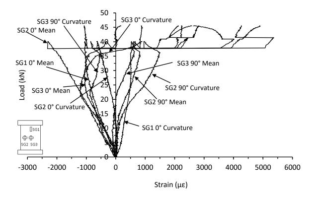
Figure C.68. Mean and curvature strain responses from thin symmetrical CP carbon/epoxy panel with 135kg/m<sup>3</sup> core density impacted at 40J (RM-8-8-CP-40J-A)
