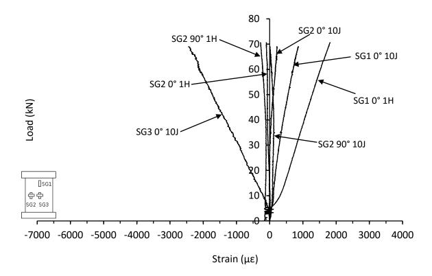
Figure 7.2.31. Comparison of curvature strain responses from thin symmetrical CP carbon/epoxy panels with one 40mm hole drilled (HD-8-8-CP-1H-B) and 10J impact with no precondition (HD-8-8-CP-10J)
