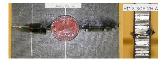
Figure 7.3.9. Post failure image of thin symmetrical CP carbon/epoxy panel with 40mm holes in both skins (HD-8-8-CP-2H-A)
