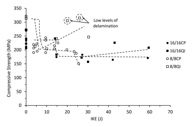
Figure 7.4.1. Compressive strength vs incident kinetic energy for thick and thin symmetrical CP and QI carbon/epoxy panels 70kg/m<sup>3</sup> core density
