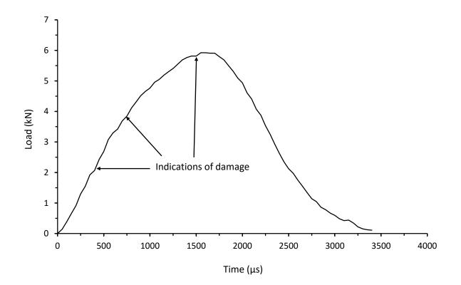
Figure 3.3.2. Load time response for a thin unsymmetrical CP carbon/epoxy panel with 70kg/m<sup>3</sup> core density impacted at 20J (HD-8-6-CP-20J)
