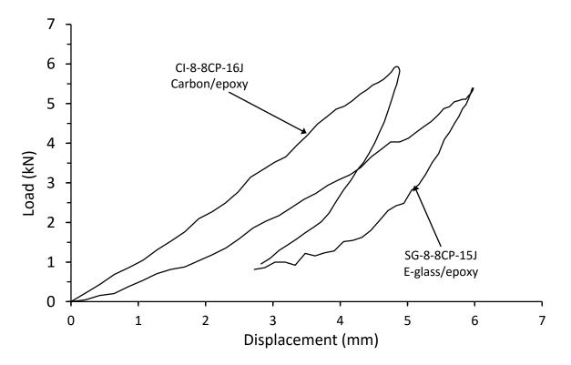
Figure 4.2.24. Load vs displacement response comparison for thin symmetrical CP carbon and E-glass/epoxy panels with 70kg/m<sup>3</sup> core density impacted 16J and 15J respectively
