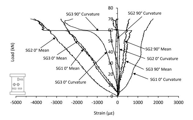
Figure C.11. Mean and curvature strain responses from thin unsymmetrical CP carbon/epoxy panel with 70kg/m<sup>3</sup> core density impacted at 20J (HD-8-6-CP-20J)
