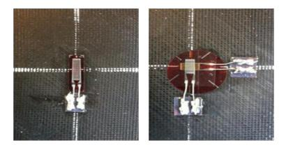
Figure 5.1.5. Bonded and soldered single and rosette strain gauges
