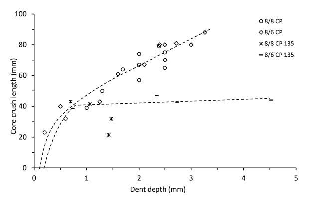
Figure 4.5.8. Core crush length vs dent depth for thin symmetrical and unsymmetrical CP and QI carbon/epoxy panels with 70 and 135 kg/m<sup>3</sup> core densities
