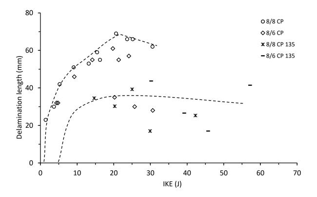
Figure 4.5.1. Delamination length vs incident kinetic energy for thin symmetrical and unsymmetrical CP carbon/epoxy panels with 70 and 135 kg/m<sup>3</sup> core densities
