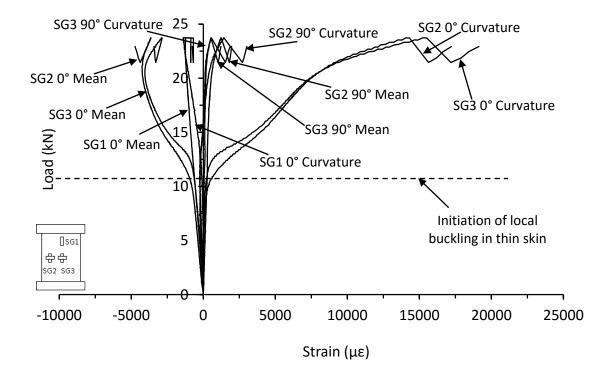
Figure 7.2.15. Mean and curvature strain responses from thin unsymmetrical QI carbon/epoxy panel with 40mm of core removed (LB-8-6-QI-CR-A)
