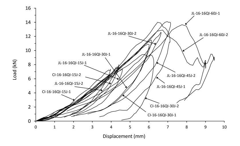
Figure B6. All impact testing load displacement responses from thick symmetrical QI carbon/epoxy panels with 70kg/m<sup>3</sup> core density
