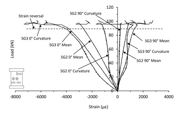
Figure 7.2.6. Mean and curvature strain responses from thick symmetrical QI carbon/epoxy panel with 70kg/m<sup>3</sup> core density impacted at 30J (CI-16-16-QI-30J-A)
