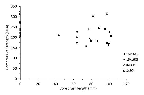
Figure 7.4.7. Compressive strength vs core crush length for thick and thin symmetrical CP and QI carbon/epoxy panels 70kg/m<sup>3</sup> core density
