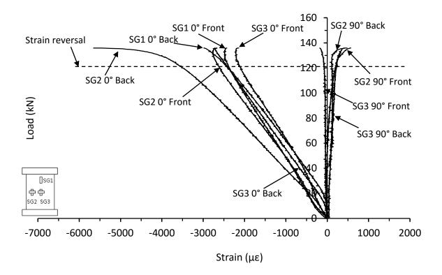
Figure 7.2.17. Strain responses from thick symmetrical CP carbon/epoxy panel with 40mm of core removed (CI-16-16-CP-CR-A)
