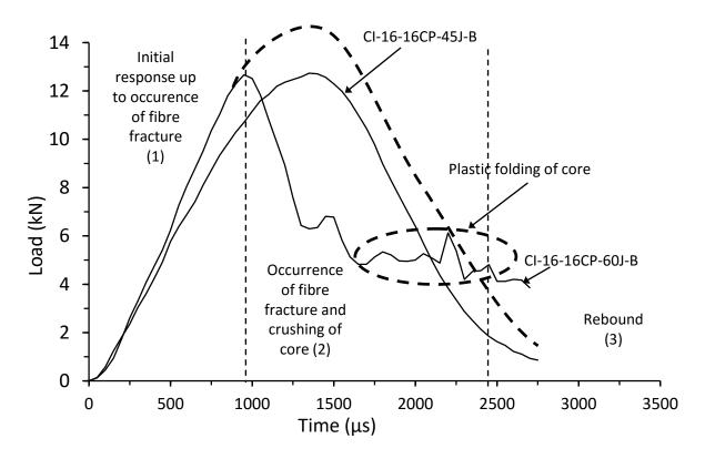
Figure 4.2.5. Load vs time response for thick symmetrical CP carbon/epoxy panels with 70kg/m<sup>3</sup> core density impacted at 45J and 60J
