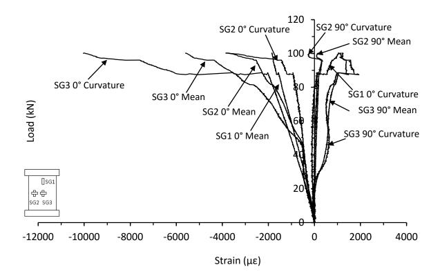
Figure C.31. Mean and curvature strain responses from thick symmetrical CP carbon/epoxy panel with 70kg/m<sup>3</sup> core density impacted at 60J (CI-16-16-CP-60J)
