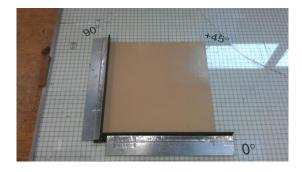
Figure 2.2.5. Angle guide on glass layup table with plies in situ
