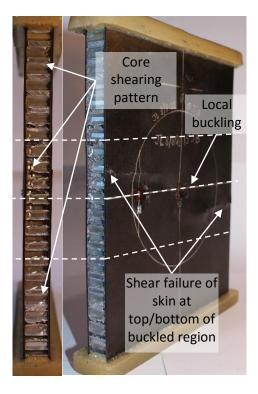
Figure 7.3.1. Photograph of thin symmetrical QI carbon/epoxy panel impacted at 15J after in-plane compression showing left external edge and impacted skin front (JL-8-8-QI-15J)
