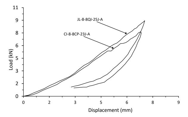
Figure 4.2.22. Load vs displacement response comparison for thin symmetrical CP and QI carbon/epoxy panels with 70kg/m<sup>3</sup> core impacted at 23J and 25J respectively
