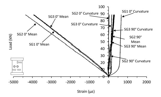
Figure 6.2.1. Mean and curvature strain response for a thin symmetrical CP carbon/epoxy control panel with 135kg/m<sup>3</sup> core density (RM-8-8-CP-0J-B)
