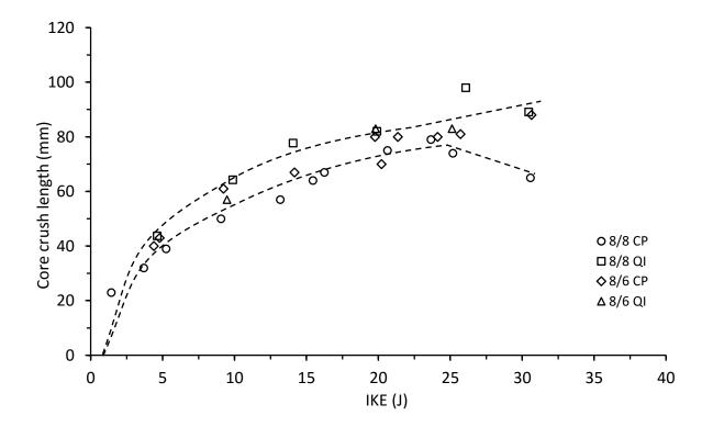
Figure 4.4.4. Core crush length vs incident kinetic energy for thin symmetrical and unsymmetrical CP and QI carbon/epoxy panels with 70 kg/m<sup>3</sup> core density
