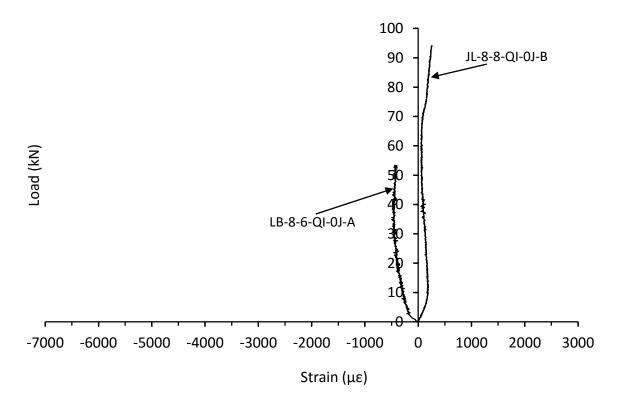
Figure 6.3.8. Curvature strain response from the far-field region for thin symmetrical and unsymmetrical QI carbon/epoxy control panels with 70kg/m<sup>3</sup> core density
