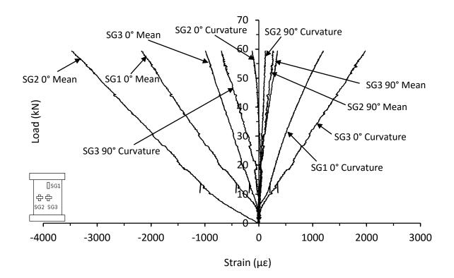
Figure C.3. Mean and curvature strain responses from thin symmetrical CP carbon/epoxy panel with 70kg/m<sup>3</sup> core density impacted at 20J (HD-8-8-CP-20J)
