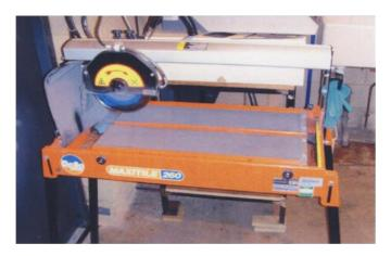
Figure 2.2.10. Diamond edged radial saw
