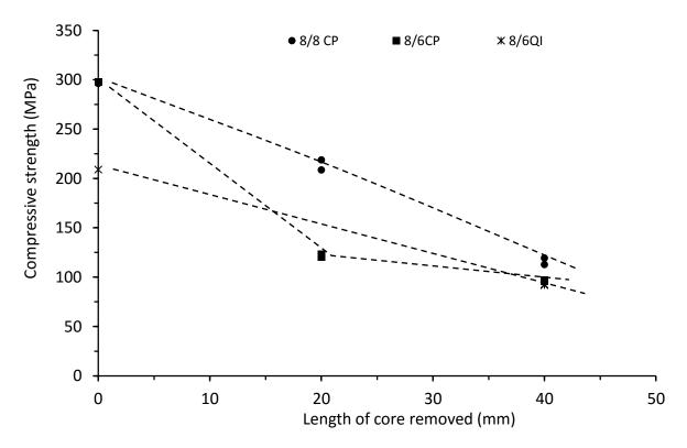
Figure 7.8.1. Compressive strengths of core removed thin symmetrical and unsymmetrical CP and QI carbon/epoxy panels with 70kg/m<sup>3</sup> core density
