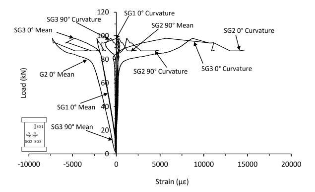
Figure D.9. Mean and curvature strain responses from thick unsymmetrical CP carbon/epoxy panel with 70kg/m<sup>3</sup> core density with 40mm of core removed (NC-16-12-CP-CR-A)
