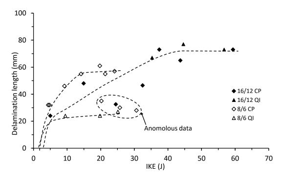
Figure 4.3.2. Delamination length vs incident kinetic energy for thin and thick unsymmetrical CP and QI carbon/epoxy panels with 70 kg/m<sup>3</sup> core density
