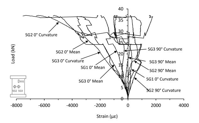
Figure C.77. Mean and curvature strain responses from thin unsymmetrical CP carbon/epoxy panel with 135kg/m<sup>3</sup> core density impacted at 45J (RM-8-6-CP-45J-A)
