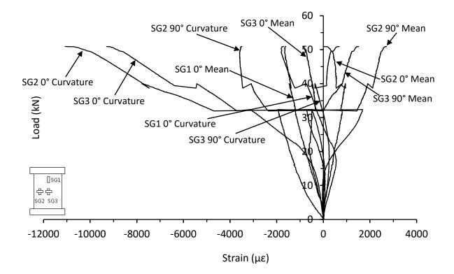
Figure C.55. Mean and curvature strain responses from thin symmetrical CP carbon/epoxy panel with 110kg/m<sup>3</sup> core density impacted at 20J (AR-8-8-CP-20J-B)
