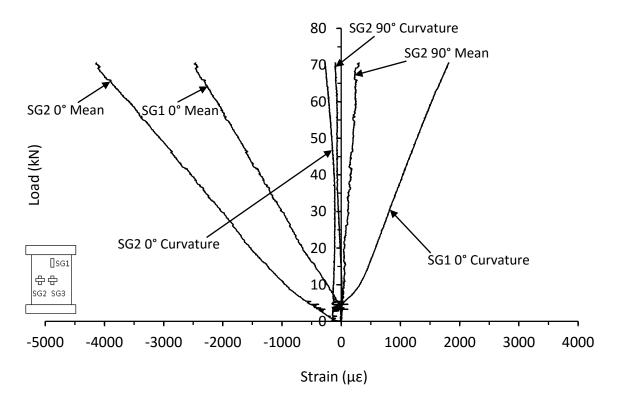
Figure D.20. Mean and curvature strain responses from thin symmetrical CP carbon/epoxy panel with 70kg/m<sup>3</sup> core density with 40mm hole drilled in the top skin (HD-8-8-CP-1H-B)
