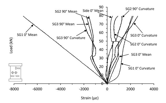
Figure C.79. Mean and curvature strain responses from thin symmetrical CP E-glass/epoxy panel with 70kg/m<sup>3</sup> core density impacted at 8J (SG-8-8-CP-8J)
