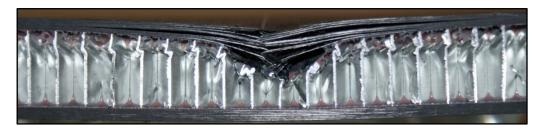
Figure 4.2.7. Cross section of thick symmetrical CP carbon/epoxy panel with 70 kg/m<sup>3</sup> core density impacted at 60J
