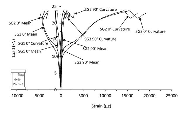
Figure D.5. Mean and curvature strain responses from thin unsymmetrical QI carbon/epoxy panel with 70kg/m<sup>3</sup> core density with 40mm of core removed (LB-8-6-QI-CR-A)
