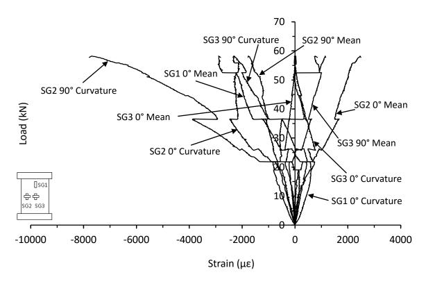
Figure C.66. Mean and curvature strain responses from thin symmetrical CP carbon/epoxy panel with 135kg/m<sup>3</sup> core density impacted at 25J (MB-8-8-CP-25J)
