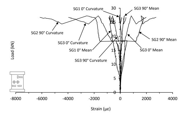
Figure D.16. Mean and curvature strain responses from thin symmetrical CP carbon/epoxy panel with 70kg/m<sup>3</sup> core density with 20mm of core removed impacted at 20J (HD-8-8-CP-ICR-20J)
