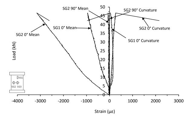
Figure D.25. Mean and curvature strain responses from thin unsymmetrical CP carbon/epoxy panel with 70kg/m<sup>3</sup> core density with 40mm hole drilled in both skins (HD-8-6-CP-2H-A)
