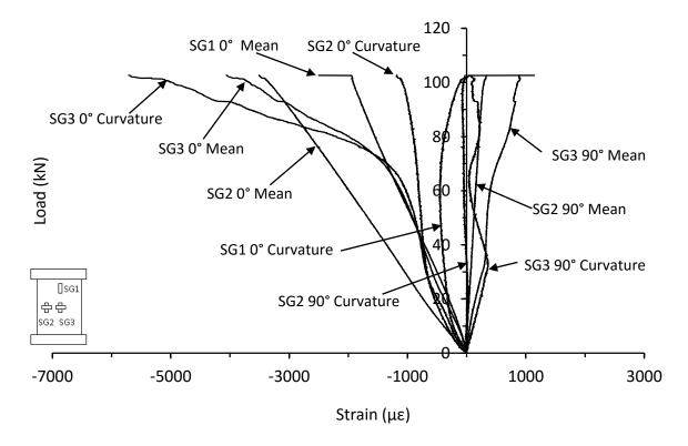
Figure C.40. Mean and curvature strain responses from thick unsymmetrical CP carbon/epoxy panel with 70kg/m<sup>3</sup> core density impacted at 30J (NC-16-12-CP-30J)
