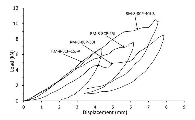
Figure 4.2.16. Load vs displacement response for thin symmetrical CP carbon/epoxy panels with 135kg/m<sup>3</sup> core density impacted at 15J, 25J, 30J, and 40J
