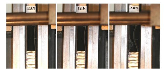
Figure 7.2.16. Progression of local skin buckling in mid-section in thin unsymmetrical QI carbon/epoxy panel with 40mm core removed (LB-8-6-QI-CR-A)
