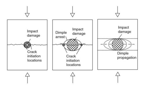
Figure 1.3.5. Failure modes observed in impact damaged sandwich panels under in-plane compression loading from Raju [33]
