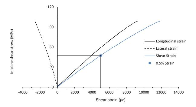
Figure 2.1.7. In-plane shear stress vs. longitudinal, transverse and shear strain responses for specimen IPS61 Using the shear stress-strain relationship, the modulus can be obtained from the chord at 0.5% strain. Poisson's ratio can also be obtained using Equation 2.1.23, using the longitudinal and transverse strain readings at  $3000\mu\epsilon$  and  $1000\mu\epsilon$ .
