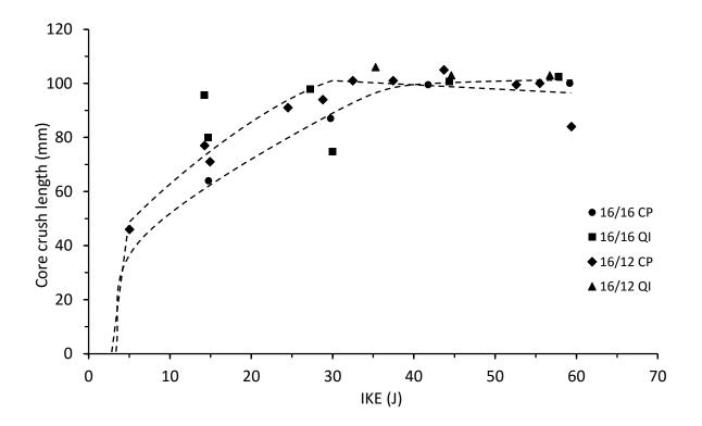
Figure 4.4.3. Core crush length vs incident kinetic energy for thick symmetrical and unsymmetrical CP and QI carbon/epoxy panels with 70 kg/m<sup>3</sup> core density
