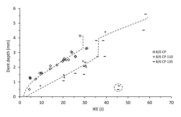
Figure 4.5.4. Dent depth vs incident kinetic energy for thin unsymmetrical CP carbon/epoxy panels with 70, 110 and 135 kg/m<sup>3</sup> core densities
