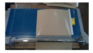
Figure 2.2.1. Prepreg cutting on the guillotine
