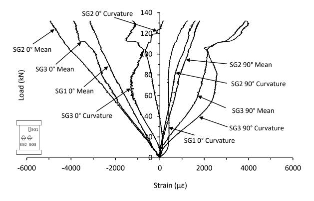
Figure C.36. Mean and curvature strain responses from thick symmetrical QI carbon/epoxy panel with 70kg/m<sup>3</sup> core density impacted at 45J (JL-16-16-QI-45J-B)
