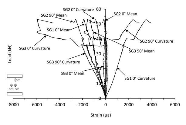
Figure C.70. Mean and curvature strain responses from thin unsymmetrical CP carbon/epoxy panel with 135kg/m<sup>3</sup> core density impacted at 20J (MB-8-6-CP-20J)
