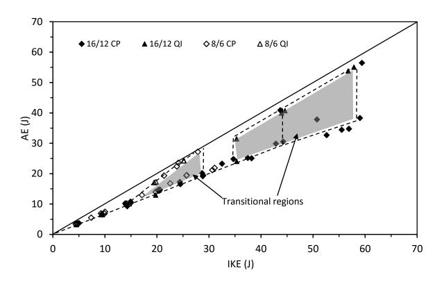
Figure 4.3.8. Absorbed energy vs incident kinetic energy for thin and thick unsymmetrical CP and QI carbon/epoxy panels with 70 kg/m<sup>3</sup> core density
