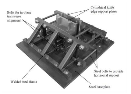
Figure 5.2.1. CAI testing jig
