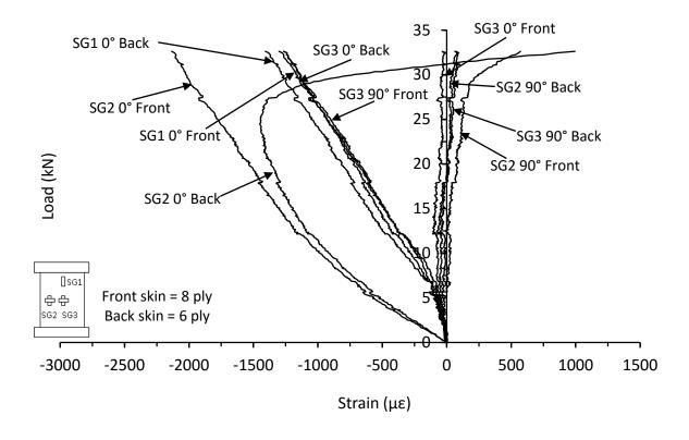
Figure 7.2.23. Strain responses from thin unsymmetrical CP carbon/epoxy panel with 20mm of core removed (HD-8-6-CP-CR-A)
