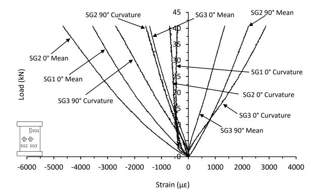
Figure C.27. Mean and curvature strain responses from thin unsymmetrical QI carbon/epoxy panel with 70kg/m<sup>3</sup> core density impacted at 20J (LB-8-6-QI-20J-B)
