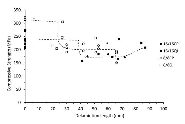
Figure 7.4.5. Compressive strength vs delamination length for thick and thin symmetrical CP and QI carbon/epoxy panels 70kg/m<sup>3</sup> core density
