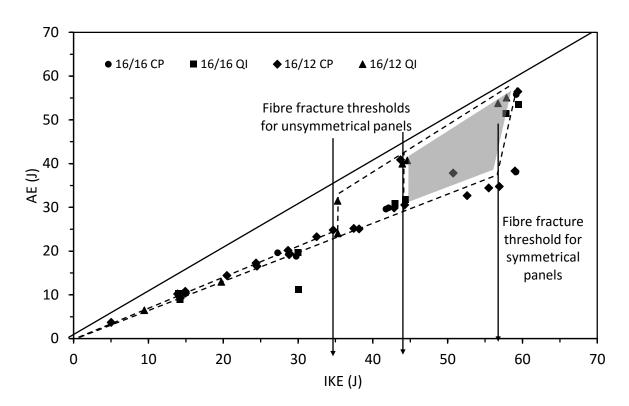
Figure 4.4.7. Absorbed energy vs incident kinetic energy for thick symmetrical and unsymmetrical CP and QI carbon/epoxy panels with 70 kg/m<sup>3</sup> core density
