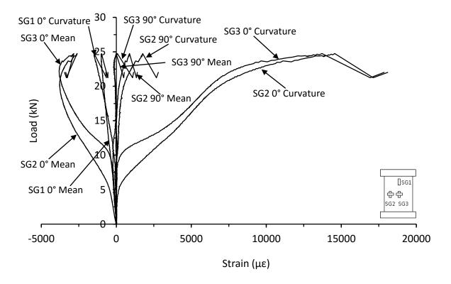
Figure D.4. Mean and curvature strain responses from thin unsymmetrical CP carbon/epoxy panel with 70kg/m<sup>3</sup> core density with 40mm of core removed (NC-8-6-CP-CR-B)
