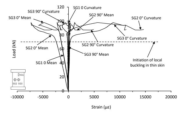
Figure 7.2.20. Mean and curvature strain responses from thick unsymmetrical CP carbon/epoxy panel with 40mm of core removed (NC-16-12-CP-CR-A)
