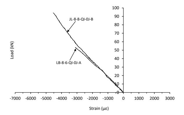
Figure 6.3.7. Mean strain response from the far-field region for thin symmetrical and unsymmetrical QI carbon/epoxy control panels with 70kg/m<sup>3</sup> core density
