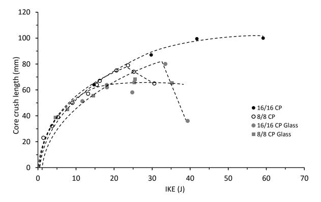
Figure 4.5.10. Core crush length vs incident kinetic energy for thin and thick symmetrical CP carbon and Eglass/epoxy panels with 70 kg/m<sup>3</sup> core density
