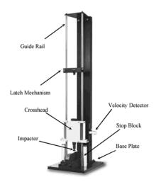
Figure 1.2.1. Sample drop weight tower apparatus suggested in ASTM D7766/D7766M-11, image from ASTM D7136/D7316M-07
