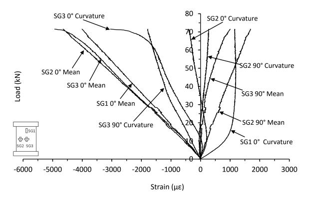
Figure C.20. Mean and curvature strain responses from thin symmetrical QI carbon/epoxy panel with 70kg/m<sup>3</sup> core density impacted at 15J (JL-8-8-QI-15J-B)
