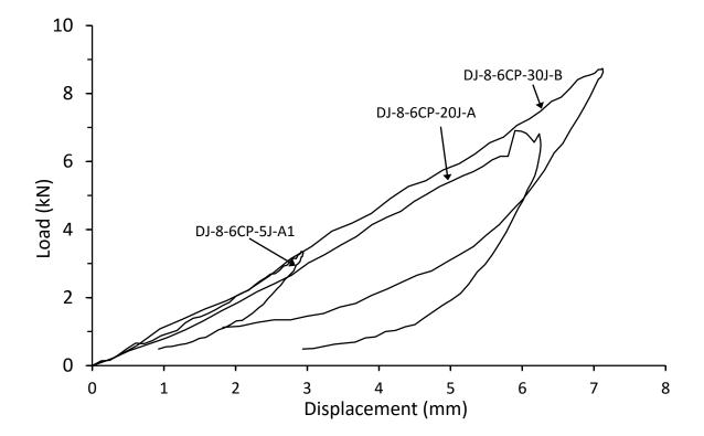
Figure 4.2.13. Load vs displacement response for thin unsymmetrical CP carbon/epoxy panels with 70kg/m<sup>3</sup> core density impacted at 5J, 20J, and 30J
