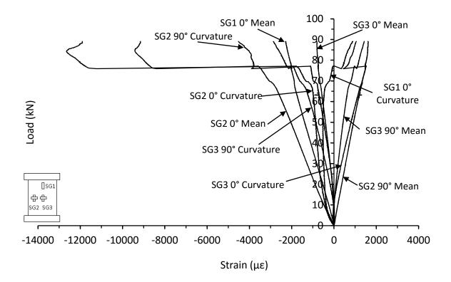
Figure C.51. Mean and curvature strain responses from thick unsymmetrical QI carbon/epoxy panel with 70kg/m<sup>3</sup> core density impacted at 45J (LB-16-12-QI-45J-B)
