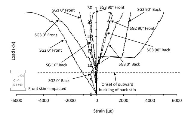
Figure 7.2.27. Strain responses from thin unsymmetrical CP carbon/epoxy panel with 20mm of core removed after a 20J impact (HD-8-6-CP-ICR-20J)
