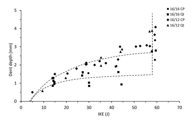
Figure 4.4.5. Dent depth vs incident kinetic energy for thick symmetrical and unsymmetrical CP and QI carbon/epoxy panels with 70 kg/m<sup>3</sup> core density
