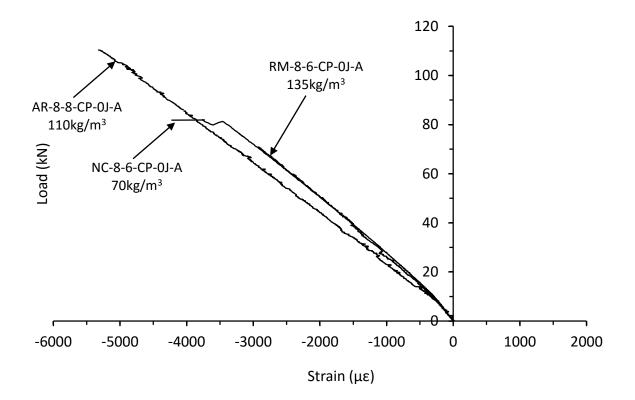
Figure 6.3.12. Mean strain response from the far-field region for thin symmetrical and unsymmetrical CP carbon/epoxy control panels with 70, 110 and 135kg/m<sup>3</sup> core density
