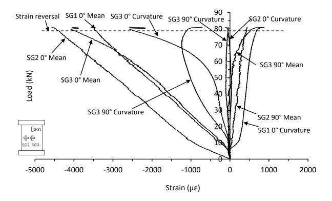
Figure 7.2.4. Mean and curvature strain responses from thin unsymmetrical CP carbon/epoxy panel with 70kg/m<sup>3</sup> core density impacted at 10J (HD-8-6-CP-10)
