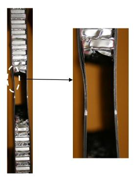
Figure 7.3.7. Post failure image of thin symmetrical CP carbon/epoxy panel with 40mm core removed from mid-section (CI-8-8-CP-CR-1)
