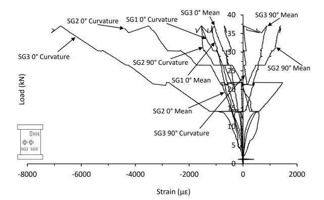
Figure C.59. Mean and curvature strain responses from thin unsymmetrical CP carbon/epoxy panel with 110kg/m<sup>3</sup> core density impacted at 20J (AR-8-6-CP-20J-A)
