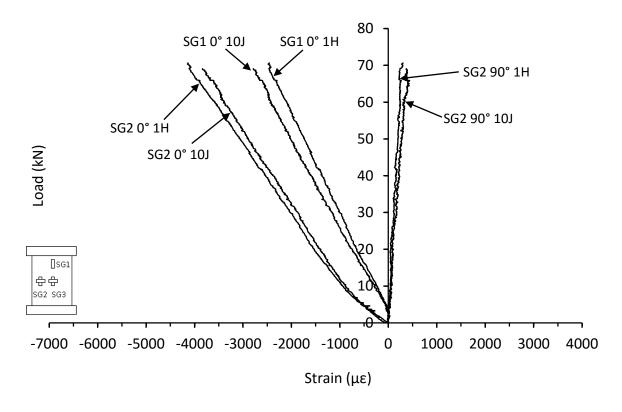
Figure 7.2.30. Comparison of mean strain responses from thin symmetrical CP carbon/epoxy panels with one 40mm hole drilled (HD-8-8-CP-1H-B) and 10J impact with no precondition (HD-8-8-CP-10J)
