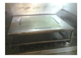
Figure 2.3.2. Oven table with bagging release film tapped down ready for skin/core bonding
