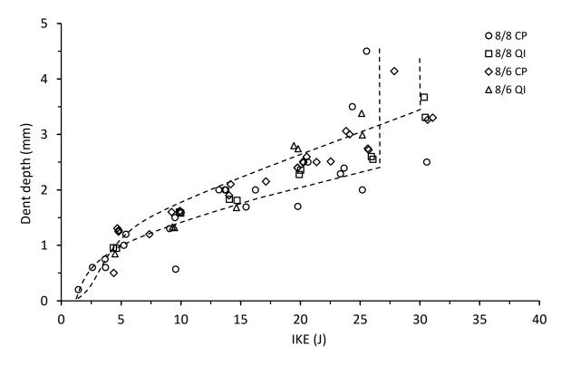
Figure 4.4.6. Dent depth vs incident kinetic energy for thin symmetrical and unsymmetrical CP and QI carbon/epoxy panels with 70 kg/m<sup>3</sup> core density
