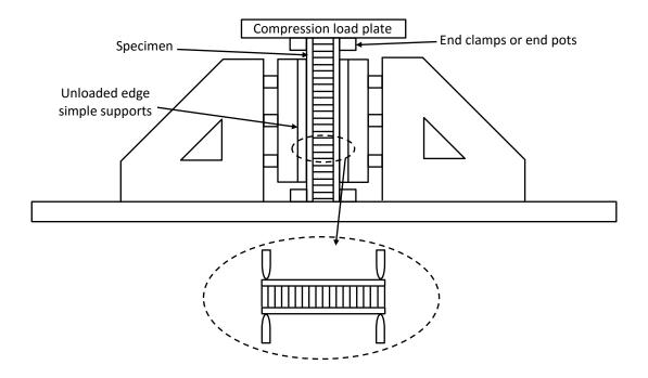
Figure 1.3.4. In-plane compression set up with clamped loaded ends and simply supported at the unloaded sides
