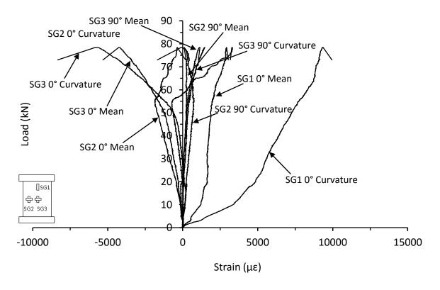
Figure C.44. Mean and curvature strain responses from thick unsymmetrical CP carbon/epoxy panel with 70kg/m<sup>3</sup> core density impacted at 54J (DJ-16-12-CP-54J-A)
