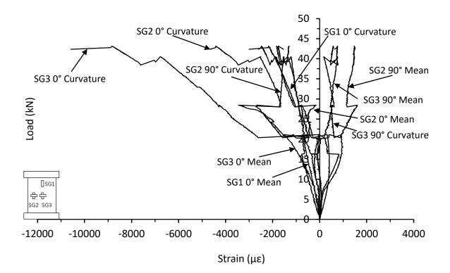
Figure C.75. Mean and curvature strain responses from thin unsymmetrical CP carbon/epoxy panel with 135kg/m<sup>3</sup> core density impacted at 38J (RM-8-6-CP-38J-A)
