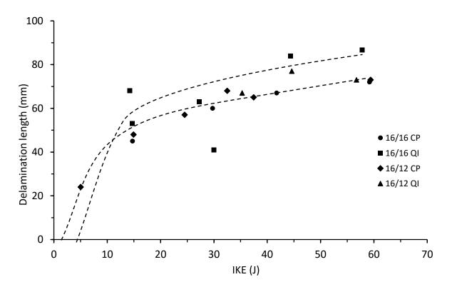
Figure 4.4.1. Delamination length vs incident kinetic energy for thick symmetrical and unsymmetrical CP and QI carbon/epoxy panels with 70 kg/m<sup>3</sup> core density
