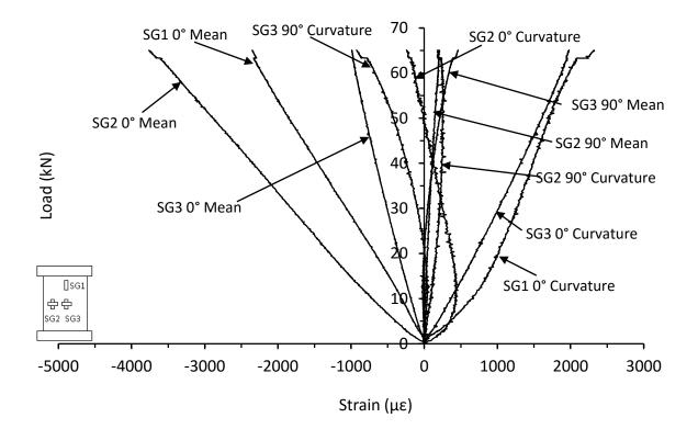
Figure C.13. Mean and curvature strain responses from thin unsymmetrical CP carbon/epoxy panel with 70kg/m<sup>3</sup> core density impacted at 23J (NC-8-6-CP-23J-1)
