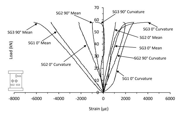
Figure C.82. Mean and curvature strain responses from thin symmetrical CP E-glass/epoxy panel with 70kg/m<sup>3</sup> core density impacted at 35J (SG-8-8-CP-35J)
