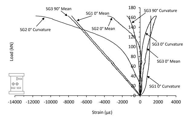
Figure C.84. Mean and curvature strain responses from thick symmetrical CP E-glass/epoxy panel with 70kg/m<sup>3</sup> core density impacted at 18J (SG-16-16-CP-18J)
