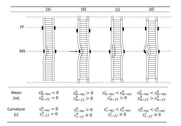
Figure 7.10.4. Illustration of the probable buckling deformation process of impact damaged panels under inplane compression in the longitudinal loading direction.
