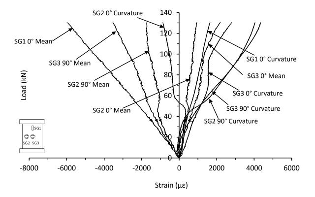
Figure C.87. Mean and curvature strain responses from thick symmetrical CP E-glass/epoxy panel with 70kg/m<sup>3</sup> core density impacted at 45J (SG-16-16-CP-45J)
