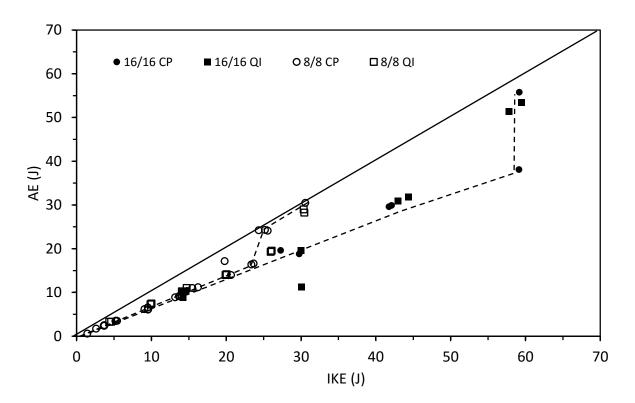
Figure 4.3.7. Absorbed energy vs incident kinetic energy for thin and thick symmetrical CP and QI carbon/epoxy panels with 70 kg/m<sup>3</sup> core density
