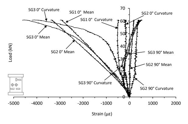
Figure C.4. Mean and curvature strain responses from thin unsymmetrical CP carbon/epoxy panel with 70kg/m<sup>3</sup> core density impacted at 5J (DJ-8-6-CP-5J-A2)
