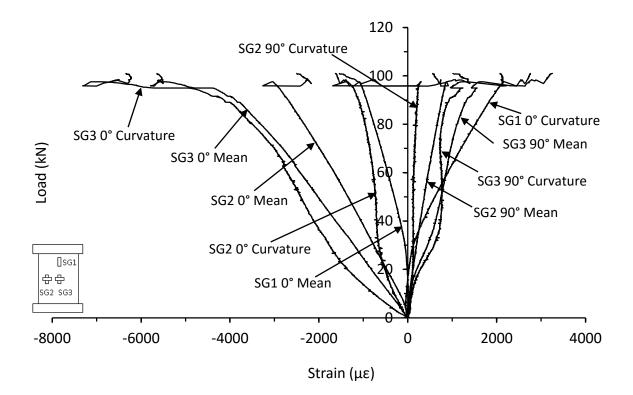
Figure C.35. Mean and curvature strain responses from thick symmetrical QI carbon/epoxy panel with 70kg/m<sup>3</sup> core density impacted at 30J (CI-16-16-QI-30J)
