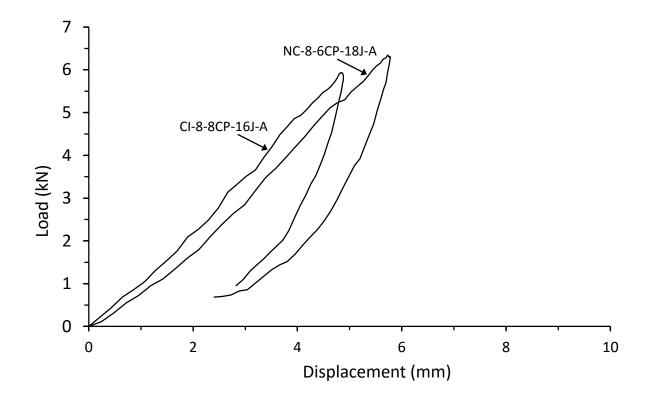
Figure 4.2.18. Load vs displacement response comparison for thin symmetrical and unsymmetrical CP carbon/epoxy panels with 70kg/m<sup>3</sup> core density impacted at 16J and 18J respectively
