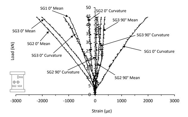
Figure C.5. Mean and curvature strain responses from thin unsymmetrical CP carbon/epoxy panel with 70kg/m<sup>3</sup> core density impacted at 5J (DJ-8-6-CP-5J-A3)
