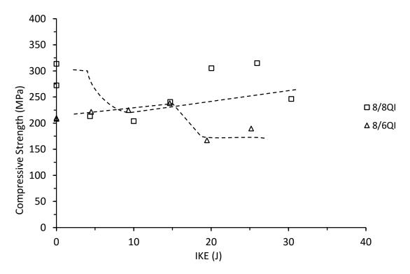
Figure 7.5.2. Compressive strength vs incident kinetic energy for thin symmetrical and unsymmetrical QI carbon/epoxy panels with 70kg/m<sup>3</sup> core density
