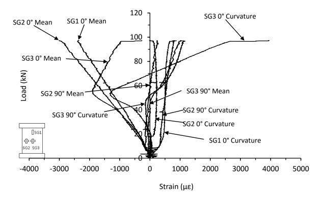
Figure C.38. Mean and curvature strain responses from thick unsymmetrical CP carbon/epoxy panel with 70kg/m<sup>3</sup> core density impacted at 15J (DJ-16-12-CP-15J-A)
