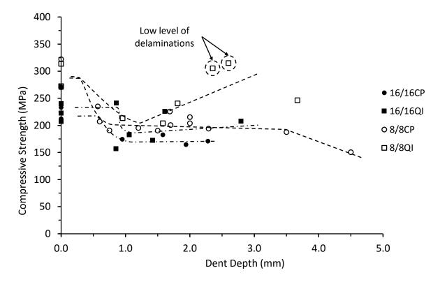
Figure 7.4.3. Compressive strength vs dent depth for thick and thin symmetrical CP and QI carbon/epoxy panels 70kg/m<sup>3</sup> core density
