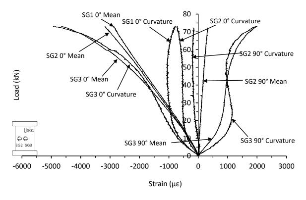
Figure C.8. Mean and curvature strain responses from thin unsymmetrical CP carbon/epoxy panel with 70kg/m<sup>3</sup> core density impacted at 10J (NC-8-6-CP-10J)
