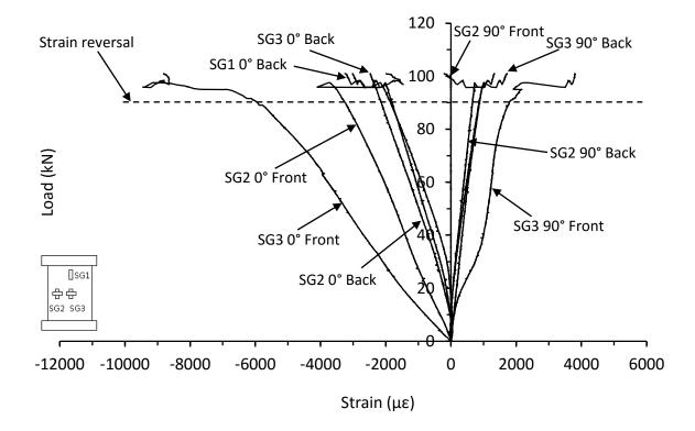
Figure 7.2.5. Strain responses from thick symmetrical QI carbon/epoxy panel with 70kg/m<sup>3</sup> core density impacted at 30J (CI-16-16-QI-30J-A)
