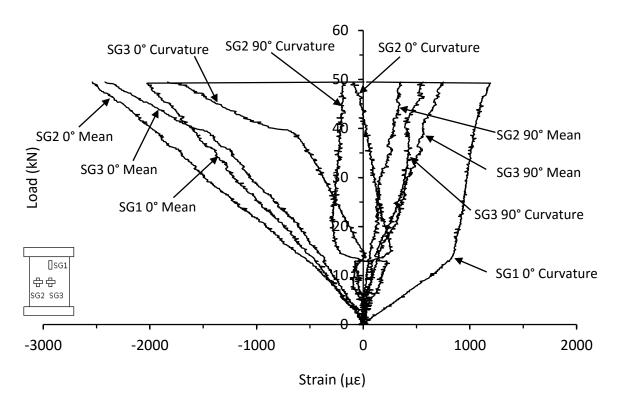
Figure C.12. Mean and curvature strain responses from thin unsymmetrical CP carbon/epoxy panel with 70kg/m<sup>3</sup> core density impacted at 20J (DJ-8-6-CP-20-A)
