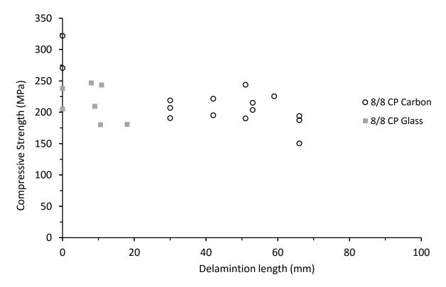
Figure 7.7.2. Compressive strength vs delamination length for thin symmetrical CP carbon and E-glass/epoxy panels with 70kg/m<sup>3</sup> core density
