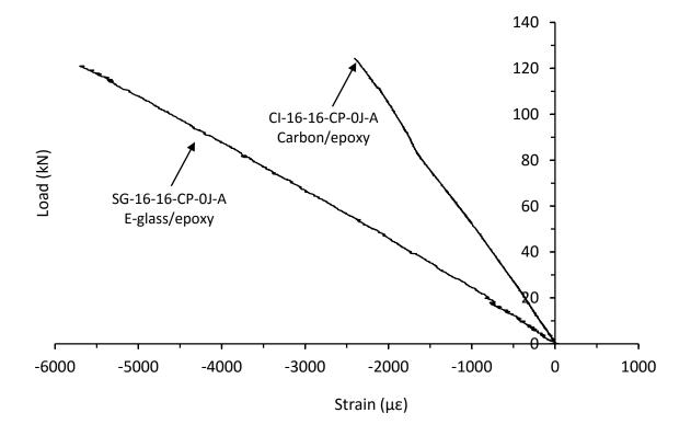
Figure 6.3.14. Mean strain response from the far-field region for thick symmetrical CP carbon and Eglass/epoxy panels with 70kg/m<sup>3</sup> core density
