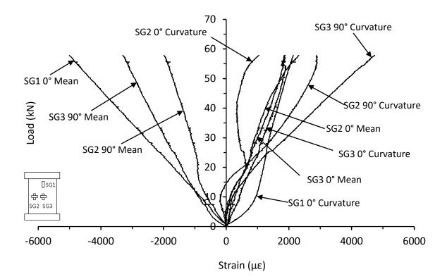
Figure C.81. Mean and curvature strain responses from thin symmetrical CP E-glass/epoxy panel with 70kg/m<sup>3</sup> core density impacted at 25J (SG-8-8-CP-25J)
