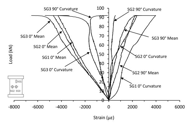
Figure C.22. Mean and curvature strain responses from thin symmetrical QI carbon/epoxy panel with 70kg/m<sup>3</sup> core density impacted at 25J (JL-8-8-QI-25J-B)
