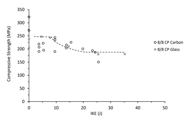
Figure 7.7.1. Compressive strength vs incident kinetic energy for thin symmetrical CP carbon and Eglass/epoxy panels with 70kg/m<sup>3</sup> core density
