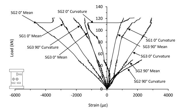
Figure C.37. Mean and curvature strain responses from thick symmetrical QI carbon/epoxy panel with 70kg/m<sup>3</sup> core density impacted at 60J (JL-16-16-QI-60J-B)
