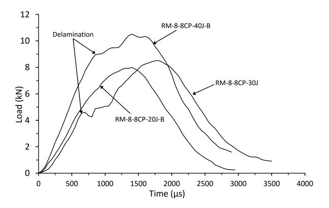
Figure 4.2.9. Load vs time response for thin symmetrical CP carbon/epoxy panels with 135 kg/m<sup>3</sup> core density impacted at 20J, 30J and 40J
