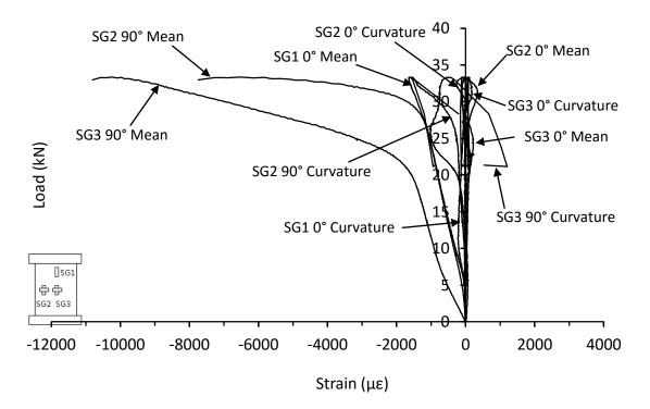
Figure D.2. Mean and curvature strain responses from thin symmetrical CP carbon/epoxy panel with 70kg/m<sup>3</sup> core density with 40mm of core removed (CI-8-8-CP-CR-2)
