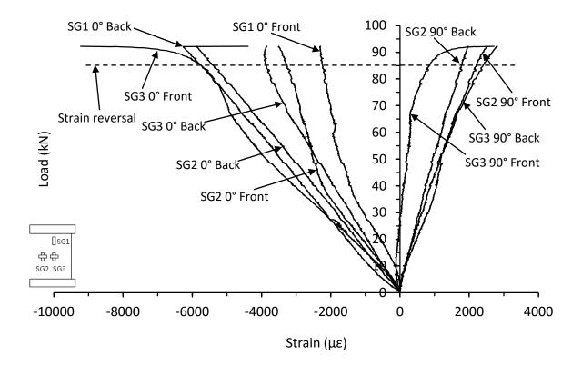
Figure 7.2.1. Strain responses from thin symmetrical QI carbon/epoxy panel with 70kg/m<sup>3</sup> core density impacted at 25J (JL-8-8-QI-25J-B)
