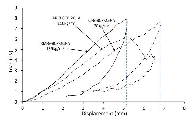
Figure 4.2.26 Load vs displacement response comparison for thin symmetrical CP carbon/epoxy panels with 70, 110 and 135kg/m<sup>3</sup> core densities impacted at 23J, 20J and 20J respectively
