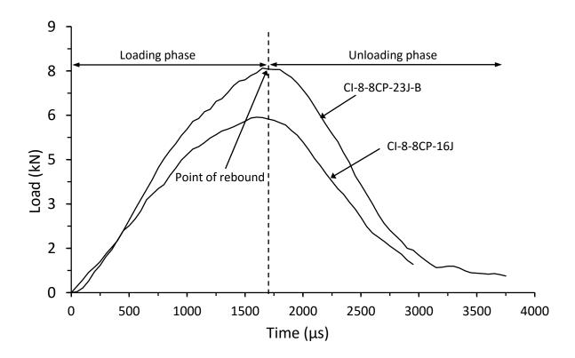
Figure 4.2.1. Load vs time response for thin symmetrical CP carbon/epoxy panels with 70kg/m<sup>3</sup> core density impacted at 16J and 23J
