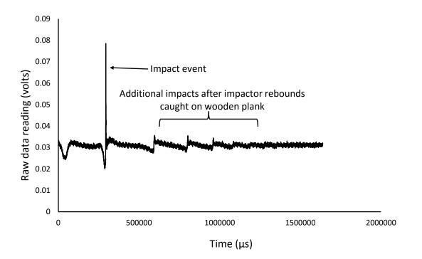
Figure 3.3.1.Raw data response for a thin unsymmetrical CP carbon/epoxy panel with 70kg/m<sup>3</sup> core density impacted at 20J (HD-8-6-CP-20J)
