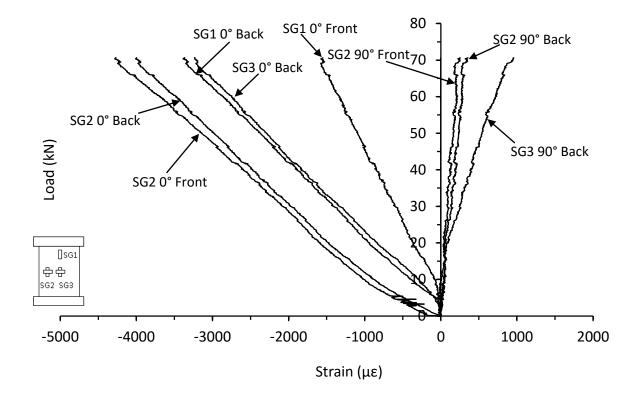
Figure 7.2.29. Strain responses from thin symmetrical CP carbon/epoxy panel with one 40mm hole drilled in the top skin (HD-8-8-CP-1H-B)
