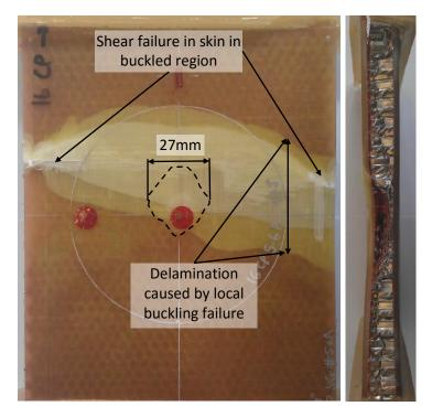
Figure 7.3.6. Photograph of thick symmetrical CP E-glass/epoxy panel impacted at 45J after in-plane compression showing impacted skin front and right external edge (SG-16-16-CP-45J)
