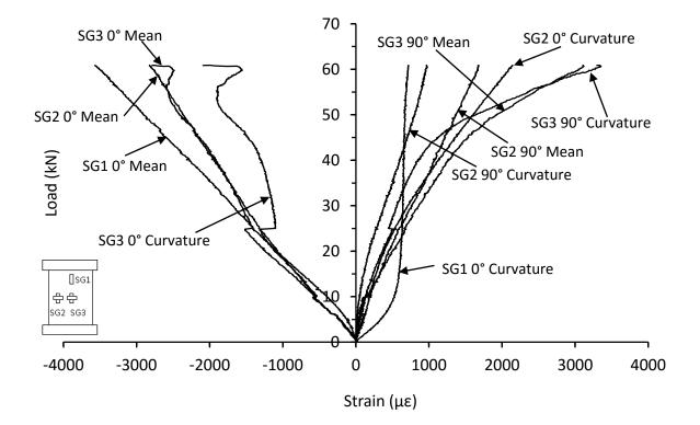
Figure C.19. Mean and curvature strain responses from thin symmetrical QI carbon/epoxy panel with 70kg/m<sup>3</sup> core density impacted at 10J (JL-8-8-QI-10J-B)
