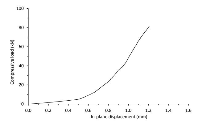
Figure 5.3.3. Compressive load against in-plane LVDT displacement for a thick symmetrical QI carbon/epoxy control panel with 70kg/m<sup>3</sup> core density (CI-16-16-QI-OJ-A)
