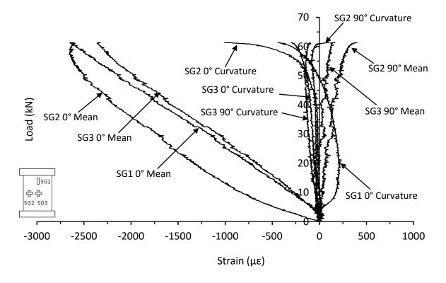
Figure 7.2.22. Mean and curvature strain responses from thin symmetrical CP carbon/epoxy panel with 20mm of core removed (HD-8-8-CP-CR-A)
