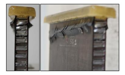
Figure 6.1.4. Observed shear band mechanism failure in thin symmetrical CP carbon/epoxy panels with 135kg/m<sup>3</sup> core (RM-8-8-CP-0J-B)
