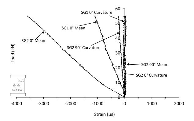
Figure D.21. Mean and curvature strain responses from thin symmetrical CP carbon/epoxy panel with 70kg/m<sup>3</sup> core density with 40mm hole drilled in both skins (HD-8-8-CP-2H-A)
