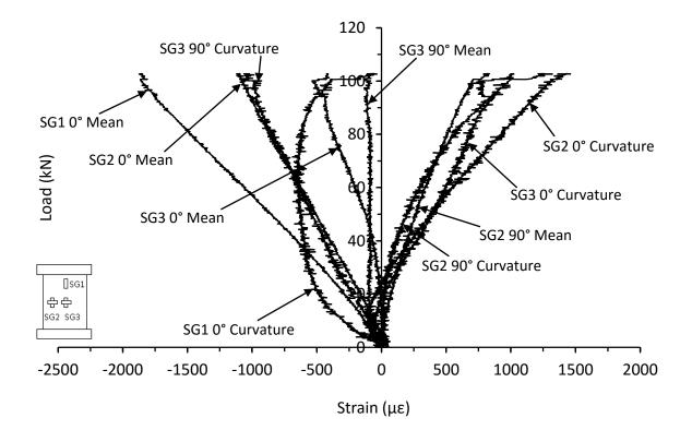
Figure C.29. Mean and curvature strain responses from thick symmetrical CP carbon/epoxy panel with 70kg/m<sup>3</sup> core density impacted at 15J (CI-16-16-CP-15J)
