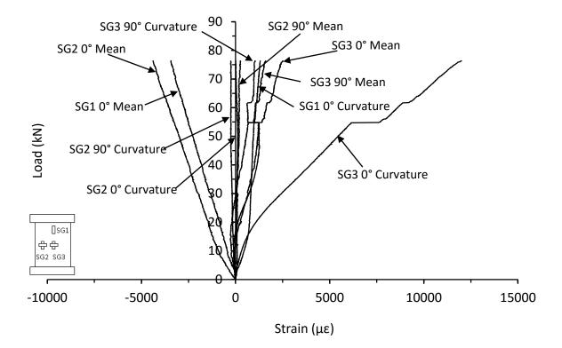
Figure C.57. Mean and curvature strain responses from thin unsymmetrical CP carbon/epoxy panel with 110kg/m<sup>3</sup> core density impacted at 10J (AR-8-6-CP-10J)
