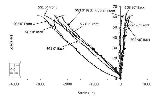
Figure 7.2.21. Strain responses from thin symmetrical CP carbon/epoxy panel with 20mm of core removed (HD-8-8-CP-CR-A)
