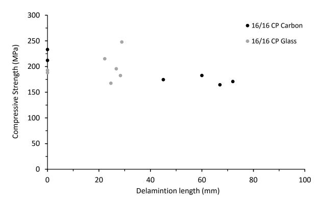
Figure 7.7.4. Compressive strength vs delamination length for thick symmetrical CP carbon and Eglass/epoxy panels with 70kg/m<sup>3</sup> core density
