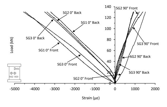
Figure 5.3.4. Strain response from a thick symmetrical QI carbon/epoxy control panel with 70kg/m<sup>3</sup> core density (CI-16-16-QI-OJ-A)
