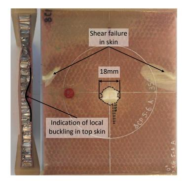
Figure 7.3.5. Photograph of thin symmetrical CP E-glass/epoxy panel impacted at 35J after in-plane compression showing left external edge and impacted skin front (SG-8-8-CP-35J)
