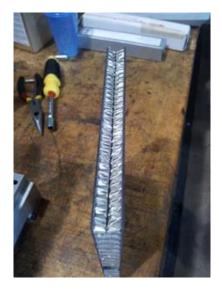
Figure 5.1.2. Photo of V-notch cut into top of panel to improve epoxy penetration
