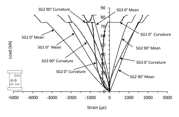
Figure C.52. Mean and curvature strain responses from thick unsymmetrical QI carbon/epoxy panel with 70kg/m<sup>3</sup> core density impacted at 60J (LB-16-12-QI-60J-A)
