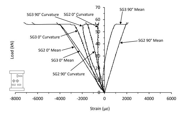
Figure C.25. Mean and curvature strain responses from thin unsymmetrical QI carbon/epoxy panel with 70kg/m<sup>3</sup> core density impacted at 10J (LB-8-6-QI-10J-B)
