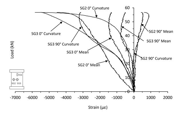
Figure D.15. Mean and curvature strain responses from thin symmetrical CP carbon/epoxy panel with 70kg/m<sup>3</sup> core density with 20mm of core removed impacted at 10J (HD-8-8-CP-ICR-10J)
