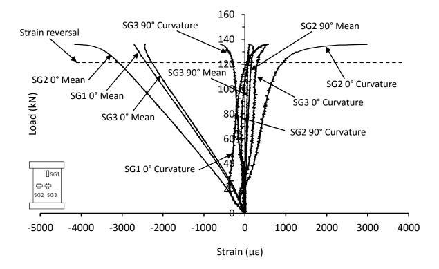
Figure 7.2.18. Mean and curvature strain responses from thick symmetrical CP carbon/epoxy panel with 40mm of core removed (CI-16-16-CP-CR-A)
