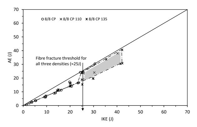
Figure 4.5.5. Absorbed energy vs incident kinetic energy for thin symmetrical CP carbon/epoxy panels with 70, 110 and 135 kg/m<sup>3</sup> core densities
