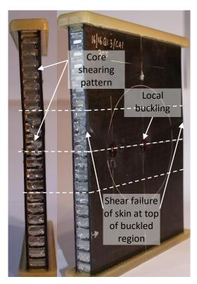
Figure 7.3.3. Photograph of thick symmetrical QI carbon/epoxy panel impacted at 30J after in-plane compression showing left external edge and impacted skin front (CI-16-16-QI-30J-A)
