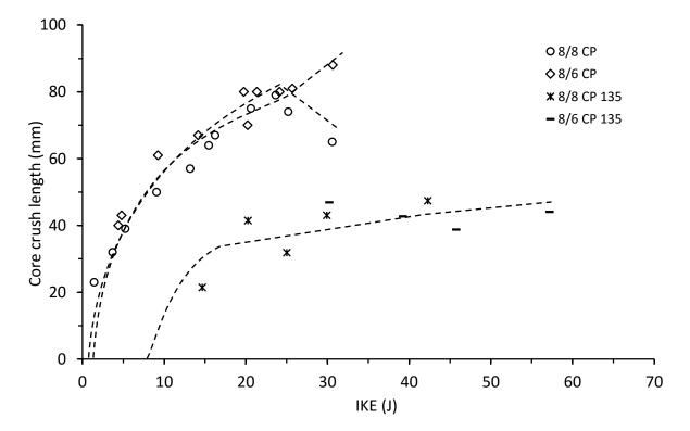
Figure 4.5.2. Core crush length vs incident kinetic energy for thin symmetrical and unsymmetrical CP carbon/epoxy panels with 70 and 135 kg/m<sup>3</sup> core densities
