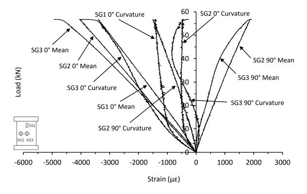
Figure C.24. Mean and curvature strain responses from thin unsymmetrical QI carbon/epoxy panel with 70kg/m<sup>3</sup> core density impacted at 5J (LB-8-6-QI-5J-A)
