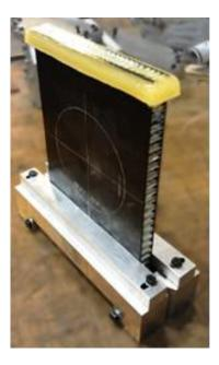
Figure 5.1.3. Photo of a cured end pot at one end, and showing the configuration of the panel while curing the other end
