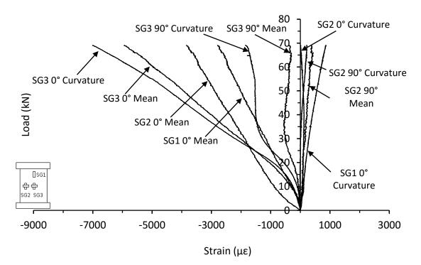
Figure C.2.Mean and curvature strain responses from thin symmetrical CP carbon/epoxy panel with 70kg/m<sup>3</sup> core density impacted at 10J (HD-8-8-CP-10J)
