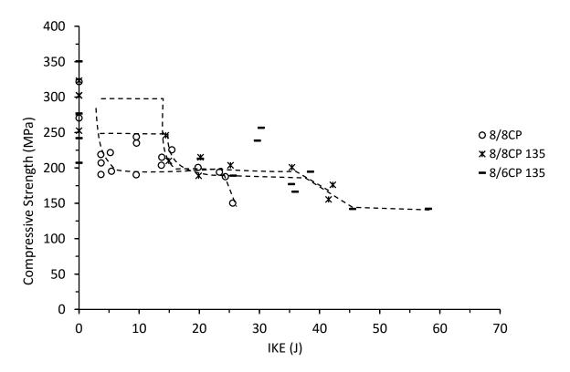
Figure 7.6.2. Compressive strength vs incident kinetic energy for thin symmetrical and unsymmetrical CP carbon/epoxy panels with 70 and 135kg/m<sup>3</sup> core density
