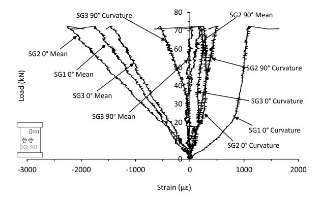
Figure C.41. Mean and curvature strain responses from thick unsymmetrical CP carbon/epoxy panel with 70kg/m<sup>3</sup> core density impacted at 30J (DJ-16-12-CP-30J-A)
