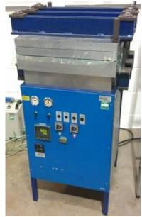
Figure 2.2.8. (a) Autoclave with lid off showing bagging film and breather layers (b) autoclave with steel cross members held in place by bolts
