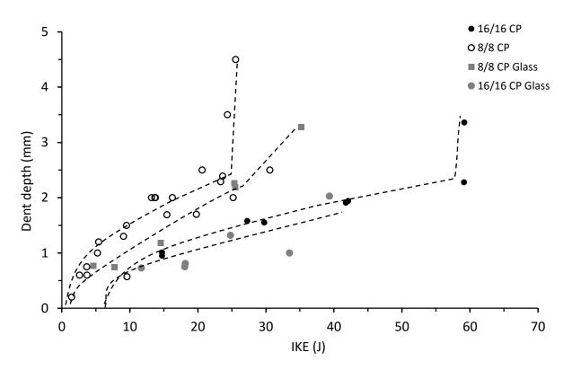
Figure 4.5.11. Dent depth vs incident kinetic energy for thin and thick symmetrical CP carbon and Eglass/epoxy panels with 70 kg/m<sup>3</sup> core density
