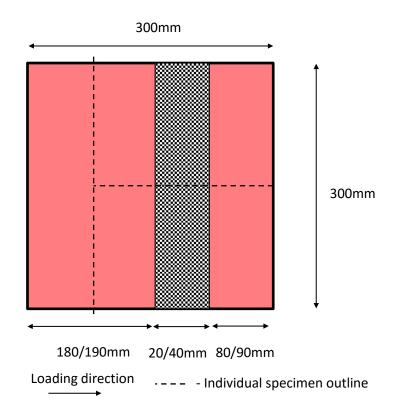
Figure 2.4.1. Adhesive placement on 300 x 300mm skin for in-plane compression core removal specimens
