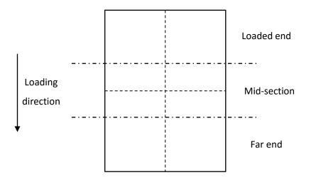
Figure 6.1.1. Diagram showing the three discrete regions of the panel used in identifying the location of the panel failure after in-plane compression
