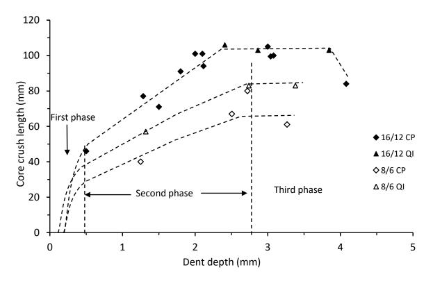
Figure 4.3.12. Core crush length vs dent depth for thin and thick unsymmetrical CP and QI carbon/epoxy panels with 70 kg/m<sup>3</sup> core density
