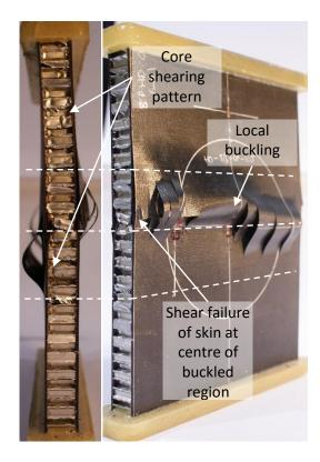
Figure 7.3.2. Photograph of thin unsymmetrical CP carbon/epoxy panel impacted at 10J after in-plane compression showing left external edge and impacted skin front (HD-8-6-CP-10J)
