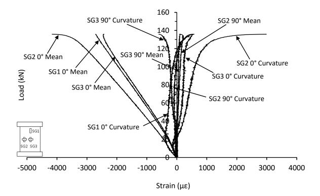
Figure D.7. Mean and curvature strain responses from thick symmetrical CP carbon/epoxy panel with 70kg/m<sup>3</sup> core density with 40mm of core removed (CI-16-16-CP-CR-1)
