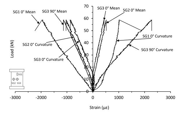
Figure C.73. Mean and curvature strain responses from thin unsymmetrical CP carbon/epoxy panel with 135kg/m<sup>3</sup> core density impacted at 30J (MB-8-6-CP-30J)
