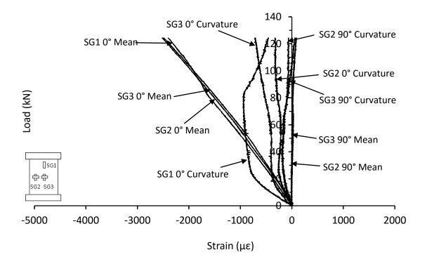
Figure 6.2.2. Mean and curvature strain response for a thick symmetrical CP carbon/epoxy control panel with 70kg/m<sup>3</sup> core density (CI-16-16-CP-0J-A)
