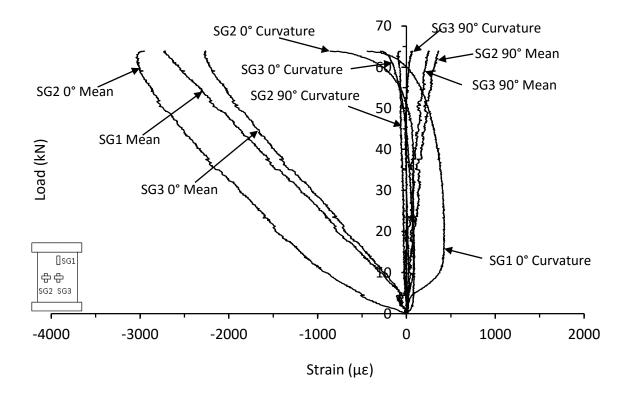
Figure D.12. Mean and curvature strain responses from thin symmetrical CP carbon/epoxy panel with 70kg/m<sup>3</sup> core density with 20mm of core removed (HD-8-8-CP-CR-B)
