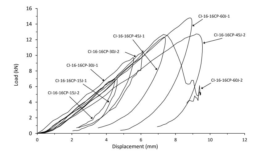
Figure B3. All impact testing load displacement responses from thick symmetrical CP carbon/epoxy panels with 70kg/m<sup>3</sup> core density
