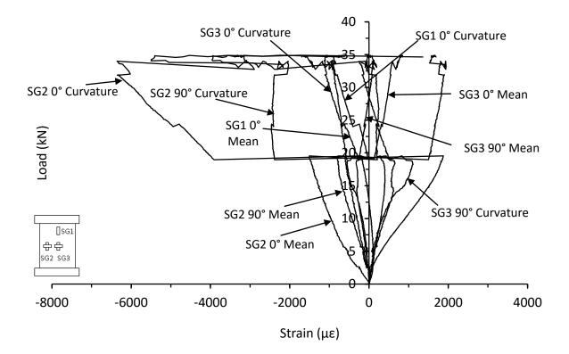
Figure C.61. Mean and curvature strain responses from thin unsymmetrical CP carbon/epoxy panel with 110kg/m<sup>3</sup> core density impacted at 40J (AR-8-6-CP-40J)
