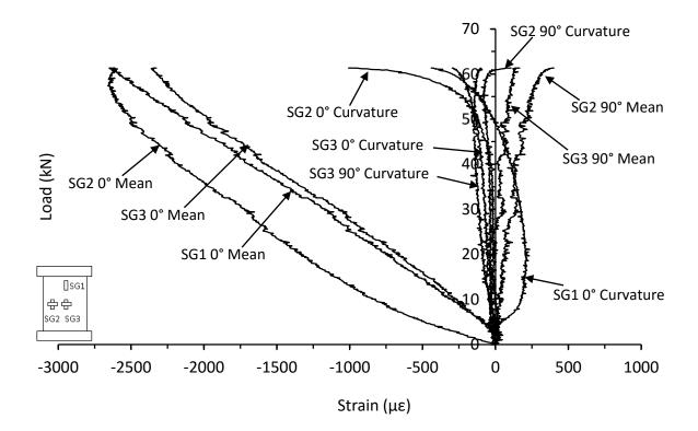
Figure D.11. Mean and curvature strain responses from thin symmetrical CP carbon/epoxy panel with 70kg/m<sup>3</sup> core density with 20mm of core removed (HD-8-8-CP-CR-A)
