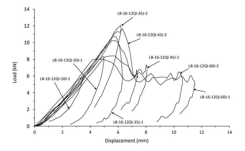
Figure B7. All impact testing load displacement responses from thick unsymmetrical QI carbon/epoxy panels with 70kg/m<sup>3</sup> core density
