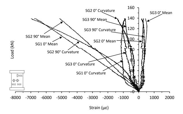
Figure C.83. Mean and curvature strain responses from thick symmetrical CP E-glass/epoxy panel with 70kg/m<sup>3</sup> core density impacted at 12J (SG-16-16-CP-12J)
