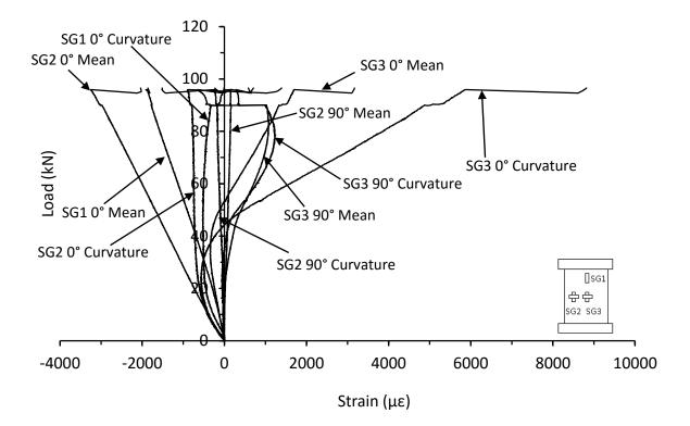
Figure C.43. Mean and curvature strain responses from thick unsymmetrical CP carbon/epoxy panel with 70kg/m<sup>3</sup> core density impacted at 45J (NC-16-12-CP-45J)
