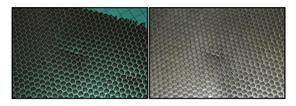
Figure 2.1.8. Examples of core defects in honeycomb material from handling, storage or manufacturing
