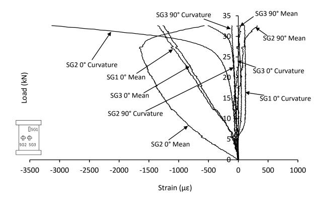
Figure 7.2.24. Mean and curvature strain responses from thin unsymmetrical CP carbon/epoxy panel with 20mm of core removed (HD-8-6-CP-CR-A)
