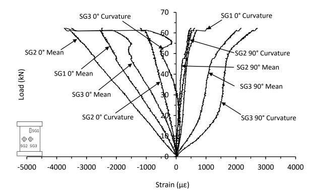
Figure C.17. Mean and curvature strain responses from thin unsymmetrical CP carbon/epoxy panel with 70kg/m<sup>3</sup> core density impacted at 30J (DJ-8-6-CP-30J-A)
