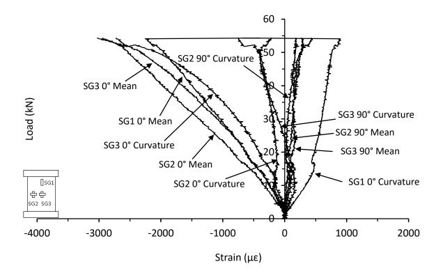
Figure C.15. Mean and curvature strain responses from thin unsymmetrical CP carbon/epoxy panel with 70kg/m<sup>3</sup> core density impacted at 25J (DJ-8-6-CP-25J-A)
