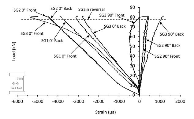
Figure 7.2.3. Strain responses from thin unsymmetrical CP carbon/epoxy panel with 70kg/m<sup>3</sup> core density impacted at 10J (HD-8-6-CP-10J)
