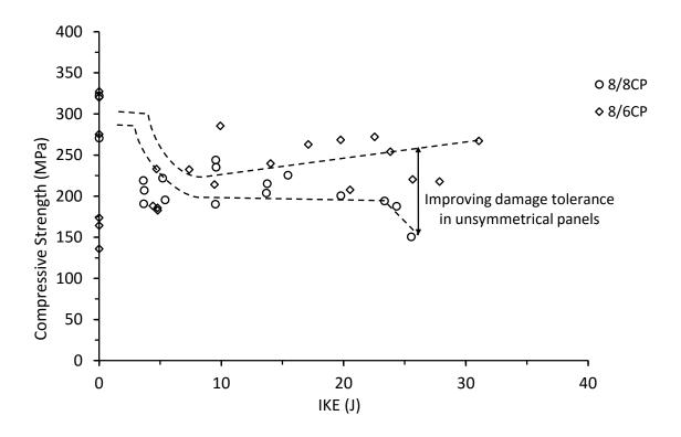
Figure 7.5.1. Compressive strength vs incident kinetic energy for thin symmetrical and unsymmetrical CP and QI carbon/epoxy panels with 70kg/m<sup>3</sup> core density
