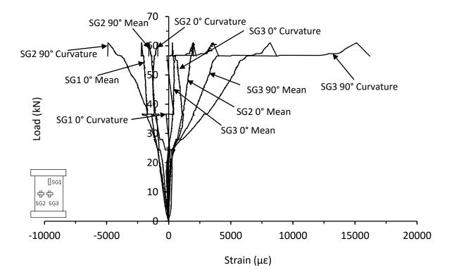
Figure C.63. Mean and curvature strain responses from thin symmetrical CP carbon/epoxy panel with 135kg/m<sup>3</sup> core density impacted at 15J (MB-8-8-CP-15J)
