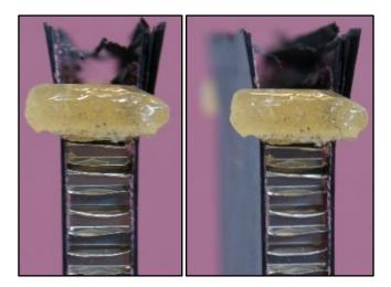
Figure 6.1.3. Observed end crushing mechanism failure in thin symmetrical CP carbon/epoxy panels with 110kg/m<sup>3</sup> core (AR-8-8-CP-0J-B)
