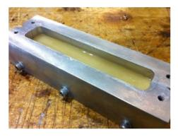
Figure 5.1.1. Photo of end potting mould with epoxy resin inside
