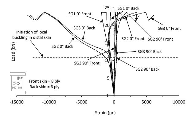
Figure 7.2.14. Strain responses from thin unsymmetrical QI carbon/epoxy panel with 40mm of core removed (LB-8-6-QI-CR-A)
