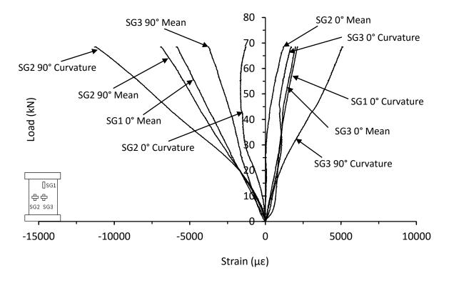
Figure C.80. Mean and curvature strain responses from thin symmetrical CP E-glass/epoxy panel with 70kg/m<sup>3</sup> core density impacted at 15J (SG-8-8-CP-15J)
