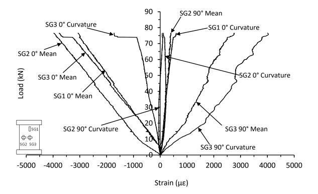
Figure C.53. Mean and curvature strain responses from thin symmetrical CP carbon/epoxy panel with 110kg/m<sup>3</sup> core density impacted at 10J (AR-8-8-CP-10J)
