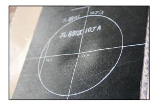
Figure 4.1.4. Impact damage in a thin symmetrical QI carbon/epoxy panel with 70kg/m<sup>3</sup> core impacted at 10J showing an example of surface indentation (JL-8-8-QI-10J-A)
