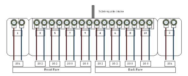
Figure 5.3.2. Assignment of strain gauges and wires to data logger channels
