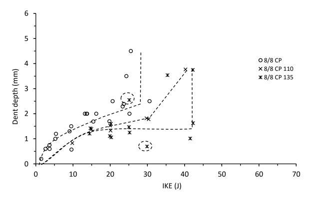
Figure 4.5.3. Dent depth vs incident kinetic energy for thin symmetrical CP carbon/epoxy panels with 70, 110 and 135 kg/m<sup>3</sup> core densities
