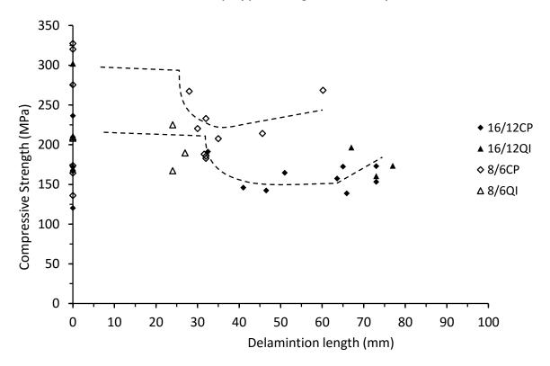
Figure 7.4.6. Compressive strength vs delamination length for thick and thin unsymmetrical CP and QI carbon/epoxy panels 70kg/m<sup>3</sup> core density
