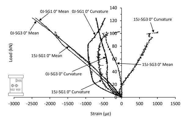
Figure 7.2.10. Mean and curvature strain responses from thick symmetrical CP carbon/epoxy control and 15J impacted panel (CI-16-16-CP-0J-A and CI-16-16-CP-15J-A)
