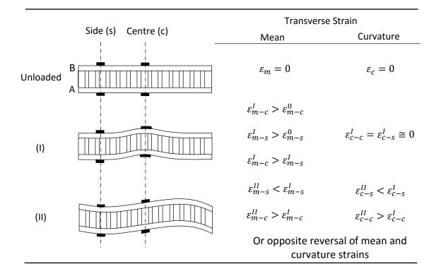
Figure 7.10.2. Illustration of the expected buckling deformation process of undamaged control panels under in-plane compression in the transverse direction
