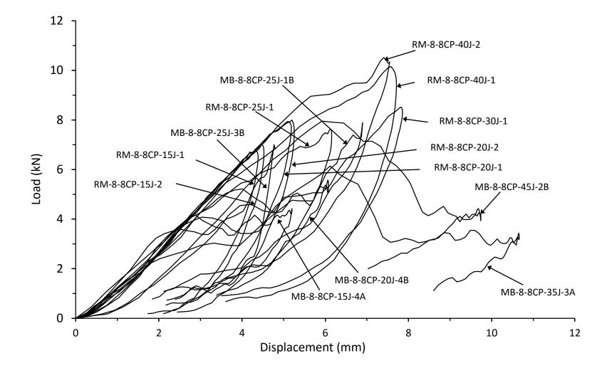
Figure B10. All impact testing load displacement responses from thin symmetrical CP carbon/epoxy panels with 135kg/m<sup>3</sup> core density
