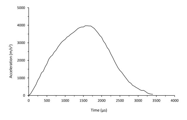
Figure 3.3.3. Acceleration time response for a thin unsymmetrical CP carbon/epoxy panel with 70kg/m<sup>3</sup> core density impacted at 20J (HD-8-6-CP-20J)
