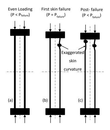
Figure 6.2.3. A deformation sequence of end region at-the-side view based on measured strain responses (a) unloaded state (b) initial compressive failure of front skin (c) transfer of load to un-failed skin
