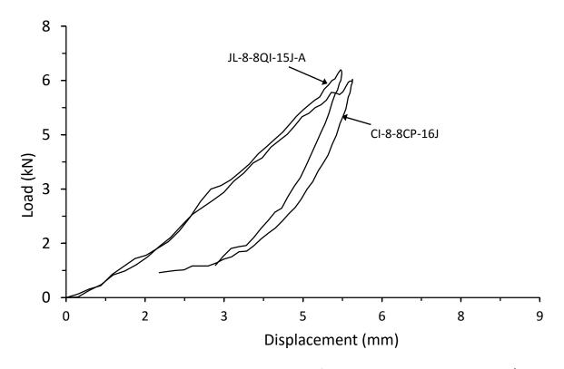
Figure 4.2.21. Load vs displacement response comparison for thin symmetrical CP and QI carbon/epoxy panels with 70kg/m<sup>3</sup> core density impacted at 16J and 15J respectively
