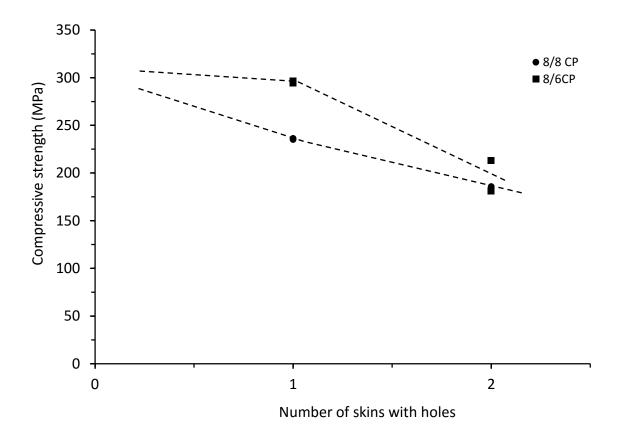
Figure 7.9.1. Compressive strengths of thin symmetrical and unsymmetrical CP carbon/epoxy panels with 40mm hole drilled in skins
