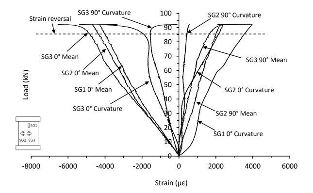
Figure 7.2.2. Mean and curvature strain responses from thin symmetrical QI carbon/epoxy panel with 70kg/m<sup>3</sup> core density impacted at 25J (JL-8-8-QI-25J-B)
