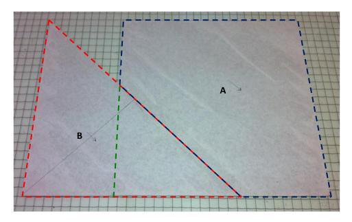
Figure 2.2.3. Alignment of pieces A and B creating 45° ply joined temporarily with tape
