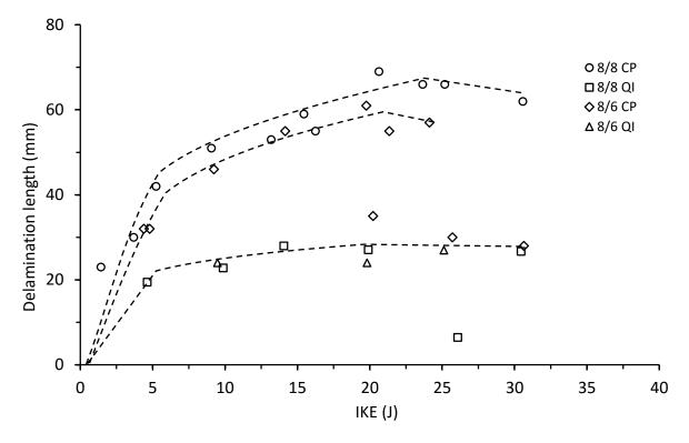
Figure 4.4.2. Delamination length vs incident kinetic energy for thin symmetrical and unsymmetrical CP and QI carbon/epoxy panels with 70 kg/m<sup>3</sup> core density
