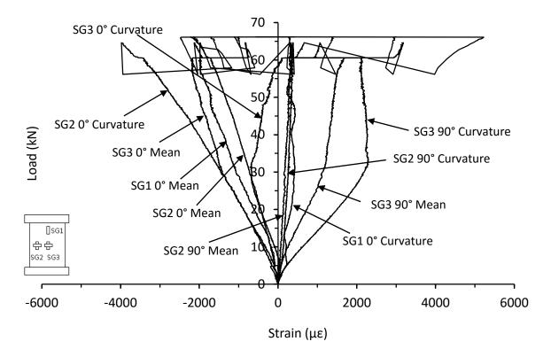
Figure C.72. Mean and curvature strain responses from thin unsymmetrical CP carbon/epoxy panel with 135kg/m<sup>3</sup> core density impacted at 30J (RM-8-6-CP-30J-A)
