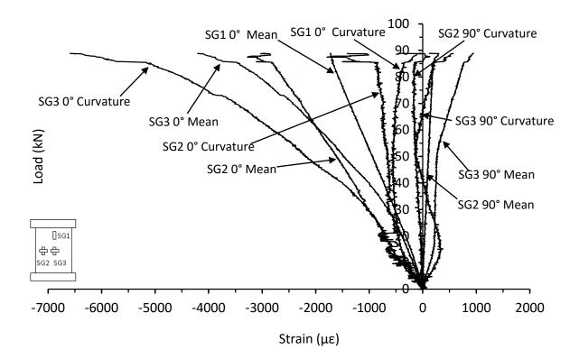
Figure C.39. Mean and curvature strain responses from thick unsymmetrical CP carbon/epoxy panel with 70kg/m<sup>3</sup> core density impacted at 20J (NC-16-12-CP-20J)
