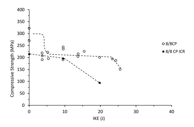
Figure 7.8.3. Compressive strength against IKE for thin symmetrical CP carbon/epoxy panels with and without 20mm of core removed
