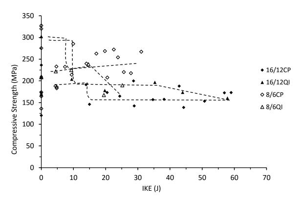
Figure 7.4.2. Compressive strength vs incident kinetic energy for thick and thin unsymmetrical CP and QI carbon/epoxy panels 70kg/m<sup>3</sup> core density
