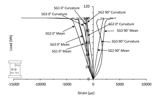
Figure C.49. Mean and curvature strain responses from thick unsymmetrical QI carbon/epoxy panel with 70kg/m<sup>3</sup> core density impacted at 35J (LB-16-12-QI-35J-B)
