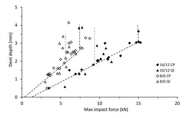
Figure 4.3.10. Dent depth vs maximum impact force for thin and thick unsymmetrical CP and QI carbon/epoxy panels with 70 kg/m<sup>3</sup> core density
