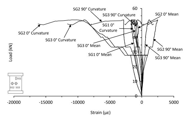
Figure C.56. Mean and curvature strain responses from thin symmetrical CP carbon/epoxy panel with 110kg/m<sup>3</sup> core density impacted at 30J (AR-8-8-CP-30J)
