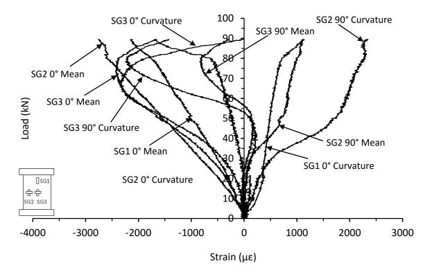
Figure C.46. Mean and curvature strain responses from thick unsymmetrical CP carbon/epoxy panel with 70kg/m<sup>3</sup> core density impacted at 60J (DJ-16-12-CP-60J-A)
