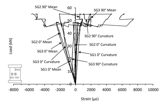
Figure C.64. Mean and curvature strain responses from thin symmetrical CP carbon/epoxy panel with 135kg/m<sup>3</sup> core density impacted at 20J (RM-8-8-CP-20J-A)
