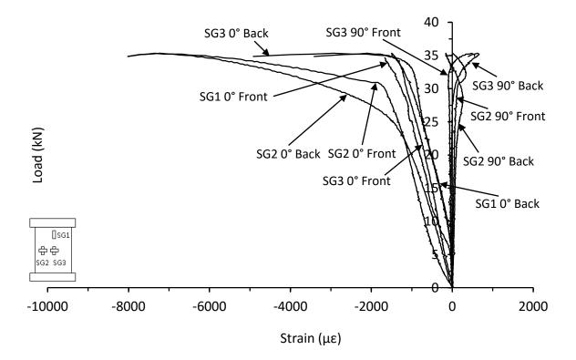
Figure 7.2.11. Strain responses from thin symmetrical CP carbon/epoxy panel with 40mm of core removed (CI-8-8-CP-CR-A)
