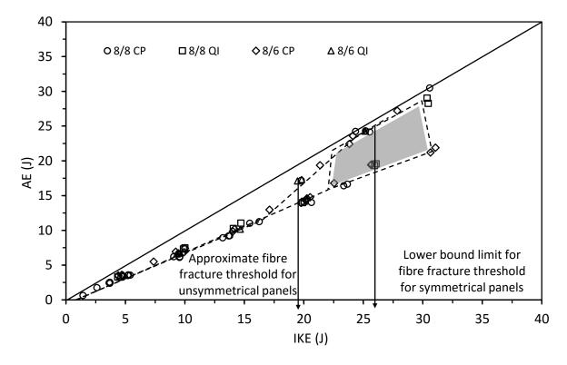
Figure 4.4.8. Absorbed energy vs incident kinetic energy for thin symmetrical and unsymmetrical CP and QI carbon/epoxy panels with 70 kg/m<sup>3</sup> core density
