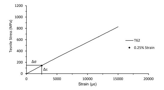
Figure 2.1.1. Tensile stress/strain response from 6 ply multi-directional laminate showing chord point used in modulus calculation, specimen T62
