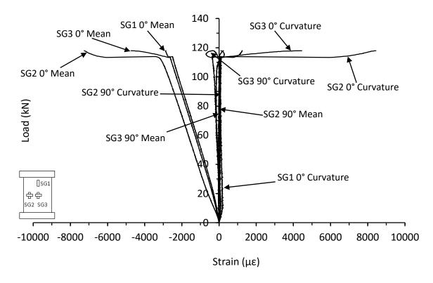
Figure D.10. Mean and curvature strain responses from thick unsymmetrical CP carbon/epoxy panel with 70kg/m<sup>3</sup> core density with 40mm of core removed (NC-16-12-CP-CR-B)
