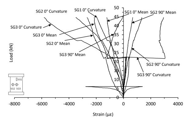
Figure C.60. Mean and curvature strain responses from thin unsymmetrical CP carbon/epoxy panel with 110kg/m<sup>3</sup> core density impacted at 30J (AR-8-6-CP-30J)
