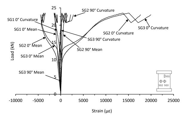
Figure D.6. Mean and curvature strain responses from thin unsymmetrical QI carbon/epoxy panel with 70kg/m<sup>3</sup> core density with 40mm of core removed (LB-8-6-QI-CR-B)
