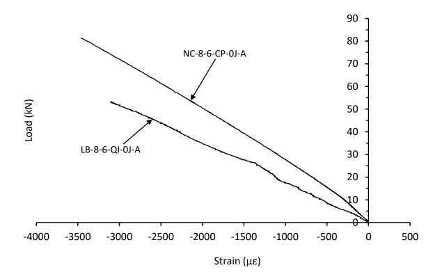
Figure 6.3.10. Mean strain response from the far-field region for thin unsymmetrical CP and QI carbon/epoxy control panels with 70kg/m<sup>3</sup> core density
