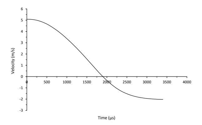
Figure 3.3.4. Velocity time response for a thin unsymmetrical CP carbon/epoxy panel with 70kg/m<sup>3</sup> core density impacted at 20J (HD-8-6-CP-20J)
