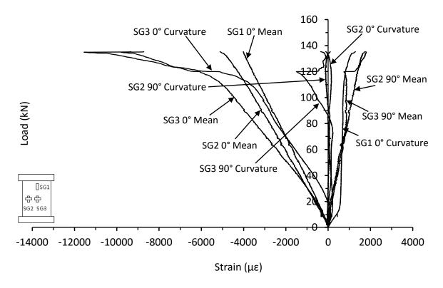
Figure C.32. Mean and curvature strain responses from thick symmetrical QI carbon/epoxy panel with 70kg/m<sup>3</sup> core density impacted at 15J (JL-16-16-QI-15J-B)
