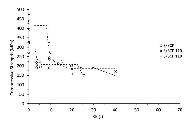
Figure 7.6.1. Compressive strength vs incident kinetic energy for thin symmetrical and unsymmetrical CP carbon/epoxy panels with 70 and 110kg/m<sup>3</sup> core density
