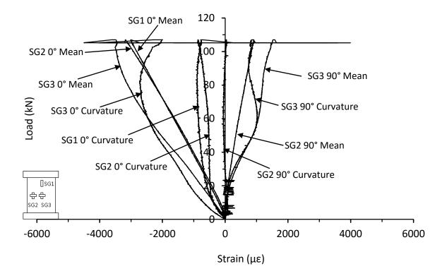
Figure C.33. Mean and curvature strain responses from thick symmetrical QI carbon/epoxy panel with 70kg/m<sup>3</sup> core density impacted at 15J (CI-16-QI-15J)
