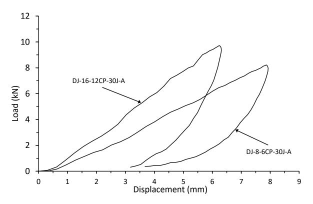
Figure 4.2.23. Load vs displacement response comparison for thick and thin unsymmetrical CP carbon/epoxy panels with 70kg/m<sup>3</sup> core density impacted at 30J
