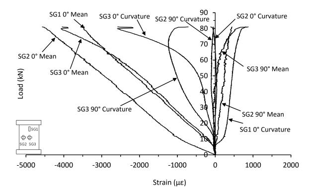
Figure C.9. Mean and curvature strain responses from thin unsymmetrical CP carbon/epoxy panel with 70kg/m<sup>3</sup> core density impacted at 10J (HD-8-6-CP-10J)
