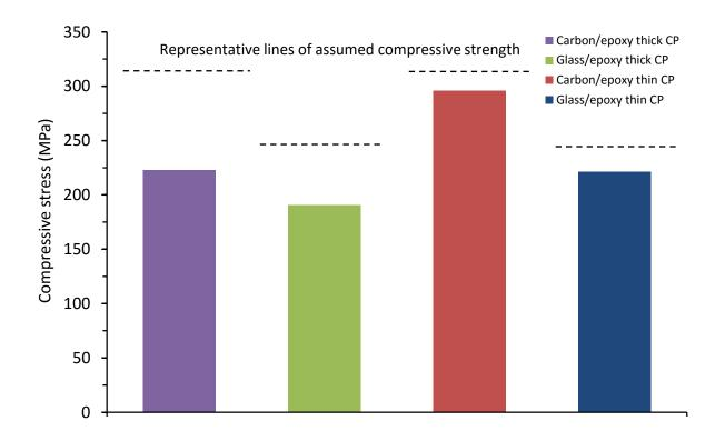
Figure 6.3.13. Average compressive stresses of thin and thick symmetrical CP carbon and E-glass/epoxy panels with 70kg/m<sup>3</sup> core density
