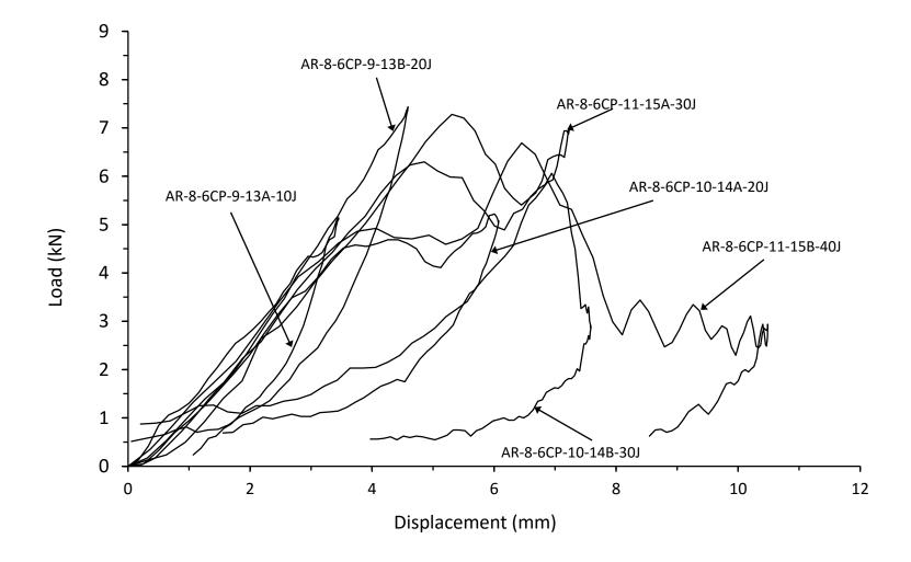
Figure B9. All impact testing load displacement responses from thin unsymmetrical CP carbon/epoxy panels with 110kg/m<sup>3</sup> core density
