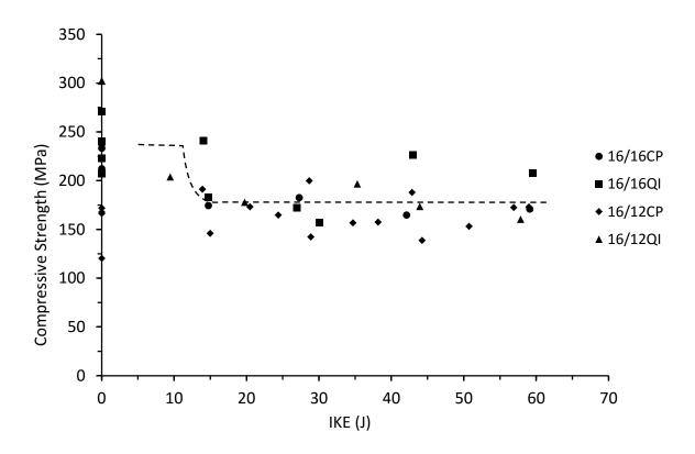
Figure 7.5.3 Compressive strength vs incident kinetic energy for thick symmetrical and unsymmetrical CP and QI carbon/epoxy panels with 70kg/m<sup>3</sup> core density
