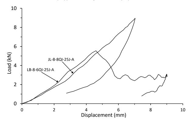
Figure 4.2.20. Load vs displacement response comparison for thin symmetrical and unsymmetrical QI carbon/epoxy panels with 70kg/m<sup>3</sup> core density impacted at 25J
