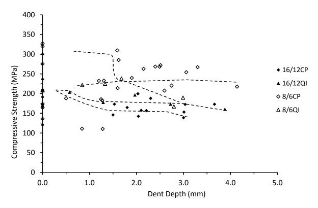
Figure 7.4.4. Compressive strength vs dent depth for thick and thin unsymmetrical CP and QI carbon/epoxy panels 70kg/m<sup>3</sup> core density
