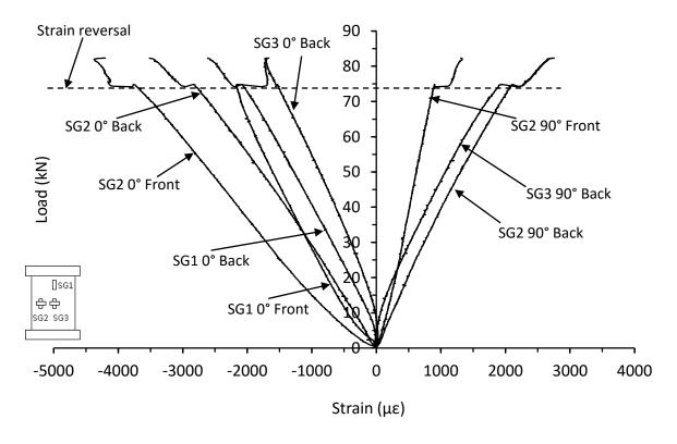
Figure 7.2.7. Strain responses from thick unsymmetrical QI carbon/epoxy panel with 70kg/m<sup>3</sup> core density impacted at 60J (LB-16-12-QI-60J-A)
