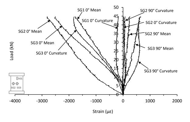
Figure C.58. Mean and curvature strain responses from thin unsymmetrical carbon/epoxy CP panel with 110kg/m<sup>3</sup> core density impacted at 20J (AR-8-6-CP-20J-B)
