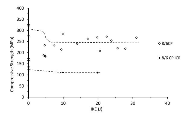
Figure 7.8.4. Compressive strength against IKE for thin unsymmetrical CP carbon/epoxy panels with and without 20mm of core removed
