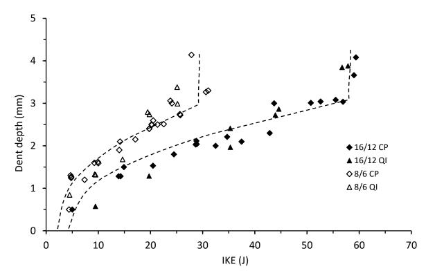
Figure 4.3.6. Dent depth vs incident kinetic energy for thin and thick unsymmetrical CP and QI carbon/epoxy panels with 70 kg/m<sup>3</sup> core density
