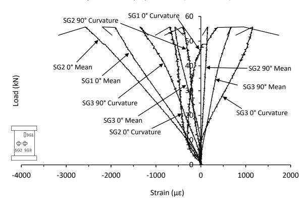
Figure C.16. Mean and curvature strain responses from thin unsymmetrical CP carbon/epoxy panel with 70kg/m<sup>3</sup> core density impacted at 28J (NC-8-6-CP-28J)
