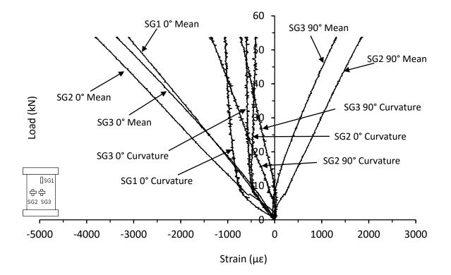
Figure 6.2.6. Mean and curvature strain response for a thin unsymmetrical QI carbon/epoxy control panel with 70kg/m<sup>3</sup> core density (LB-8-6-QI-0J-B)
