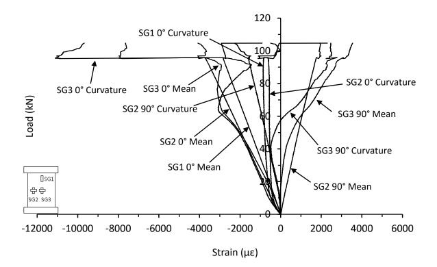
Figure C.47. Mean and curvature strain responses from thick unsymmetrical QI carbon/epoxy panel with 70kg/m<sup>3</sup> core density impacted at 10J (LB-16-12-QI-10J-A)
