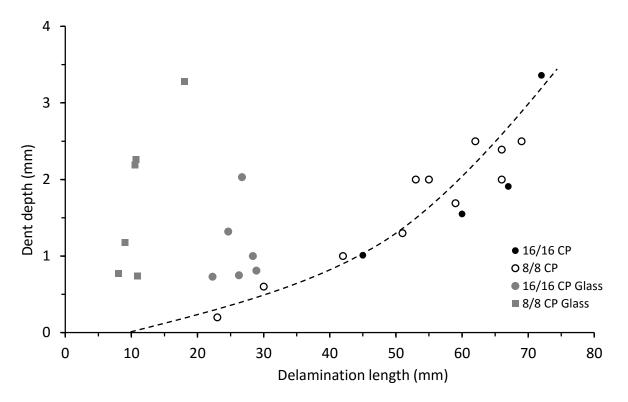
Figure 4.5.14. Dent depth vs delamination length for thin and thick symmetrical CP carbon and Eglass/epoxy panels with 70 kg/m<sup>3</sup> core density
