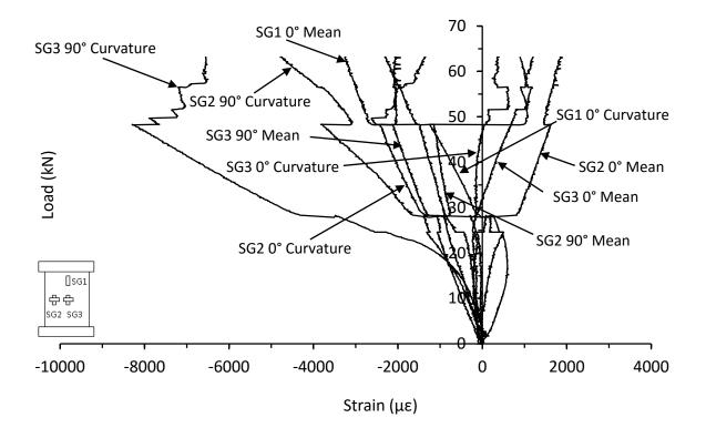
Figure C.65. Mean and curvature strain responses from thin symmetrical CP carbon/epoxy panel with 135kg/m<sup>3</sup> core density impacted at 20J (MB-8-8-CP-20J)
