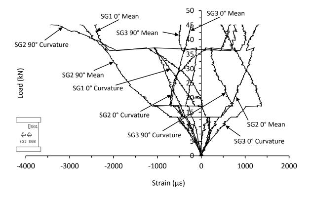
Figure C.74. Mean and curvature strain responses from thin unsymmetrical CP carbon/epoxy panel with 135kg/m<sup>3</sup> core density impacted at 35J (MB-8-6-CP-35J)
