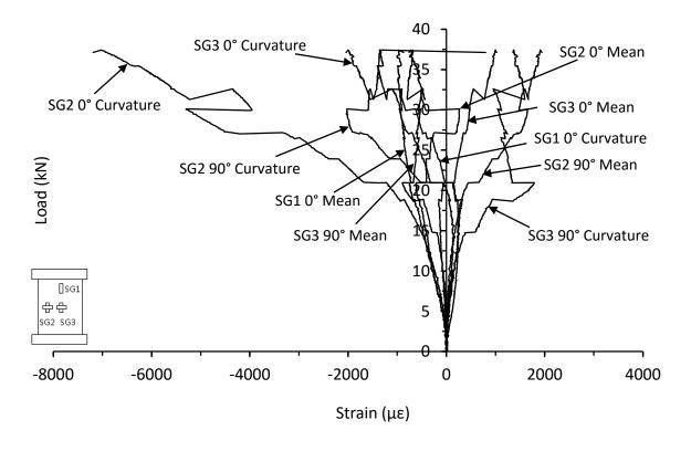
Figure C.78. Mean and curvature strain responses from thin unsymmetrical CP carbon/epoxy panel with 135kg/m<sup>3</sup> core density impacted at 60J (RM-8-6-CP-60J-A)
