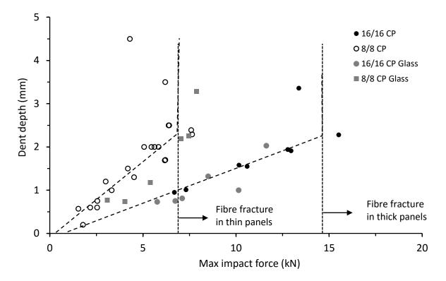
Figure 4.5.13. Dent depth vs max impact force for thin and thick symmetrical CP carbon and E-glass/epoxy panels with 70 kg/m<sup>3</sup> core density
