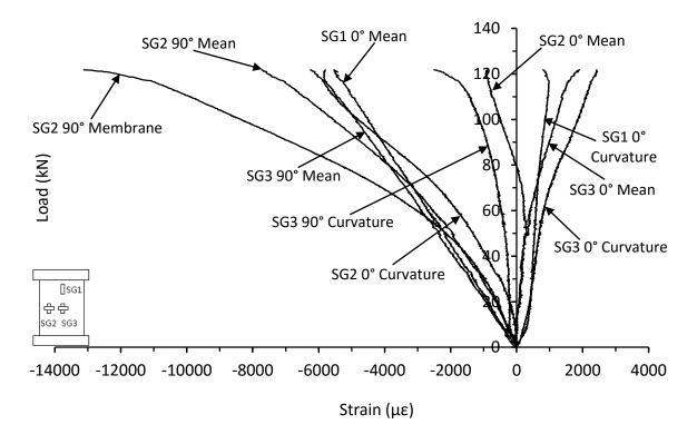
Figure C.86. Mean and curvature strain responses from thick symmetrical CP E-glass/epoxy panel with 70kg/m<sup>3</sup> core density impacted at 35J (SG-16-16-CP-35J)
