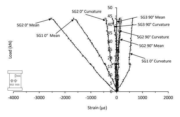
Figure C.6. Mean and curvature strain responses from thin unsymmetrical CP carbon/epoxy panel with 70kg/m<sup>3</sup> core density impacted at 5J (DJ-8-6-CP-5J-B3)
