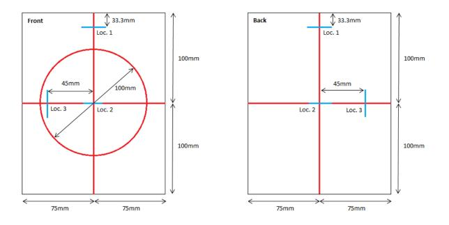
Figure 2.5.2. Surface markings for LVI specimens, and strain gauge locations
