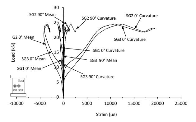
Figure D.3. Mean and curvature strain responses from thin unsymmetrical CP carbon/epoxy panel with 70kg/m<sup>3</sup> core density with 40mm of core removed (NC-8-6-CP-CR-A)
