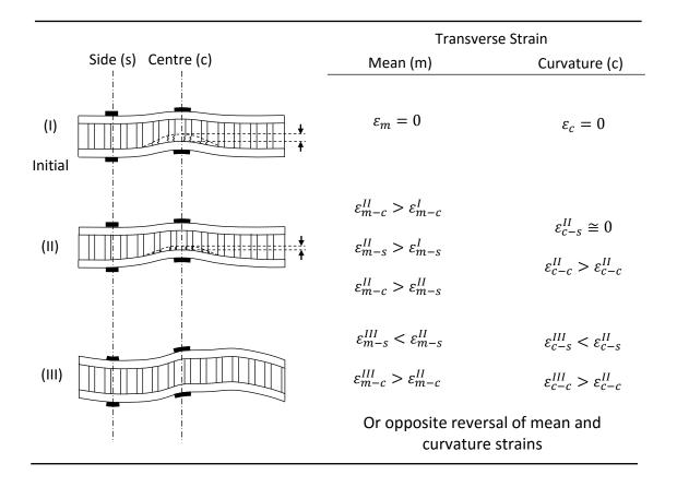
Figure 7.10.5. Illustration of the probable buckling deformation process of impact damaged panels under inplane compression in the transverse loading direction.
