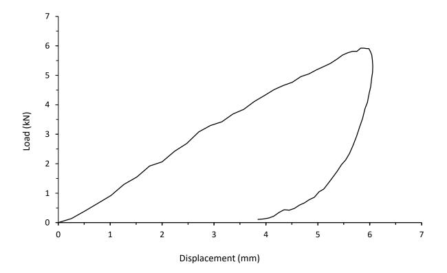
Figure 3.3.6. Load displacement response for a thin unsymmetrical CP carbon/epoxy panel with 70kg/m<sup>3</sup> core density impacted at 20J (HD-8-6-CP-20J)
