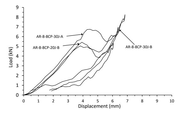
Figure 4.2.17. Load vs displacement response for thin symmetrical CP carbon/epoxy panels with 110kg/m<sup>3</sup> core density impacted at 20J and 30J
