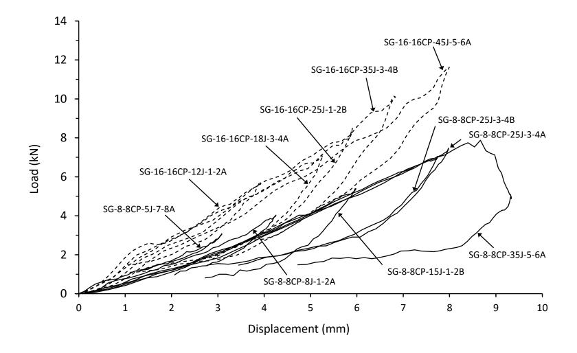
Figure B12. All impact testing load displacement responses from thin and thick symmetrical CP E-glass/epoxy panels with 70kg/m<sup>3</sup> core density
