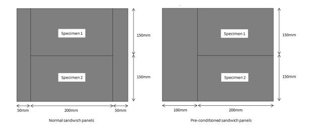
Figure 2.5.1. Cutting measurements applied to panels before cutting
