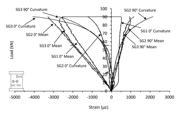
Figure C.34. Mean and curvature strain responses from thick symmetrical QI carbon/epoxy panel with 70kg/m<sup>3</sup> core density impacted at 30J (JL-16-16-QI-30J-B)
