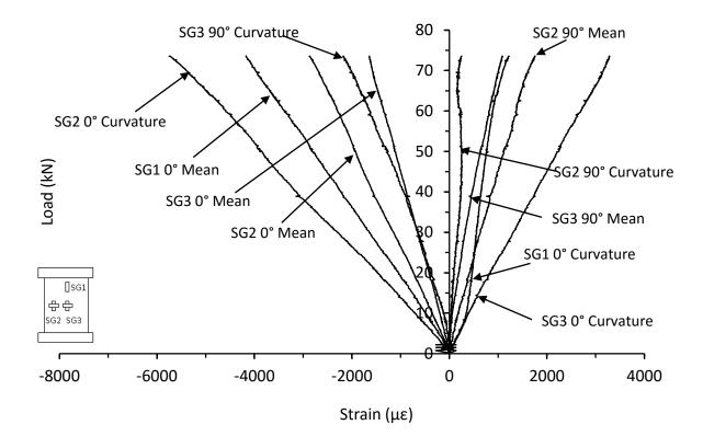
Figure C.23. Mean and curvature strain responses from thin symmetrical QI carbon/epoxy panel with 70kg/m<sup>3</sup> core density impacted at 30J (JL-8-8-QI-30J-B)
