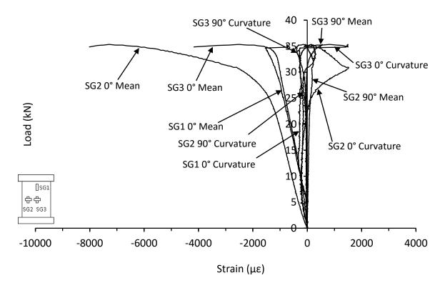
Figure 7.2.12. Mean and curvature strain responses from thin symmetrical CP carbon/epoxy panel with 40mm of core removed (CI-8-8-CP-CR-A)
