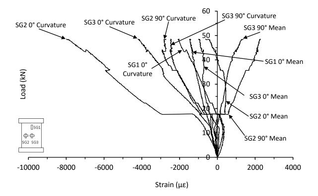
Figure C.71. Mean and curvature strain responses from thin unsymmetrical CP carbon/epoxy panel with 135kg/m<sup>3</sup> core density impacted at 25J (MB-8-6-CP-25J)
