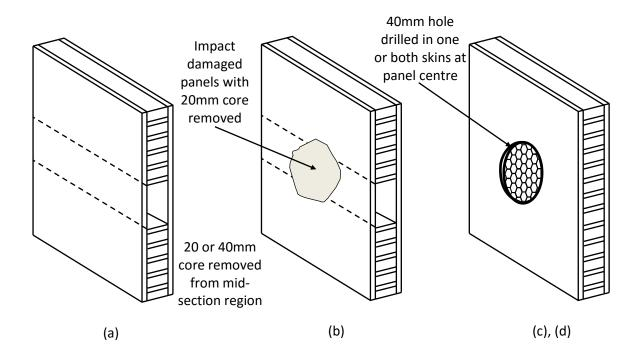
Figure 7.1.1. Sketches showing pre-conditions in panels (a) removed core at the mid-section region, (b) impacted removed core at the mid-section region, (c) drilled hole in a one skin and (d) drilled holes in both skins
