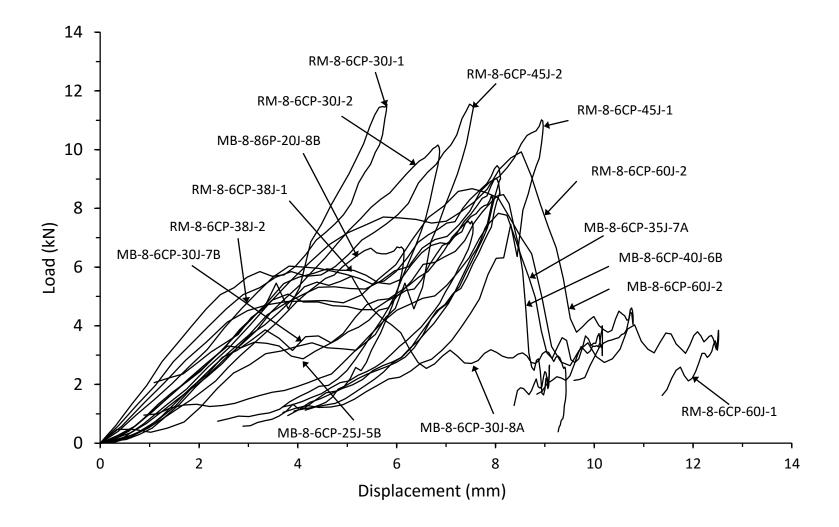
Figure B11. All impact testing load displacement responses from thin unsymmetrical CP carbon/epoxy panels with 135kg/m<sup>3</sup> core density
