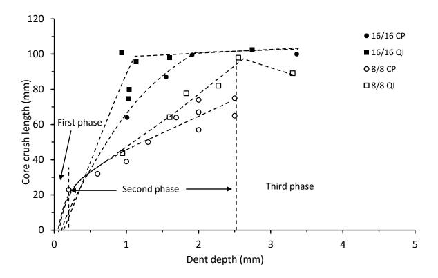
Figure 4.3.11. Core crush length vs dent depth for thin and thick symmetrical CP and QI carbon/epoxy panels with 70 kg/m<sup>3</sup> core density
