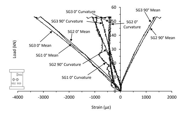
Figure 6.2.5. Mean and curvature strain response for a thin unsymmetrical QI carbon/epoxy control panel with 70kg/m<sup>3</sup> core density (LB-8-6-QI-0J-A)
