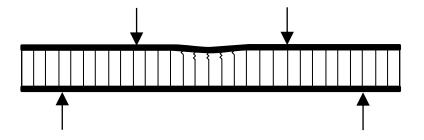
Figure 1.3.1. Four point bending flexure testing on impact damaged beams
