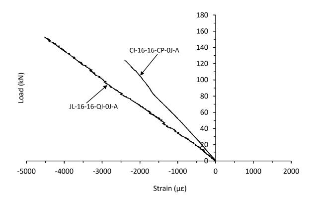
Figure 6.3.9. Mean strain response from the far-field region for thick symmetrical CP and QI carbon/epoxy control panels with 70kg/m<sup>3</sup> core density
