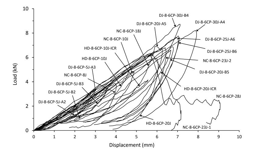
Figure B2. All impact testing load displacement responses from thin unsymmetrical CP carbon/epoxy panels with 70kg/m<sup>3</sup> core density
