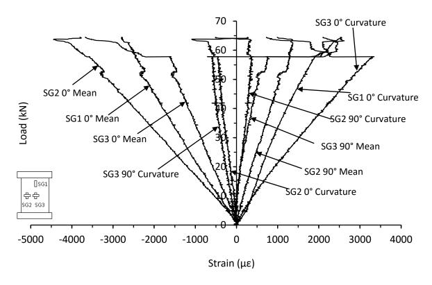
Figure C.18. Mean and curvature strain responses from thin symmetrical QI carbon/epoxy panel with 70kg/m<sup>3</sup> core density impacted at 5J (JL-8-8-QI-5J-B)
