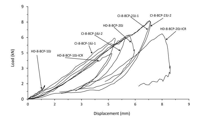
Figure B1. All impact testing load displacement responses from thin symmetrical CP carbon/epoxy panels with 70kg/m<sup>3</sup> core density
