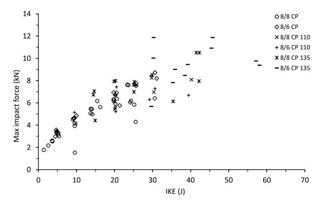
Figure 4.5.7. Maximum impact force vs incident kinetic energy for thin symmetrical and unsymmetrical CP carbon/epoxy panels with 70, 110, and 135kg/m<sup>3</sup> core densities
