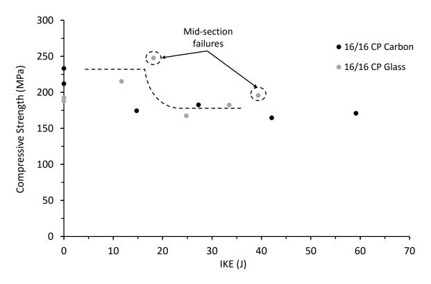
Figure 7.7.3. Compressive strength vs incident kinetic energy for thick symmetrical CP carbon and Eglass/epoxy panels with 70kg/m<sup>3</sup> core density
