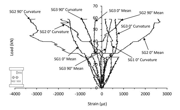
Figure C.67. Mean and curvature strain responses from thin symmetrical CP carbon/epoxy panel with 135kg/m<sup>3</sup> core density impacted at 35J (MB-8-8-CP-35J)
