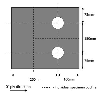
Figure 2.4.2. Hole locations on 300 x 300mm skin before bonding to core
