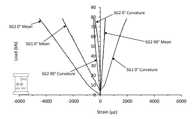
Figure D.23. Mean and curvature strain responses from thin unsymmetrical CP carbon/epoxy panel with 70kg/m<sup>3</sup> core density with 40mm hole drilled in the top skin (HD-8-6-CP-1H-A)
