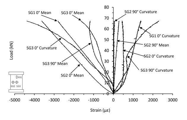
Figure C.10. Mean and curvature strain responses from thin unsymmetrical CP carbon/epoxy panel with 70kg/m<sup>3</sup> core density impacted at 18J (NC-8-6-CP-18J)
