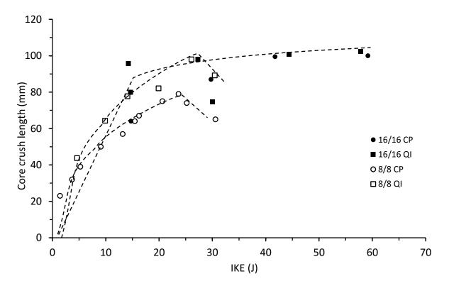
Figure 4.3.3 Core crush length vs incident kinetic energy for thin and thick symmetrical CP and QI carbon/epoxy panels with 70 kg/m<sup>3</sup> core density
