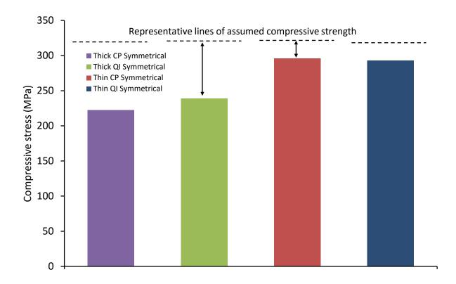
Figure 6.3.1. Average compressive stresses of thick and thin symmetrical CP and QI carbon/epoxy control panels with 70kg/m<sup>3</sup> density
