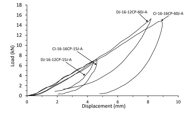
Figure 4.2.14. Load vs displacement response for thick symmetrical and unsymmetrical CP carbon/epoxy panels with 70kg/m<sup>3</sup> core density impacted at 15J and 60J
