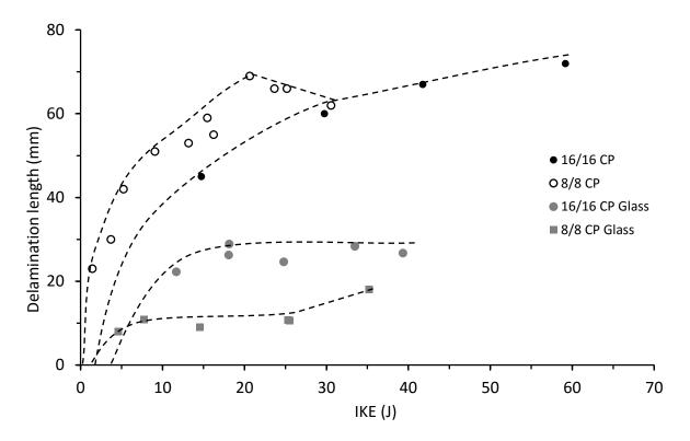
Figure 4.5.9. Delamination length vs incident kinetic energy for thin and thick symmetrical CP carbon and Eglass/epoxy panels with 70 kg/m<sup>3</sup> core density
