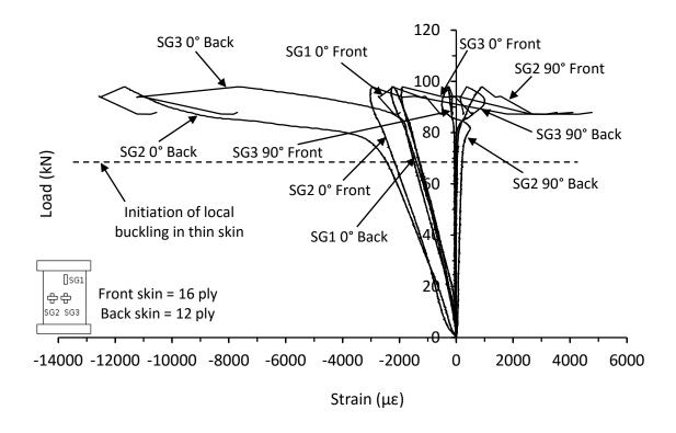
Figure 7.2.19. Strain responses from thick unsymmetrical CP carbon/epoxy panel with 40mm of core removed (NC-16-12-CP-CR-A)
