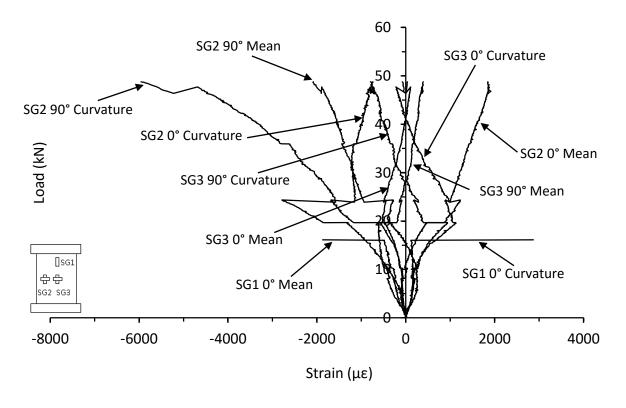
Figure C.76. Mean and curvature strain responses from thin unsymmetrical CP carbon/epoxy panel with 135kg/m<sup>3</sup> core density impacted at 40J (MB-8-6-CP-40J)
