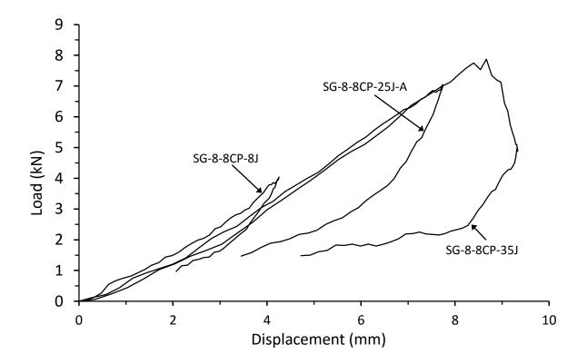
Figure 4.2.15. Load vs displacement response for thin symmetrical CP E-glass/epoxy panels with 70kg/m<sup>3</sup> impacted at 8J, 25J, and 35J
