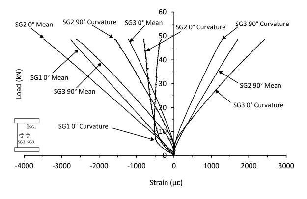
Figure C.28. Mean and curvature strain responses from thin unsymmetrical QI carbon/epoxy panel with 70kg/m<sup>3</sup> core density impacted at 25J (LB-8-6-QI-25J-A)
