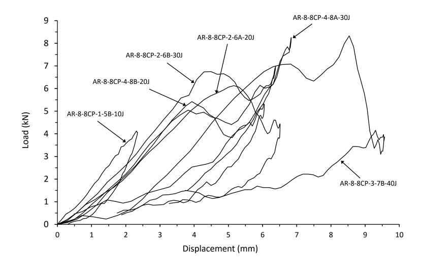
Figure B8. All impact testing load displacement responses from thin symmetrical CP carbon/epoxy panels with 110kg/m<sup>3</sup> core density
