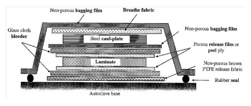
Figure 2.2.7. Diagrammatic representation of order of consumable materials used in autoclave cure process [124]
