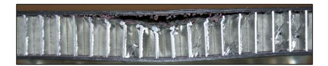
Figure 4.2.12. Cross section of thin symmetrical CP carbon/epoxy panel with 135 kg/m<sup>3</sup> core density impacted at 40J
