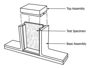
Figure 1.3.3. Schematic of compressive residual strength support fixture with specimen in place for monolithic laminates as detailed by ASTM D7137/D7317M-12.
