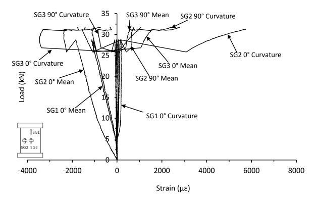
Figure D.14. Mean and curvature strain responses from thin unsymmetrical CP carbon/epoxy panel with 70kg/m<sup>3</sup> core density with 20mm of core removed (HD-8-6-CP-CR-B)
