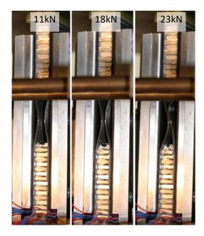
Figure 7.2.13. Progression of local skin buckling in mid-section in thin symmetrical CP carbon/epoxy panel with 40mm core removed (CI-8-8-CP-CR-A)
