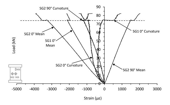
Figure 7.2.8. Mean and curvature strain responses from thick unsymmetrical QI carbon/epoxy panel with 70kg/m<sup>3</sup> core density impacted at 60J (LB-16-12-QI-60J-A)
