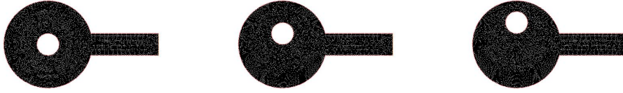
Figure 5.19: An example of some internal domains from waveguides with a single end; varying the vertical position of the obstacle.
