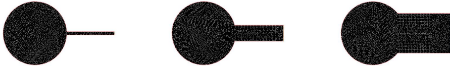
Figure 5.7: An example of some internal domains from waveguides with a single end: varying widths.
