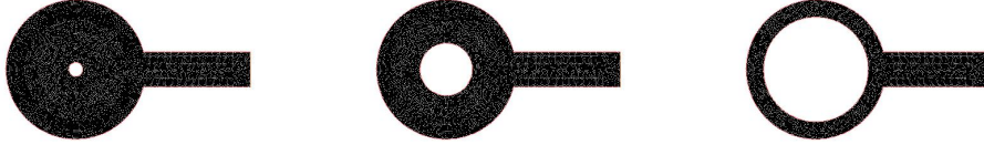
Figure 5.13: An example of some internal domains from waveguides with a single end; varying the obstacle radius.
