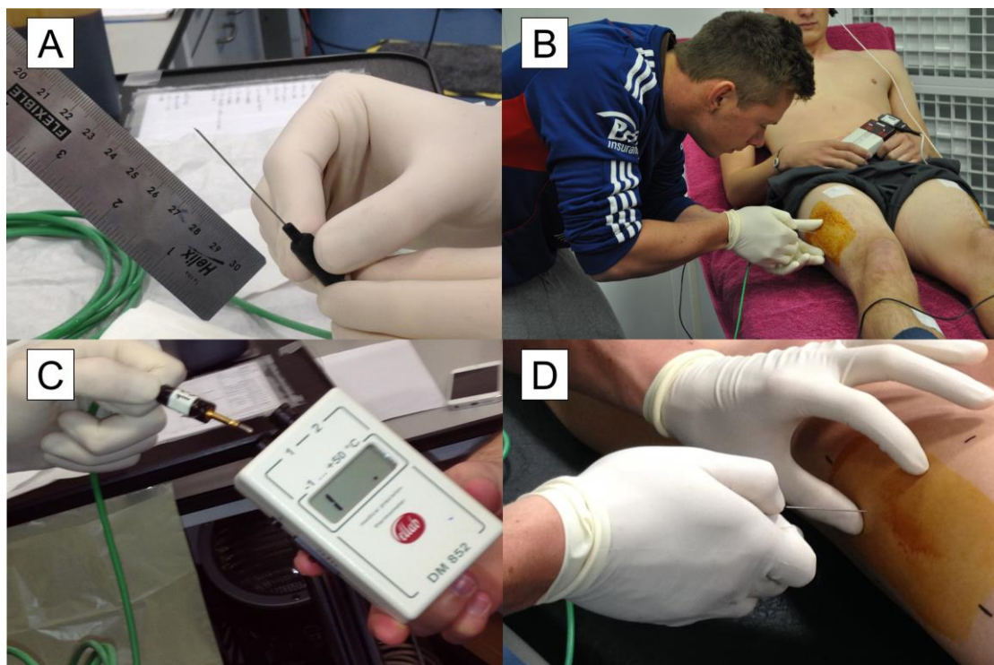
Figure 2-7: Sterile insertion of a solid needle thermocouple for the assessment of muscle temperature as described by Faulkner et al. (2013a). Panel A shows the solid needle thermocouple. Panels B and D show the insertion of the needle into vastus lateralis. Panel C shows the thermometer used to display muscle temperature.
