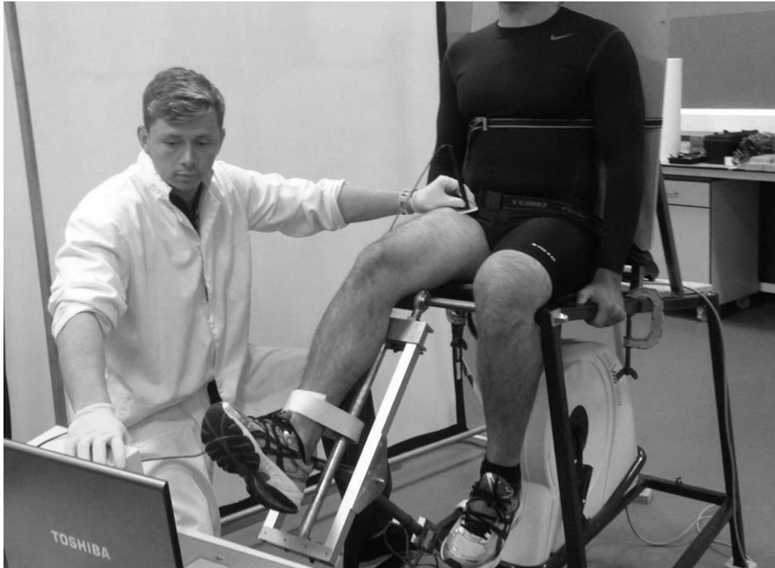
Figure 2-2: Initial prototype used to quantify one-legged isometric maximal voluntary contraction as well as induce dynamic submaximal knee extension fatigue.
