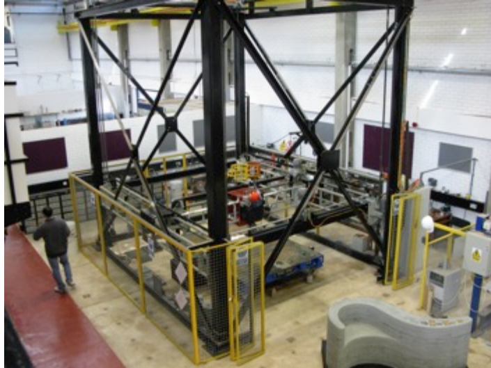
Figure 3: Three-axis gantry printing system of 3D Concrete Printing at Loughborough University – 5m (W) x 5m (L) x 6m (H).
