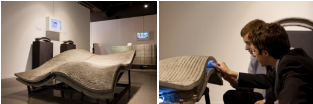
Figure 6: Printed doubly-curved 4-part sandwich panel (1.5m x 1.5m x 0.1m). The panel was exhibited at the Building Centre Exhibition, 25 th August – 8 th September 2011 in London. (Photos: courtesy of Agnese Sanvito)
