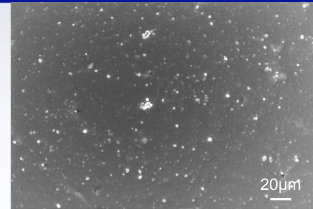
SEM image showing whisker growth on ALD coated sample after 6 months
