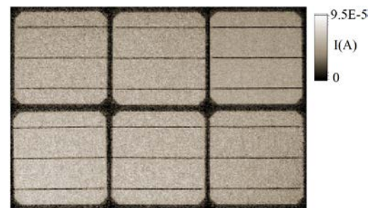
Figure 5: CS current map of the 6 cell PV module used in these experiments. The SC current map is produced having acquired 50% of measurements.
