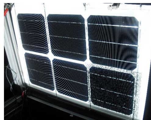
Figure 2: The 6-cell mini module used for these experiments. Patterns are projected on one of the cells (bottom right cell) while the rest are light biased.
