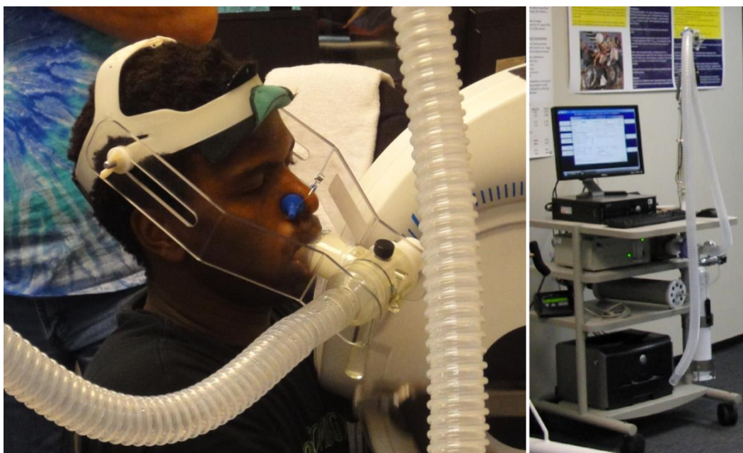
Figure 3.4 Assessment of \dot{V}O_2 using the Parvomedics TrueOne 2400 metabolic cart for breath-by-breath analysis of spirometric data
