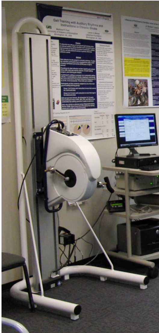
Figure 3.3 Electromagnetically-braked arm-ergometer mounted to a fixed stand with motorised height adjustment
