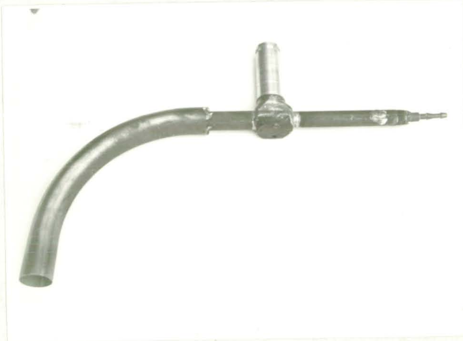
FIGURE 13: Venturi Device for Separation of Fibre
