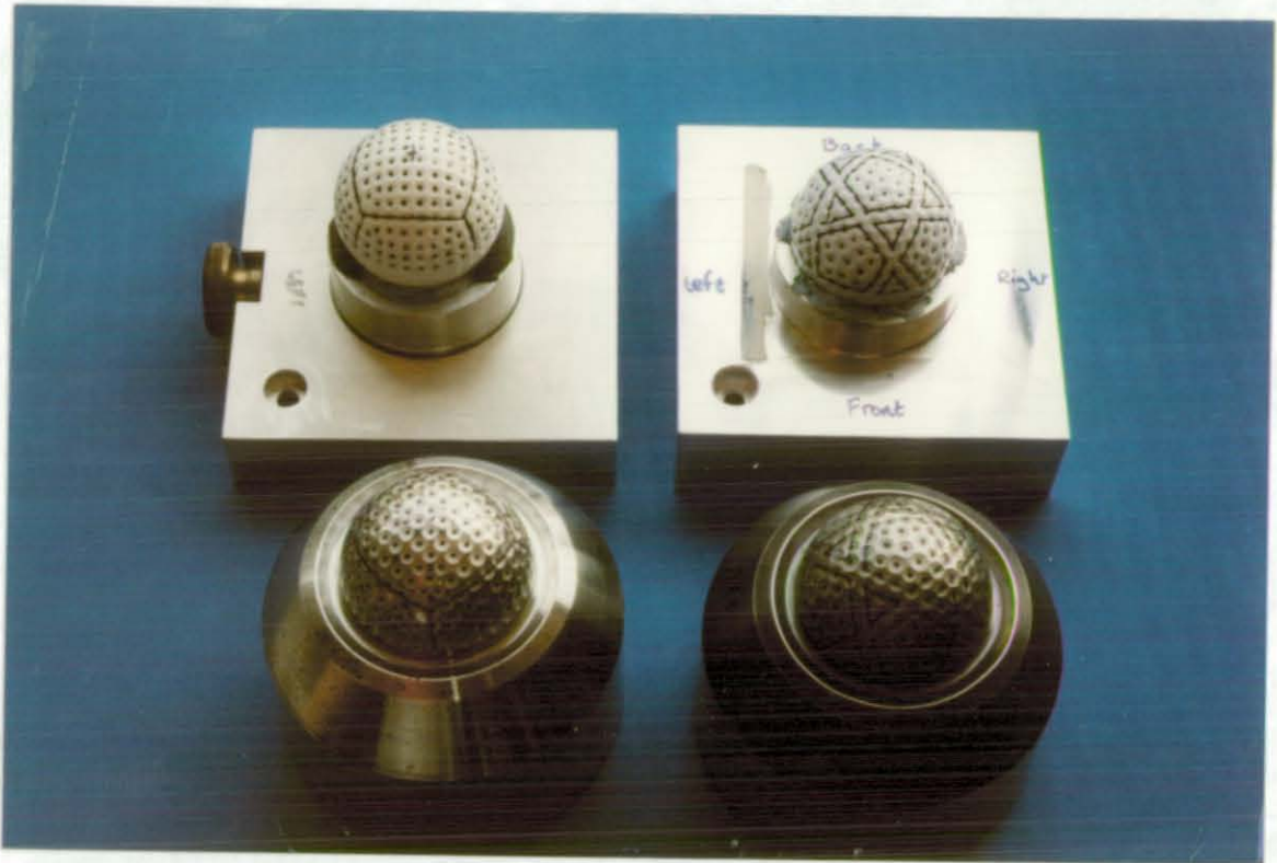
Fig. 4.14. Golf ball hobs and the ball holders.
