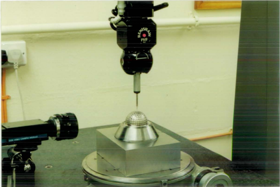
Fig. 5.1(b). The camera positioning on the CMM, for the side viewing.
