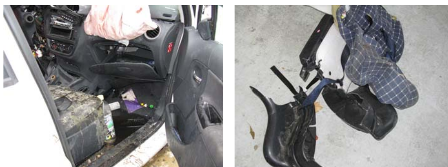
Figure 59: Views of seating position and general state of CRS after the accident
