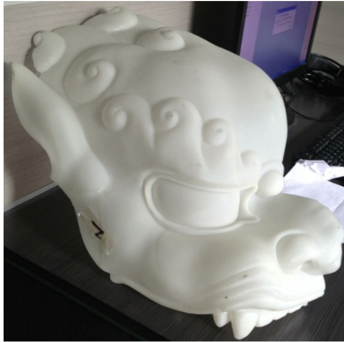
Fig. 9: AM part for a lion's face
