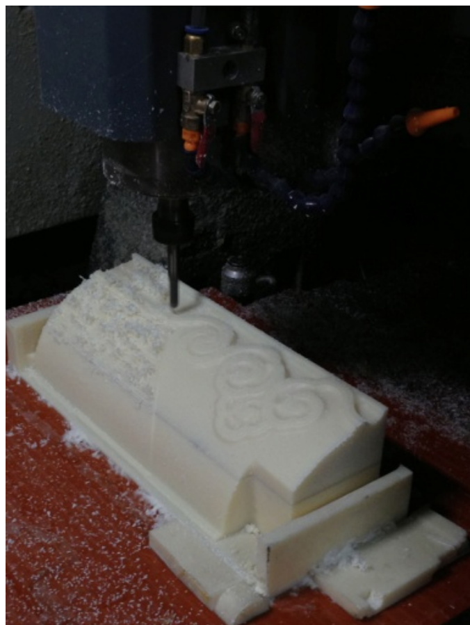
Fig. 10: CNC machining of foam model
