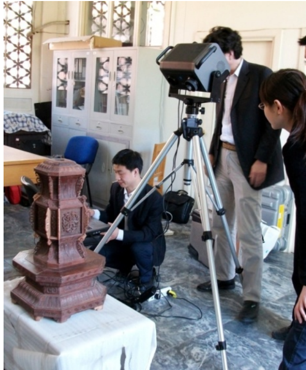
Fig. 3: Non-contact 3D Scanning
