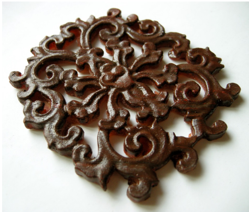
Fig. 4: Finished AM replica of the wooden relief
