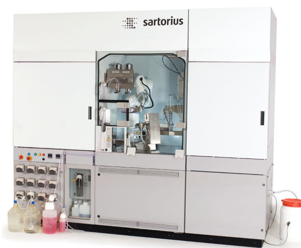
Fig. 2 TAP Biosystems' Compact Select automated cell culture platform (TAP Biosystems, Part of the Sartorius Stedim Biotech Group, Royston, UK)
