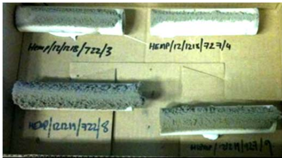
Figure 1: Hemp and coal ash deposits onto ceramic probes
