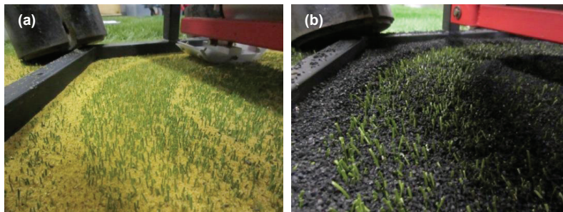
Fig. 2. Surfaces (a) D and (b) E after testing show significant decrease in infill depths along the path of the test foot.
