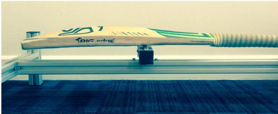
Figure 3.20: Centre of mass measurement of a cricket bat in the vertical plane.
