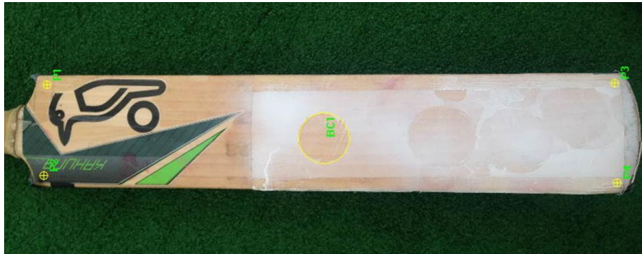
Figure 6.3: Impact location measurement using developer spray.
