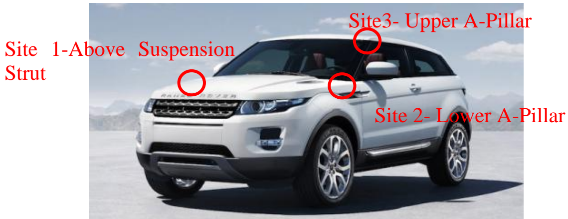
Figure 1: The three measurement response points can be seen, as these are the points at which the accelerometer will be placed. A more detailed imaged of the positioning of the accelerometer at site 1 can be seen in Fig. 2a, which is obscured by the bonnet in Fig. 1.
