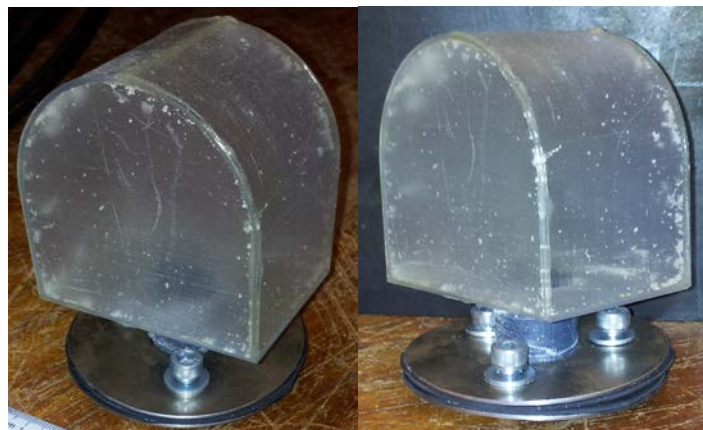
Figure 8 - 3D printed Helmholtz resonators with attachment panels.
