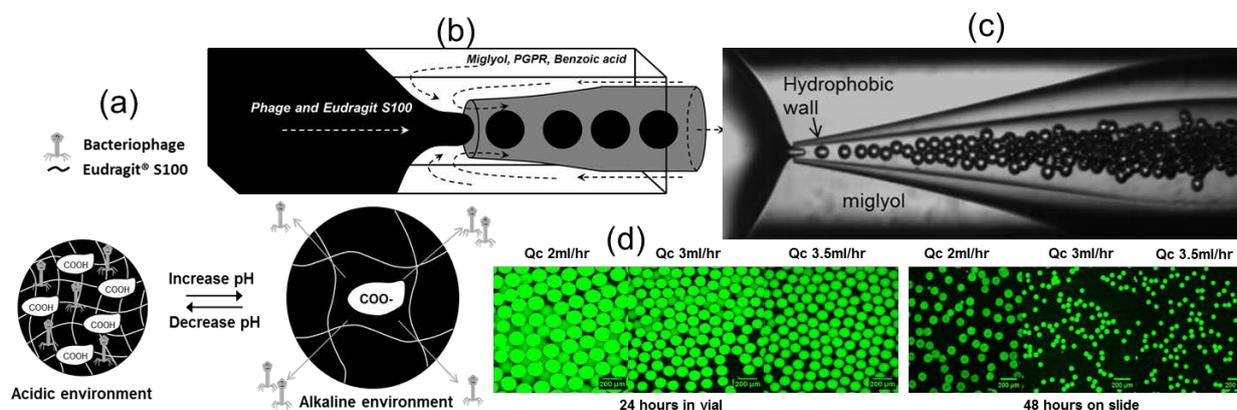
**Figure 1.** a) Schematic to show the polymer release mechanism; b) schematic of the glass capillary microfluidic device for particle generation; c) screen shot of droplet formation; d) SEM of phage encapsulated particles.
