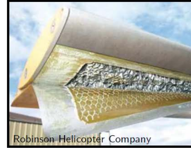
Helicopter blade delamination ▲
