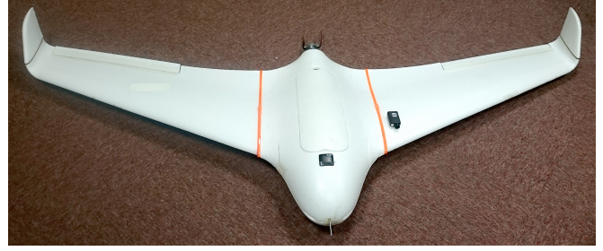
Fig. 2: The Skywalker X8 used in the modelling process. Wingspan: 2.12m, Weight 2.95kg.
