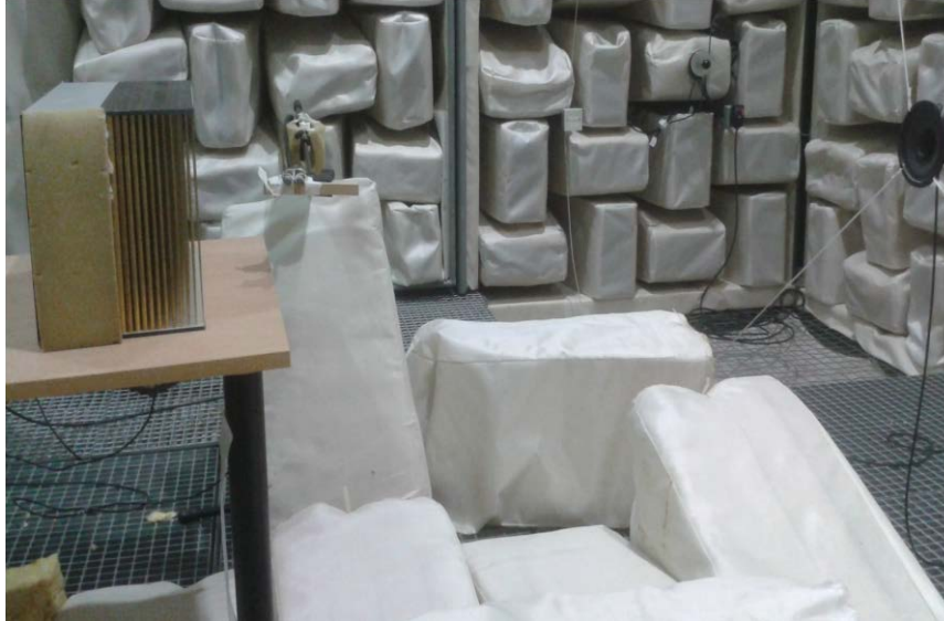
Figure 3: Photograph of the experimental set up showing the QFAA (left) and the loudspeaker (right).
