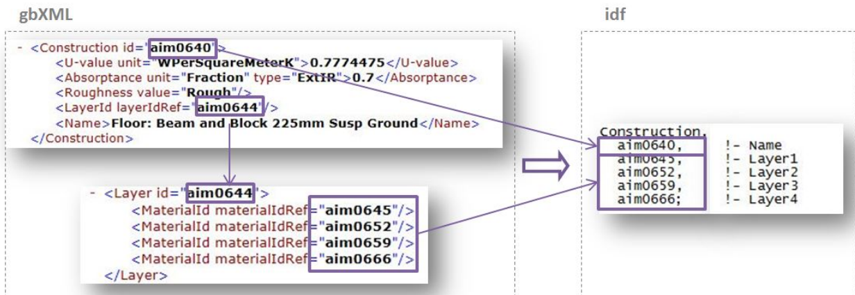
Figure 7 gbXML nodes to idf object mapping example for the 'Construction' idf object
