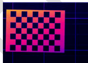
Figure 1: Image (1/20) used for camera calibration based on OpenCV
