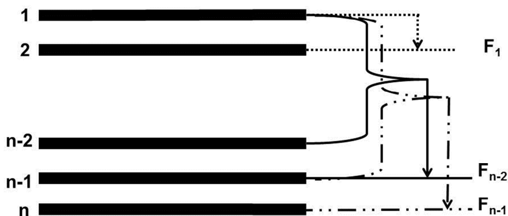
Figure 2: Schematic representation of forces applied on individual fibre layers in a fibrous network.
