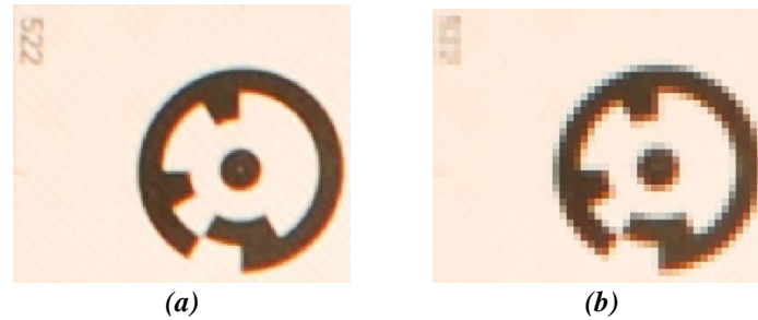
Figure 8. Effect of reducing image resolution. (a) High resolution image with chromatic aberration and spectral mixing on several pixels around the target. (b) Scaled image with reduced number of pixels influenced by chromatic aberration and other optical errors.
